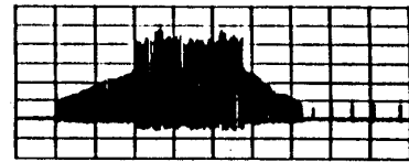
(a) Charging, storing and discharging process 10A/div, 5ms/div
