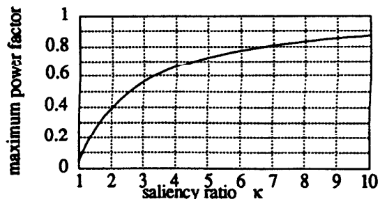
Fig. 3 Power factor vs. saliency ratio \kappa (=L_{ds}/L_{qs}) of a synchronous reluctance motor when the motor is controlled with the maximum power factor control scheme.
