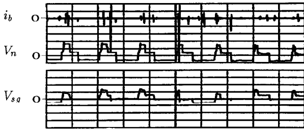
Fig. 16. Insulated-Real case with PWM inverter; bearing current i_b [0.1 A/div] expanded scale, neutral voltage V_n [200 V/div], shaft voltage V_{sg} [20 V/div], t = 100\mu\text{s}/\text{div}
