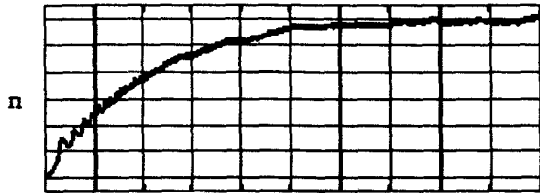
Fig. 5: Starting process with partial load. Speed from 0 to 300 rpm versus time from 0 to 10 sec.
