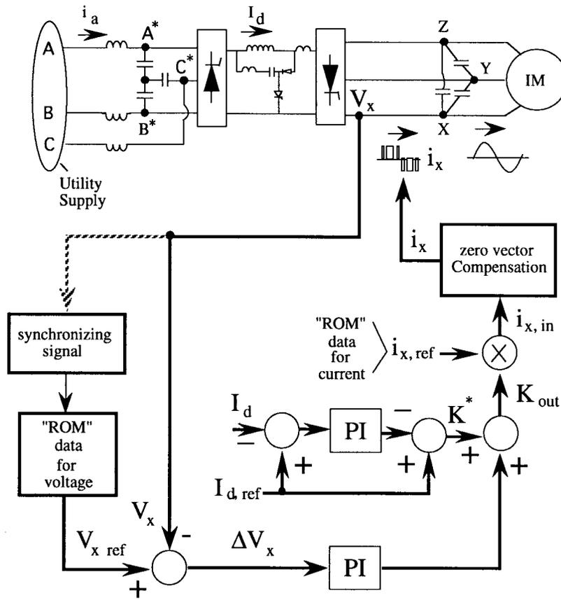
Fig. 10. V/F control by PWM current pulses.
