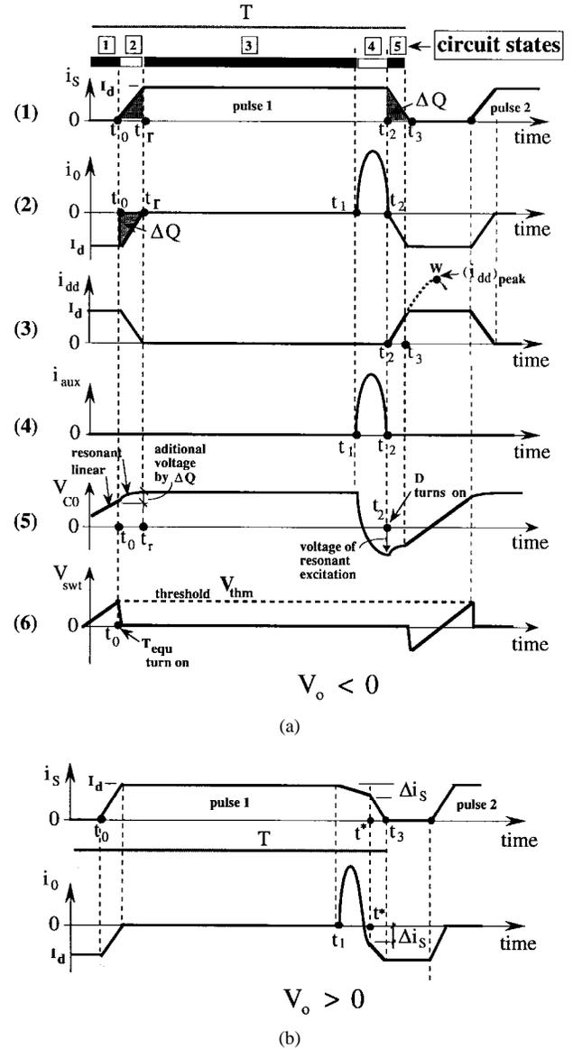
Fig. 3. (a) Current waveforms for  $V_o < 0$  and (b) current waveforms for  $V_o > 0$ .
