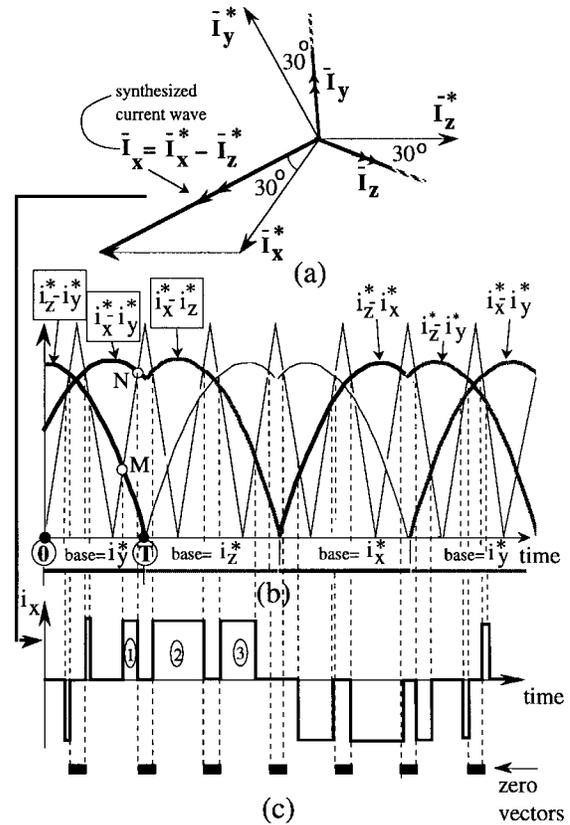
Fig. 9. PWM method and zero vectors.
