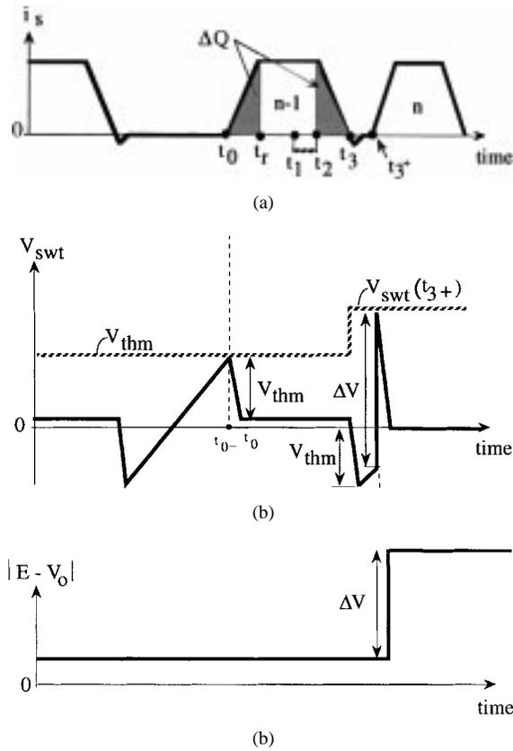
Fig. 6. (a) Consecutive current pulses “ $n-1$ ” and “ $n$ ,” (b) voltage across the equivalent switch  $T_{equ}$ , and (c) voltage change across the loop due to input and output phase change.
