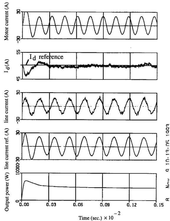
Fig. 11. Simultaneous control of line current, motor current, and biasing current (digital simulation results).
