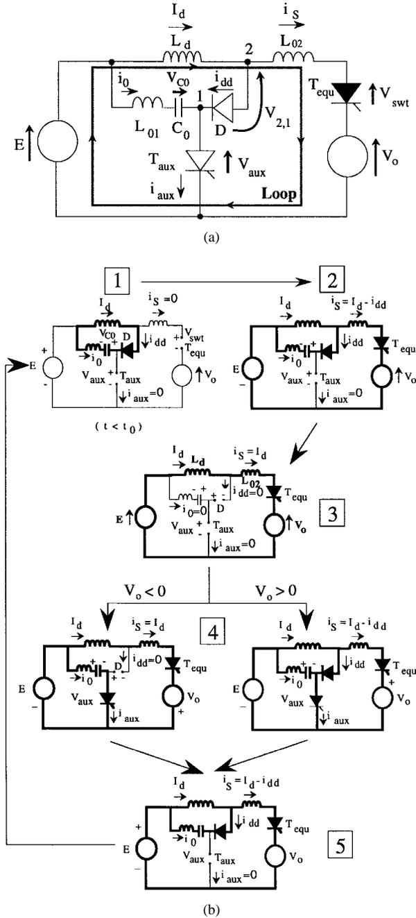
Fig. 2. (a) Mono phase equivalent circuit and (b) circuit states.
