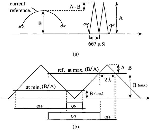
Fig. 14. Illustrations for PWM limits.
