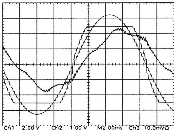
Fig. 21. GDPWM modulation wave, its fundamental component, and the motor current waveforms in the overmodulation range ( $M_i = 0.96$ , 59 Hz, 100%  $T_{eR}$ ) with  $\psi = 30^\circ$ . Scaling: 5 A/div, 2 V/div, and 2 ms/div.
