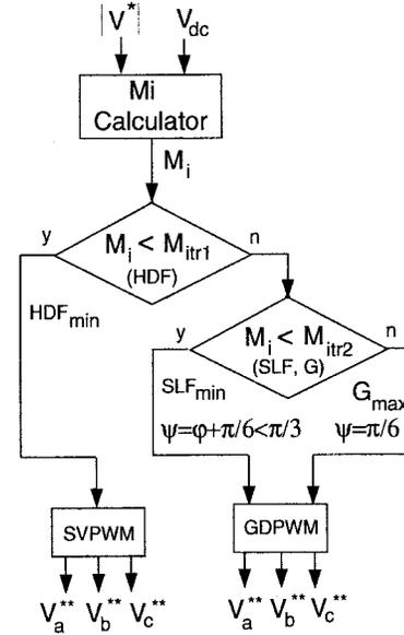
Fig. 13. The combined high-performance PWM algorithm flow diagram.
