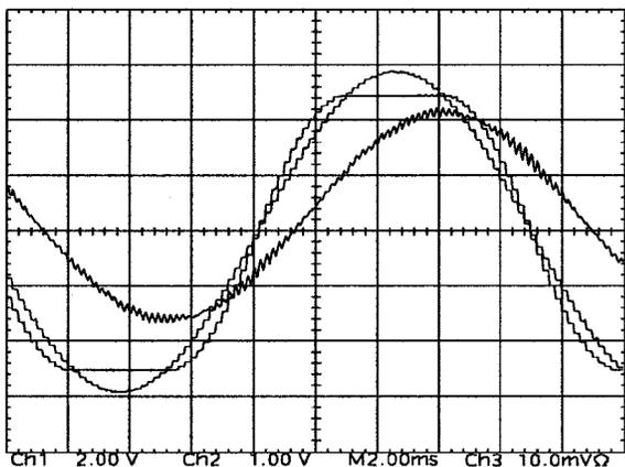
Fig. 20. Experimental GDPWM modulation wave, its fundamental component, and the motor current waveforms ( $M_i = 0.903$ , 56 Hz, 100%  $T_{eR}$ ) with  $\psi = 30^\circ$ . Scaling: 5 A/div, 2 V/div, and 2 ms/div.
