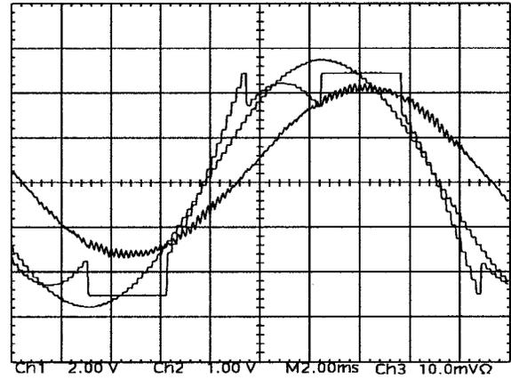
Fig. 18. Experimental GDPWM modulation wave, its fundamental component, and the motor current waveforms ( $M_i = 0.854$ , 53 Hz, 100%  $T_{eR}$ ) with  $\psi = \varphi + 30^\circ \leq 60^\circ$ . Scaling: 5 A/div, 2 V/div, and 2 ms/div.
