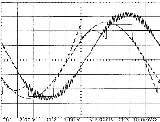
Fig. 17. Experimental GDPWM modulation wave, its fundamental component, and the motor current waveforms ( $M_i = 0.82$ , 51 Hz, 50%  $T_{eR}$ ) with  $\psi = \varphi + 30^\circ \leq 60^\circ$ . Scaling: 2 A/div, 2 V/div, and 2 ms/div.
