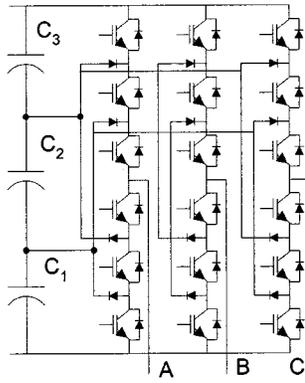
Fig. 1. Four-level inverter (diode clamped topology).
