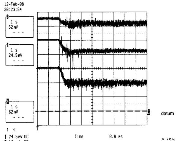
Fig. 19. Dynamic restoration of link voltages using balancing algorithm.
