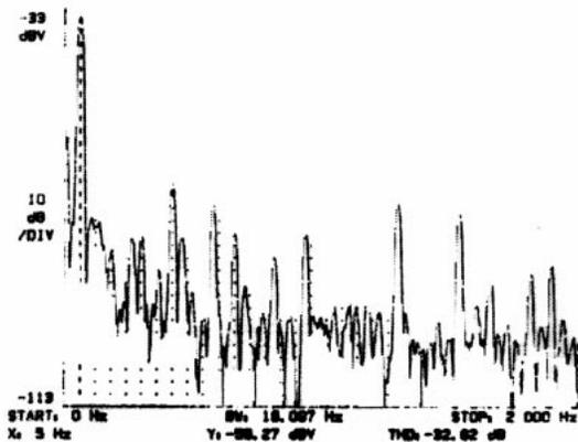
Fig. 17. Current spectrum at rated point of induction motor.
