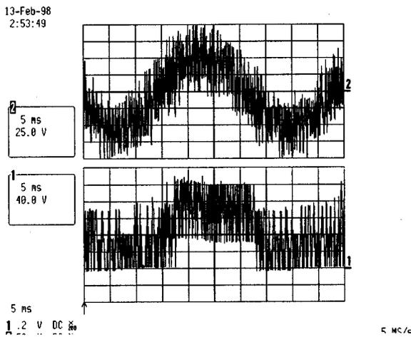
Fig. 16. Experimental waveforms at 450RPM operation. (a) Current (5 A/div) (b) Line voltage (50 V/div).
