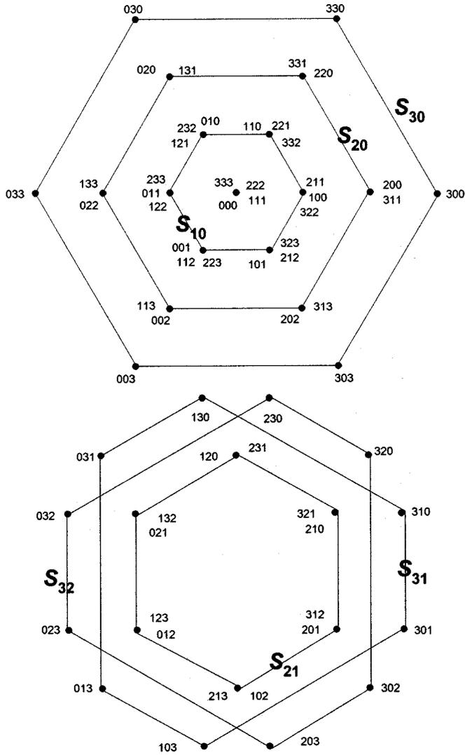
Fig. 4. Inverter switching state classification.
