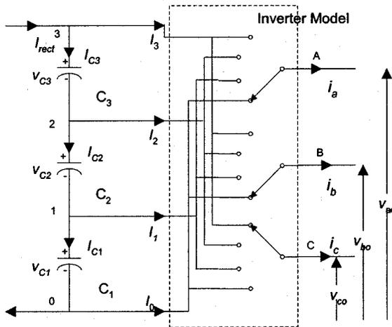
Fig. 2. Terminology for a four-level dc bus.
