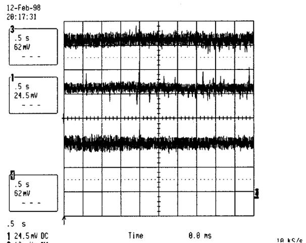
Fig. 8. Voltage balancing using  $X$ -vectors for  $S_{21}$  states.
