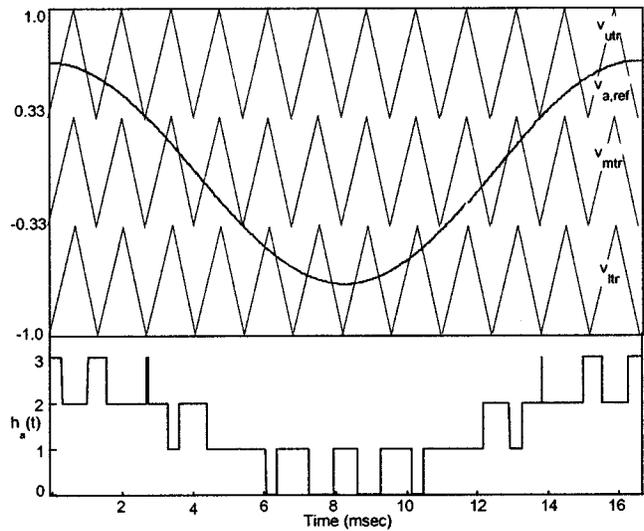
Fig. 10. Four-level sine triangle PWM.
