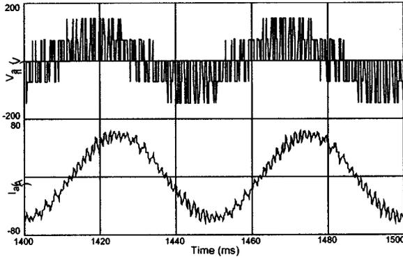
Fig. 12. Simulated plots of motor phase voltage and currents for low speed operation (273 RPM).
