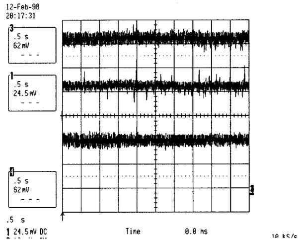
Fig. 18. Balanced dc link voltages in steady state.
