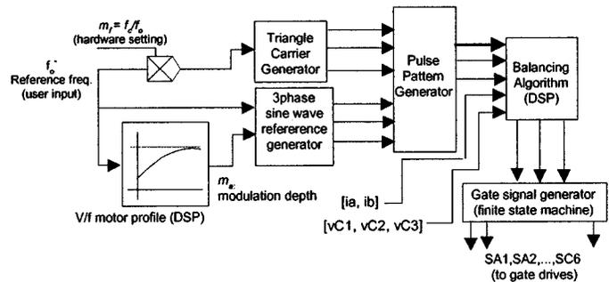
Fig. 11. Control block diagram of drive.
