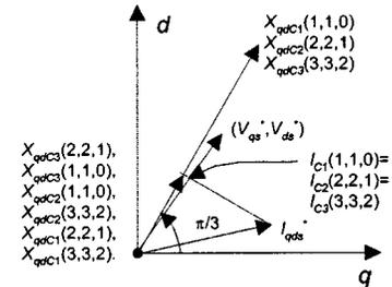
Fig. 7. Voltage balancing using  $X$ -vectors for  $S_{10}$  states.
