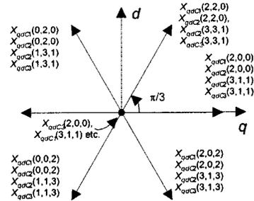
Fig. 6.  $X$  vectors for  $S_{20}$  and  $S_{31}$  states.
