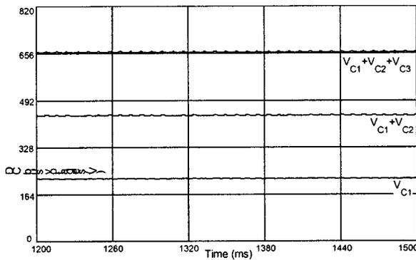
Fig. 13. DC link voltages for low speed operation.
