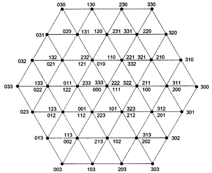
Fig. 3. Four-level inverter switching states in  $dq0$  plane.
