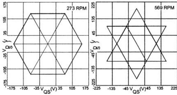
Fig. 14.  $q$  and  $d$  axis voltages for 20 and 40 Hz operation.
