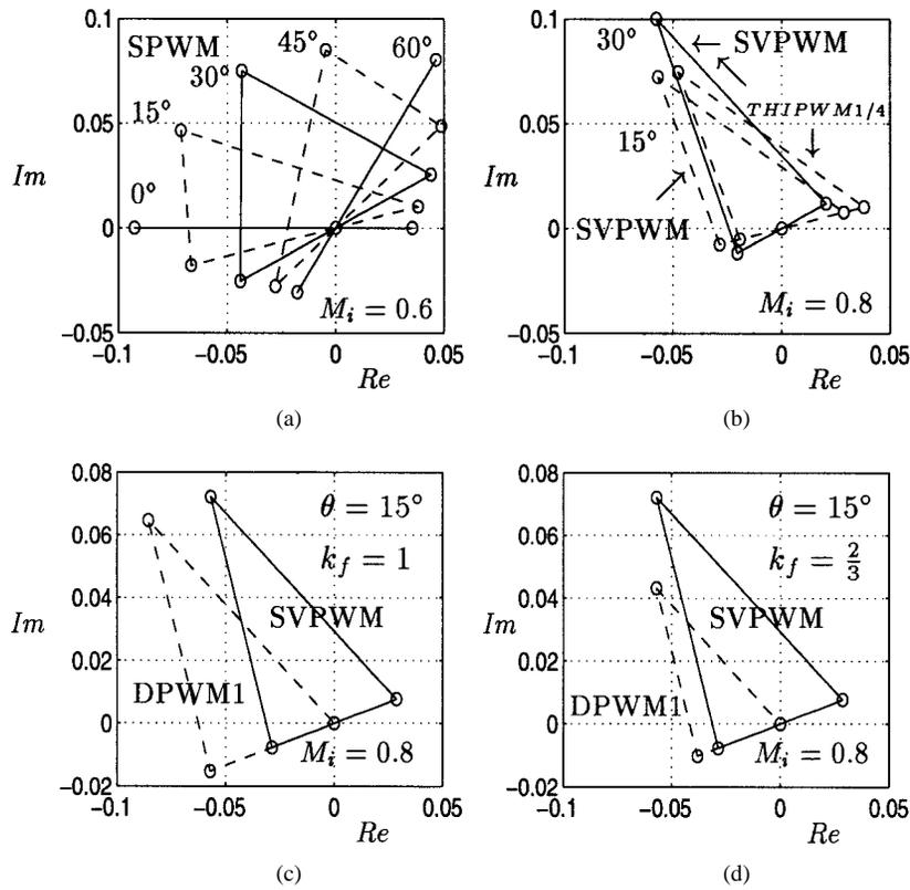
Fig. 10. The switching frequency harmonic flux trajectories of various PWM methods. (a) SPWM, (b) SVPWM and THIPWM1/4 compared for  $w_e t = 15^\circ$  and  $w_e t = 30^\circ$  values, (c) SVPWM and DPWM1 compared ( $k_f = 1$ ), and (d) SVPWM and DPWM1 for  $k_f = \frac{2}{3}$ .
