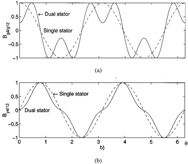
Fig. 2. Normalized flux density distributions for the DSIM. (a) Air gap. (b) Stator yoke.
