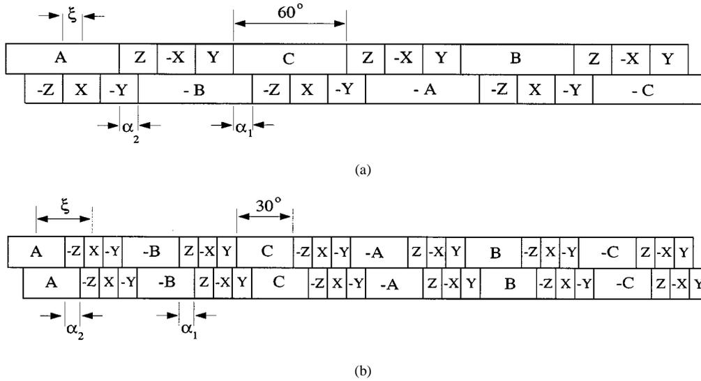
Fig. 6. Winding distribution for (a) fractional pitch and variable displacement angle  $\xi$ ,  $60^\circ$  phase belt. (b) Fractional pitch and variable displacement angle  $\xi$ ,  $30^\circ$  phase belt.
