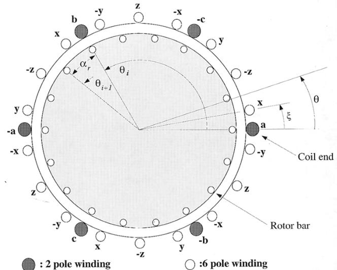
Fig. 5. DSIIM windings distribution.
