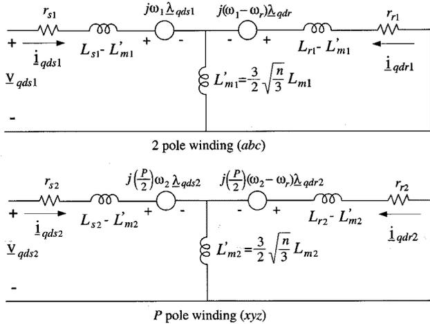
Fig. 8. Complex vector model of the dual stator winding squirrel-cage induction machine.
