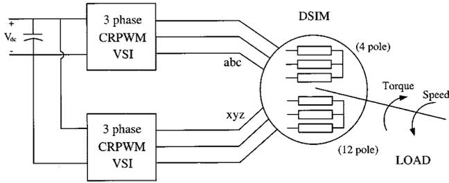
Fig. 1. Dual stator winding induction machine drive (DSIM).
