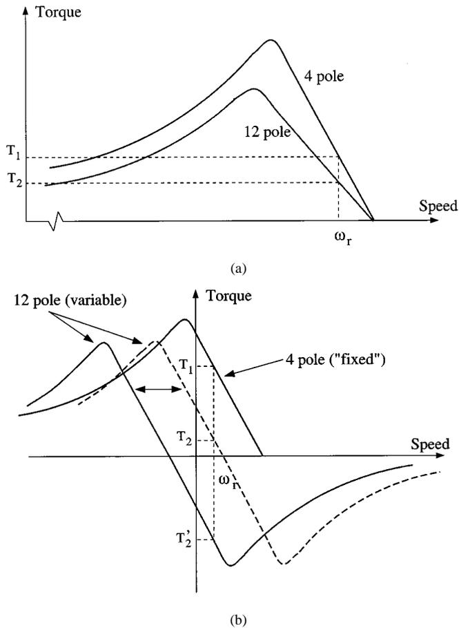
Fig. 4. General control strategy. (a) Synchronous operation. (b) Asynchronous operation.
