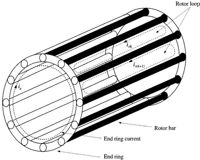
Fig. 7. Rotor current definition.
