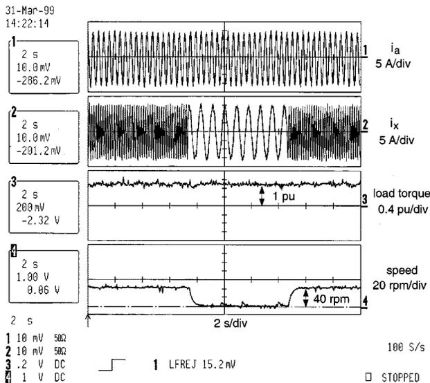
Fig. 14. Constant V/Hz operation in asynchronous mode. From top: phase-a current, phase-x current, load torque, and speed.
