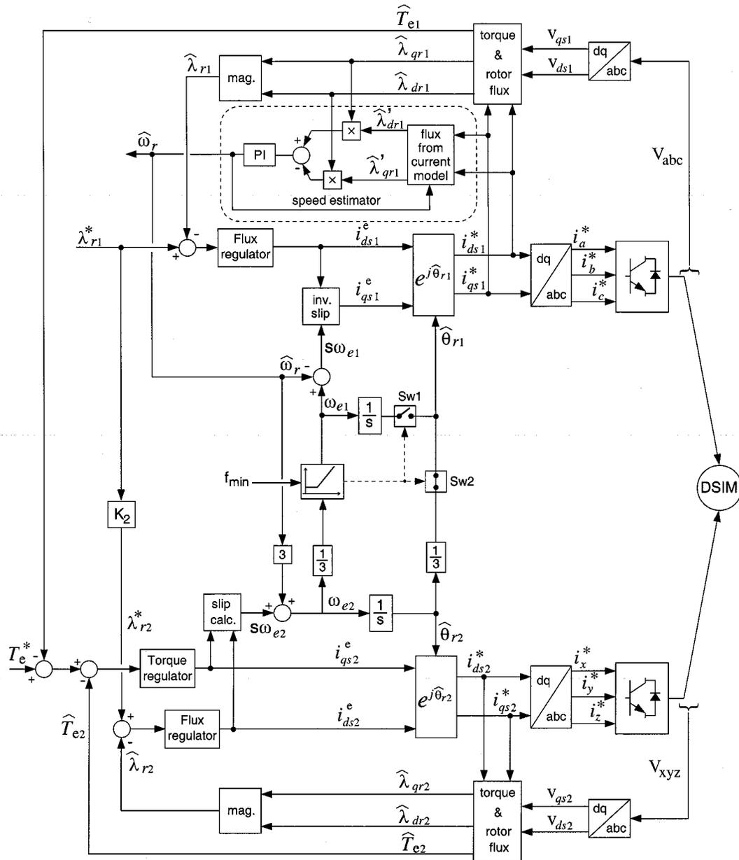
Fig. 11. Proposed control scheme using indirect field orientation.
