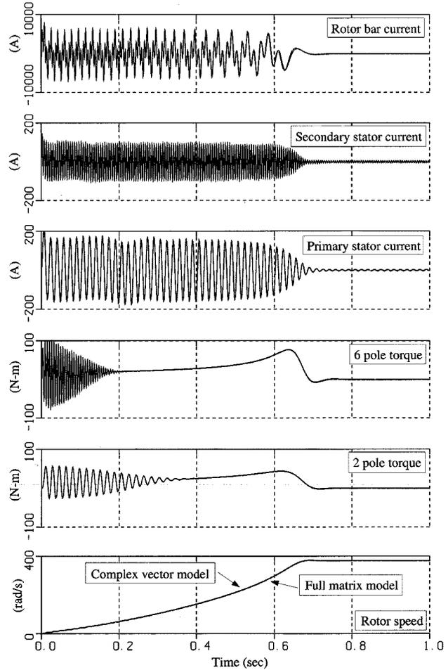
Fig. 9. Full matrix and complex vector model simulation results for a free acceleration run at 60 Hz ( $f_2 = 180$  Hz). Complex vector and full matrix model traces are superimposed.
