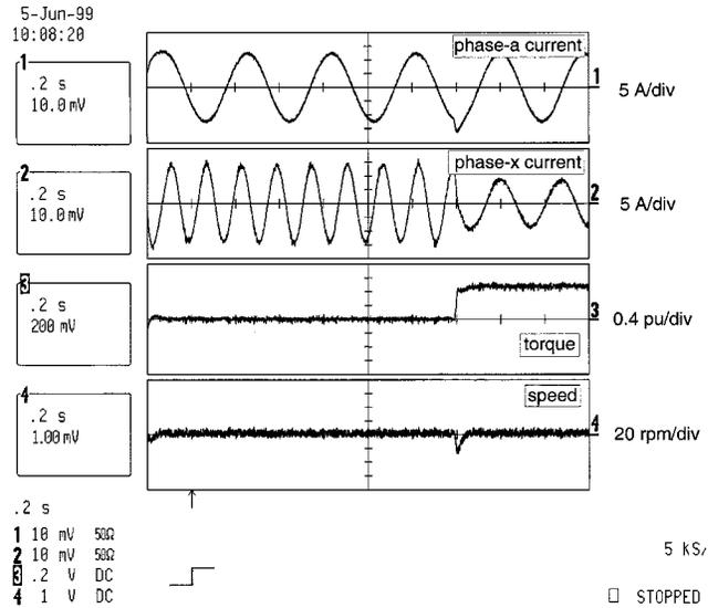
Fig. 15. Indirect field orientation in asynchronous mode. From top: phase-a current, phase-x current, load torque, and speed.
