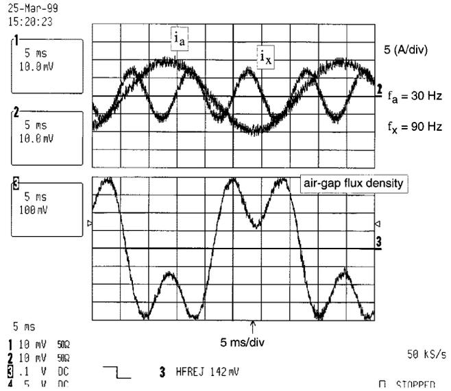
Fig. 3. Measured flux density distribution for the DSIM (top: stator currents; bottom: air gap flux density).
