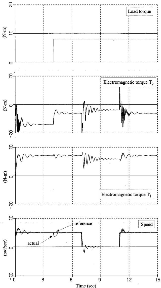
Fig. 12. Constant V/Hz operation at standstill.
