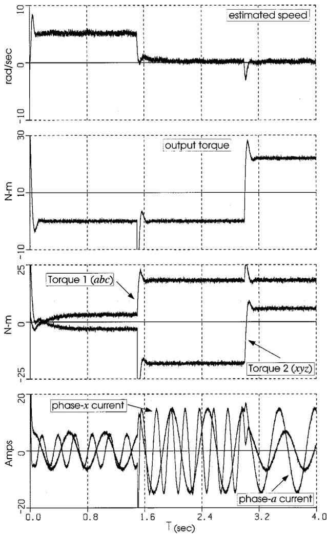
Fig. 13. Direct field orientation during asynchronous operation.
