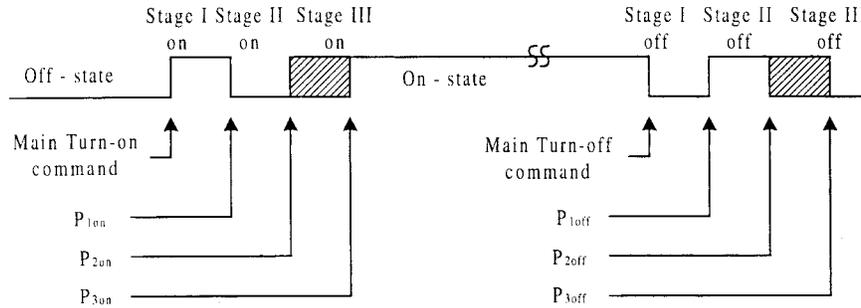
Fig. 2. Timing diagram corresponding to the three-stage active turn-on and turn-off switching.
