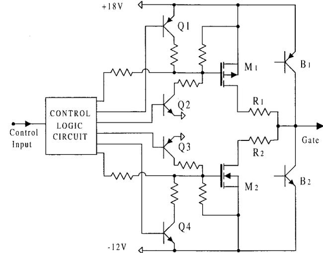
Fig. 4. Schematic of the proposed three-stage AGD circuit.
