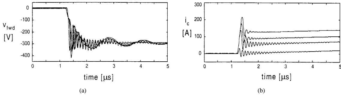
Fig. 6. Measured turn-on waveforms with the CGD at current levels of 0, 50, 80, and 120 A when the gate resistor of  $0.5 \Omega$  is used. (a) The freewheeling diode voltage. (b) The collector current. Other conditions are as follows:  $V_{dc} = 300$  V;  $V_{gg+} = 18$  V;  $V_{gg-} = -12$  V.
