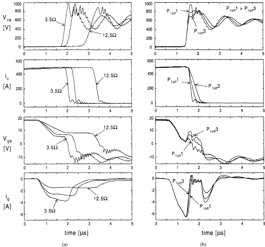
Fig. 10. Measured turn-off switching waveforms ( $v_{ce}$ ,  $i_c$ ,  $v_{ge}$ ,  $i_g$ ) with (a) the CGD and (b) the AGD when the turn-off  $di/dt$  is varied. Turn-off gate resistors used in the CGD for varying  $di/dt$  are 3.5, 5.6, and 12.5  $\Omega$ . Other conditions are as follows:  $V_{dc} = 600$  V;  $I_L = 500$  A;  $V_{gg+} = 18$  V;  $V_{gg-} = -12$  V.
