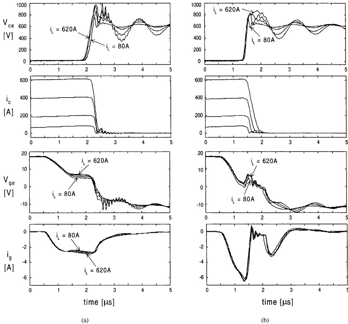
Fig. 9. Measured turn-off switching waveforms ( $v_{ce}$ ,  $i_c$ ,  $v_{ge}$ ,  $i_g$ ) with (a) the CGD and (b) the AGD at current levels of 80, 205, 405, and 620 A. Turn-off gate resistor used in the CGD is 5.6  $\Omega$ . Other conditions are as follows:  $V_{dc} = 600$  V;  $V_{gg+} = 18$  V;  $V_{gg-} = -12$  V.
