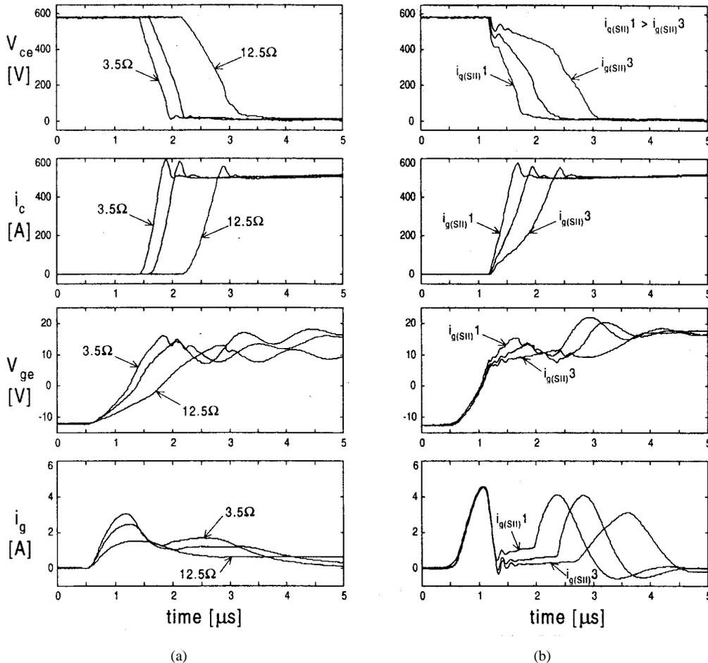
Fig. 7. Measured turn-on switching waveforms ( $v_{ce}$ ,  $i_c$ ,  $v_{ge}$ ,  $i_g$ ) with (a) the CGD and (b) the AGD when the turn-on  $di/dt$  is varied. Turn-on gate resistors used for varying  $di/dt$  in the CGD are 3.5, 5.6, and  $12.5 \Omega$ . Other conditions are as follows:  $V_{dc} = 600$  V;  $I_L = 500$  A;  $V_{gg+} = 18$  V;  $V_{gg-} = -12$  V.
