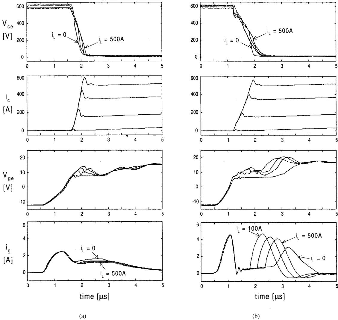
Fig. 5. Measured turn-on switching waveforms ( $v_{ce}$ ,  $i_c$ ,  $v_{ge}$ ,  $i_g$ ) with (a) the CGD and (b) the AGD at current levels of 0, 150, 350, and 500 A. Turn-on resistor of  $5.6 \Omega$  is used in the CGD. Other conditions are as follows:  $V_{dc} = 600$  V;  $V_{gg+} = 18$  V;  $V_{gg-} = -12$  V.
