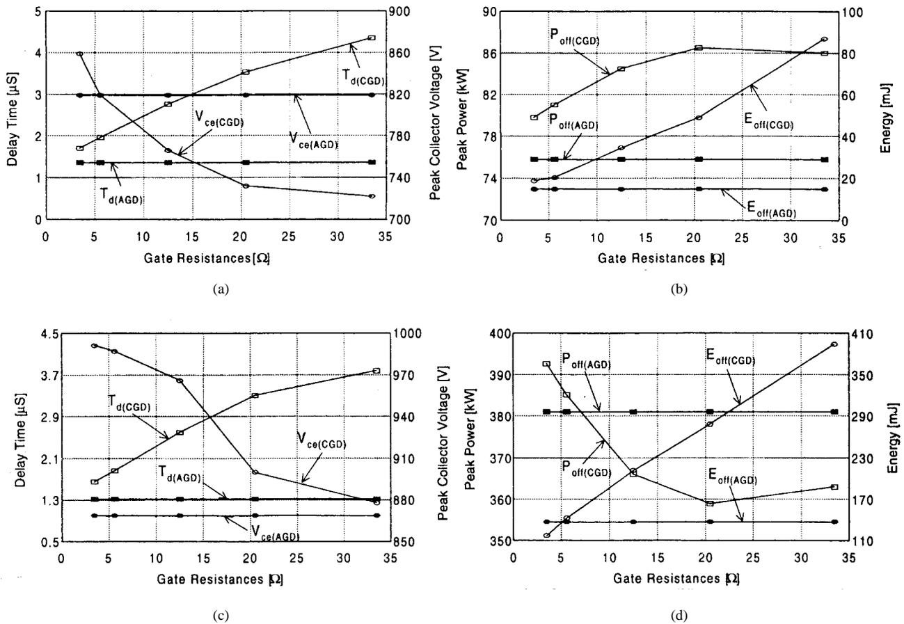
Fig. 12. Comparison of turn-off characteristics between the AGD and the CGD as the gate resistance is varied. (a) and (b)  $I_L = 150$  A. (c) and (d)  $I_L = 620$  A. (a) and (c) Investigate the delay time and the peak collector voltage. (b) and (d) Investigate the peak power and the energy loss. Operating conditions are as follows:  $V_{dc} = 600$  V;  $V_{gg+} = 18$  V;  $V_{gg-} = -12$  V.
