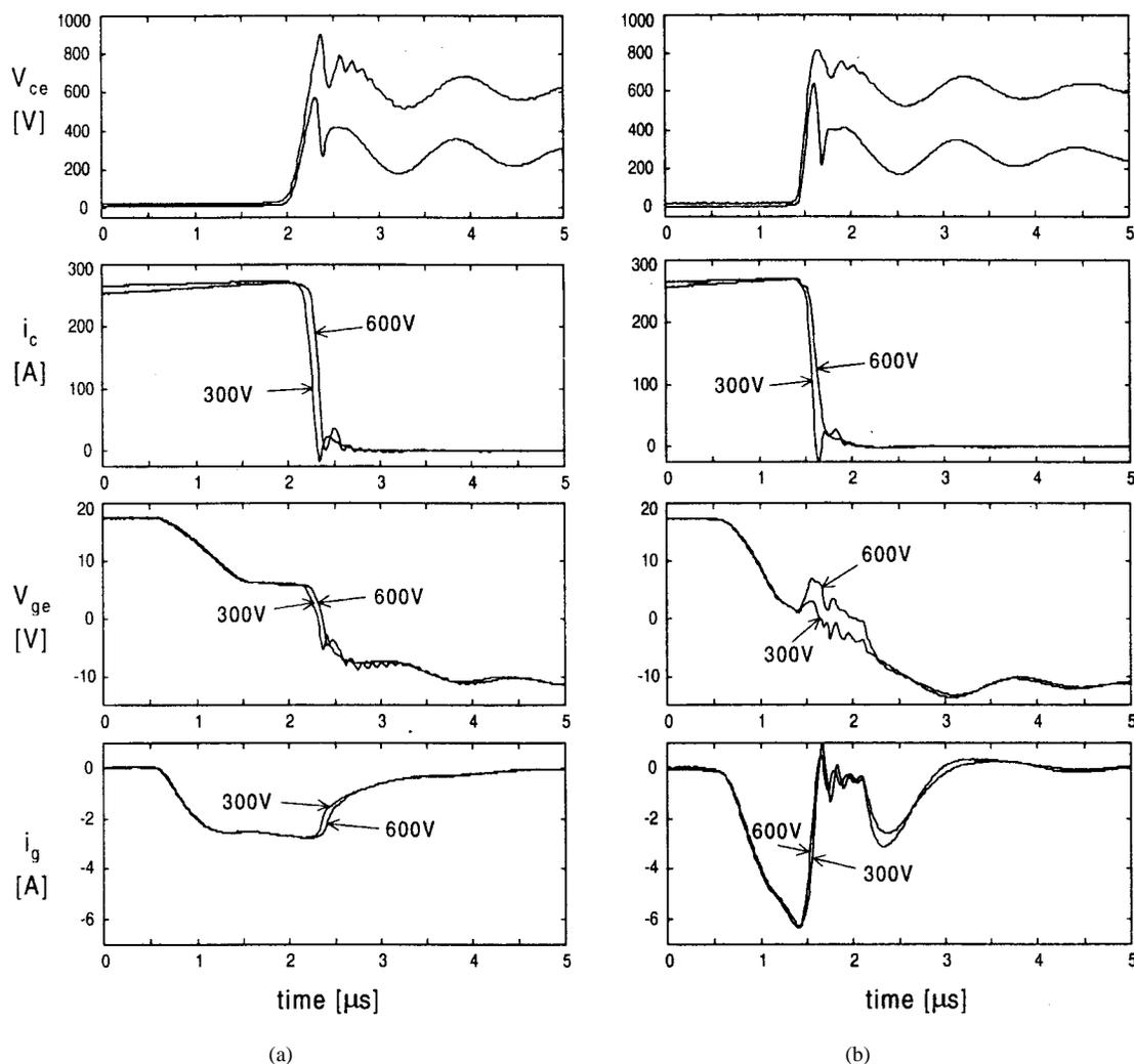
Fig. 11. Measured turn-off switching waveforms ( $v_{ce}$ ,  $i_c$ ,  $v_{ge}$ ,  $i_g$ ) with (a) the CGD and (b) the AGD when the dc-bus voltage is varied. The dc-bus voltages are 300 and 600 V. Turn-off gate resistor used in the CGD is  $5.6 \Omega$ . Other conditions are as follows:  $I_L = 270$  A;  $V_{gg+} = 18$  V;  $V_{gg-} = -12$  V.
