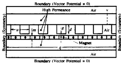
Fig. 6 Analyzed model for measuring  $V$
