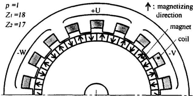
Fig. 1 Permanent Magnet Vernier Machine
