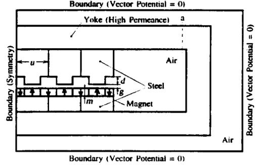
Fig. 3. Analyzed model of an ED array
