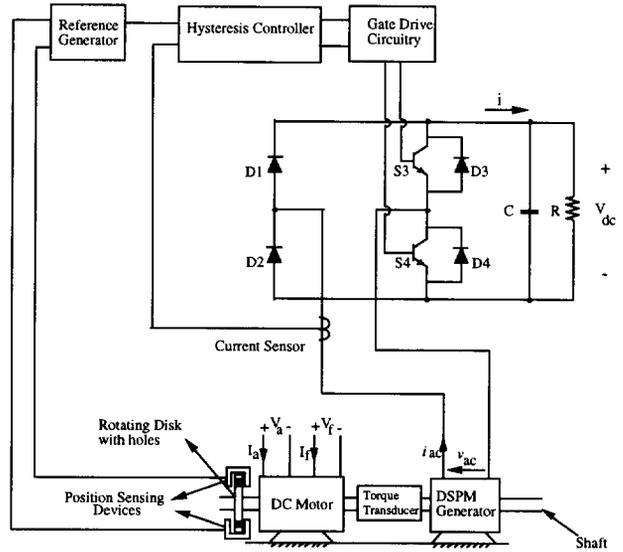
Fig. 10 Schematics of implementation of the boost converter with hysteresis current controller
