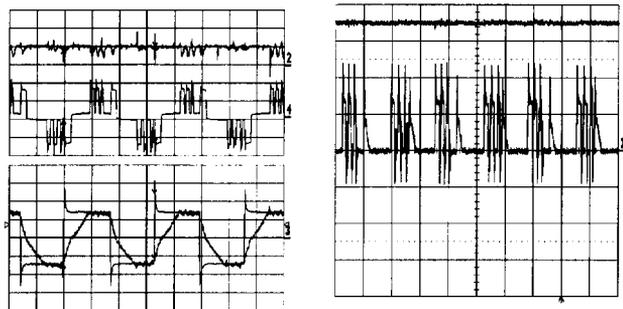
Fig. 12 **Left:** Torque 150 inch-lbs/V, AC voltage (25 V/div) (moved down by 1.8 divisions for clarity of illustration), Current reference (50A/div), Current (50A/div) at 3000RPM **Right:** DC voltage (10 V/div) and DC current (50 A/div) at 3000 RPM
