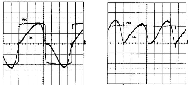
Fig. 7 Left: AC output voltage (10 V/div) and AC output current (20A/div) of the DSPM generator Right: DC load voltage (10 V/div) and DC load current (20A/div) of the DSPM generator
