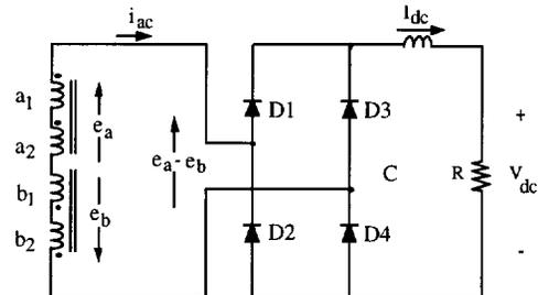
Fig. 1 Rectification with constant dc current.
