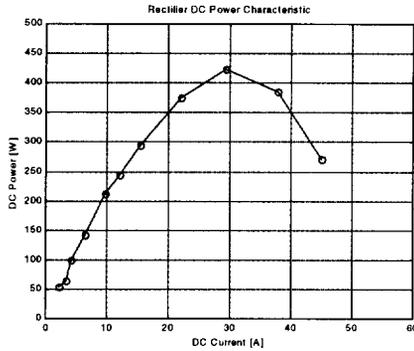
Fig. 9 DC current and DC power characteristic
