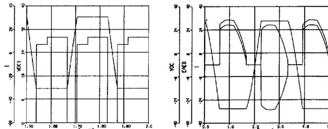
Fig. 5 Left: First Order Approximation Simulation Results: Rectified voltage  $v_{dc}$  and ac current  $i$ . Right: Nonlinear Simulation Results: Rectified voltage  $v_{dc}$ , voltage  $e_a-e_b$  ( $v_{ac}$ ), and ac current
