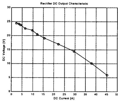
Fig. 8 DC current and DC voltage characteristic
