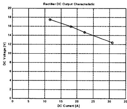
Fig. 3 DC current and DC voltage relationship for constant current rectifier
