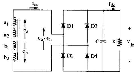
Fig. 6 Rectification with constant dc current.
