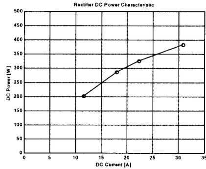
Fig. 4 DC current and DC power relationship for constant current rectifier
