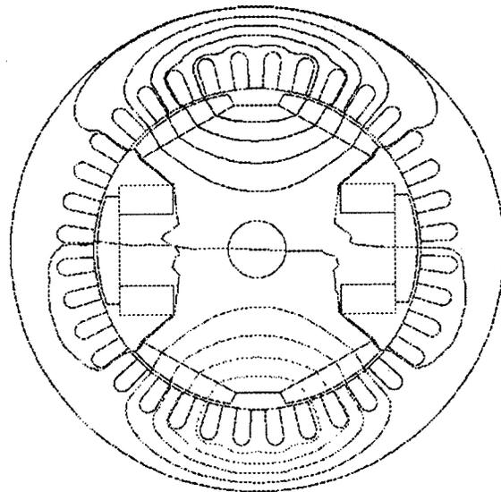
Fig. 17. Flux lines of a 6 pole SynPM machine with zero field current.
