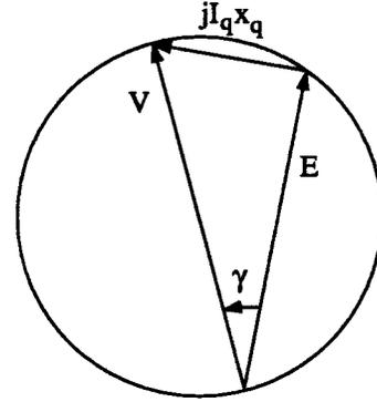
Fig. 8. Circle of voltage equation neglecting resistance.
