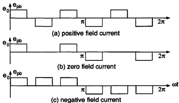
Fig. 4. Back EMF of a phase belt winding.
