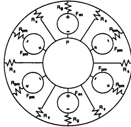
Fig. 3. Magnetic circuit model of 6 pole SynPM machines.
