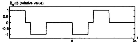
Fig. 12. Air gap flux density produced by PM.
