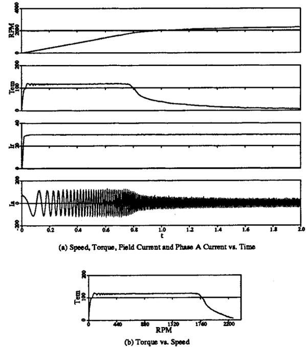
Fig. 14. Simulation of SynPM machine, without field current regulation.
