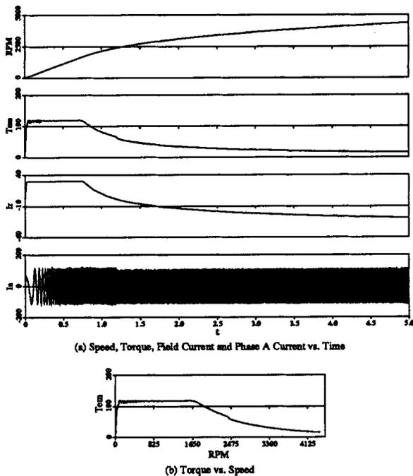
Fig. 15. Simulation of SynPM machine with field current regulation.
