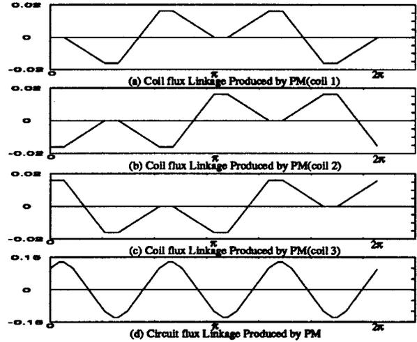
Fig. 13. Calculated flux linkages of coils and circuit.
