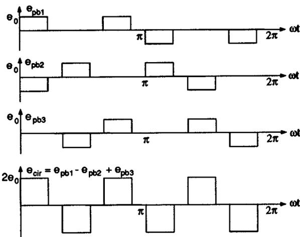
Fig. 6. Back EMF of one circuit with zero excitation.
