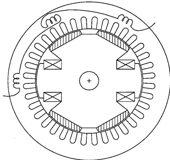
Fig. 1. Structure of SynPM machine.
