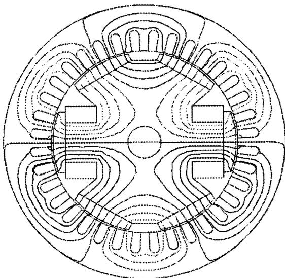
Fig. 16. Flux lines of a 6 pole SynPM machine with full positive field current.
