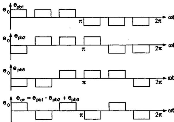
Fig. 7. Back EMF of one circuit with full negative excitation.
