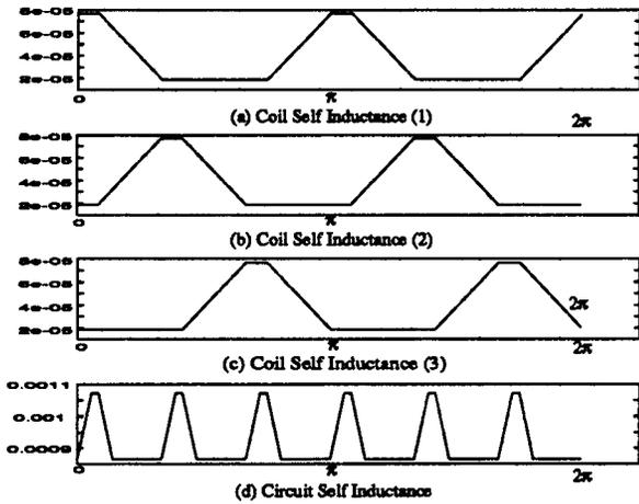
Fig. 11. Calculated coil and circuit inductances.
