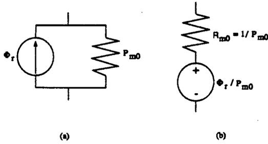
Fig. 2. Equivalent circuit of permanent magnet.
