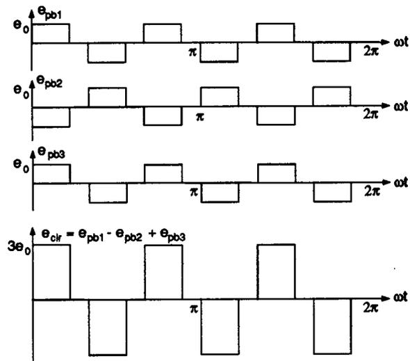
Fig. 5. Back EMF of one circuit with full positive excitation.
