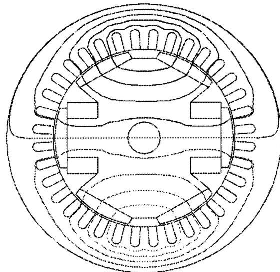
Fig. 18. Flux lines of a 6 pole SynPM machine with full negative field current.
