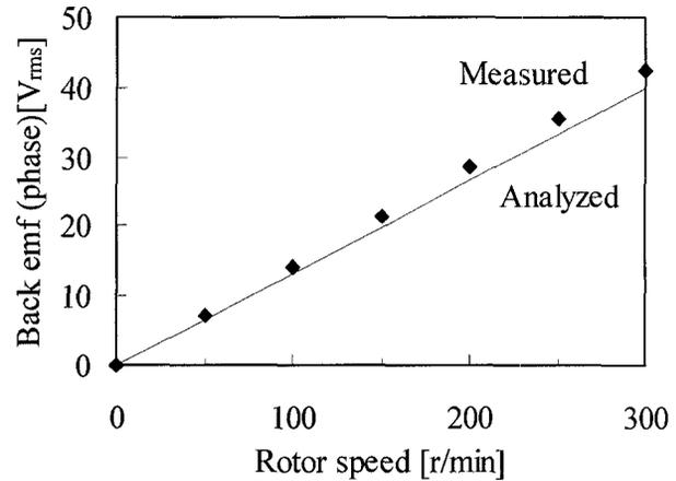
Fig. 11 Back-emf v.s. rotor speed
