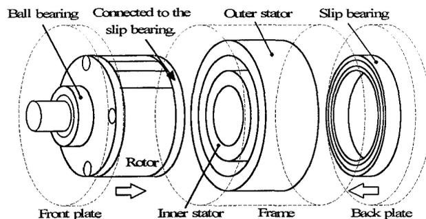
Fig. 8 Assembly of the prototype machine
