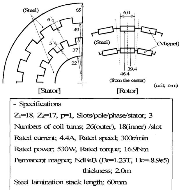
Fig. 6 Dimensions and specs of the prototype DEPMM
