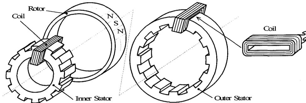
Fig. 5 Concept of the Dual-Excitation Permanent magnet Vernier machine
