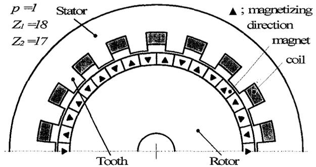
Fig. 1 Typical configuration of the PMVM
