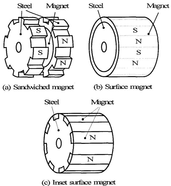
Fig. 4 Three types of the rotor structures
