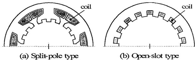
Fig. 3 Two types of the stator configurations
