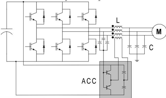
Figure 6. Simplified schematic of a VSI with active common-noise canceler.
