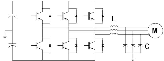
Figure 4. Simplified schematic of a VSI with differential/common mode L-C filter.
