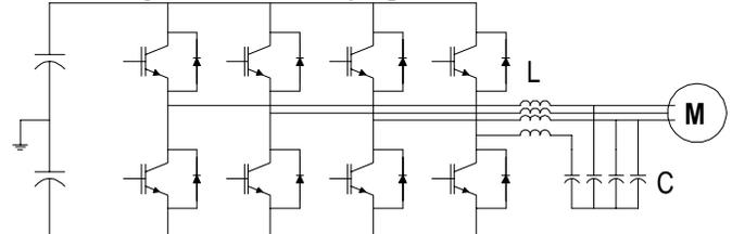
Figure 7. Simplified schematic of a VSI with four legs to impose symmetrical switching.
