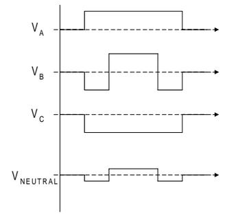
Figure 16. Waveforms with AZSS.
