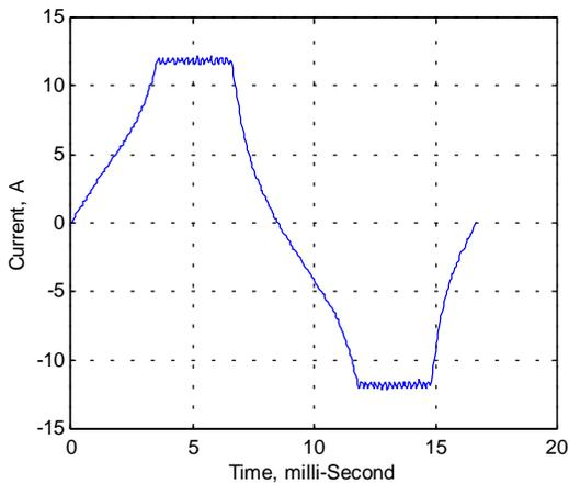
Fig. 14. One cycle machine current waveform at 200 RPM
