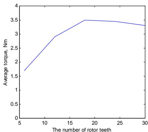
Fig. 6: The effect of number of flux loops over torque capability
