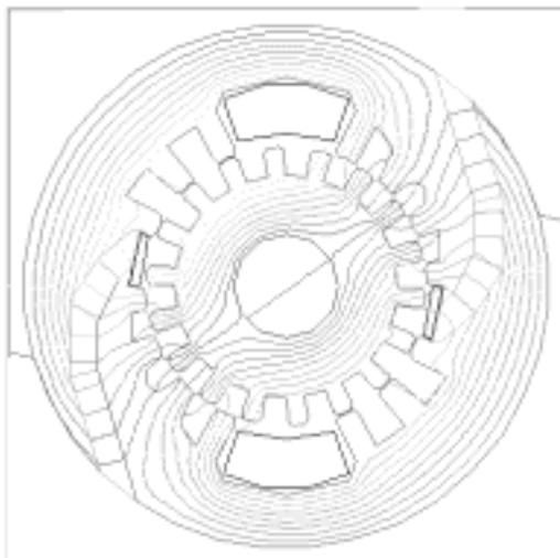
Fig. 7: Flux distribution with a negative armature current
