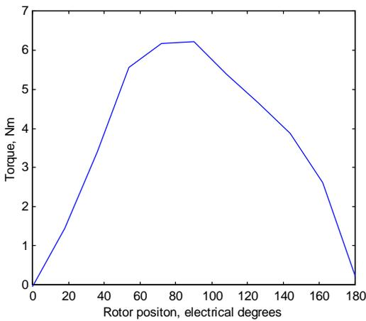
Fig. 9. Torque waveform with rotor position
