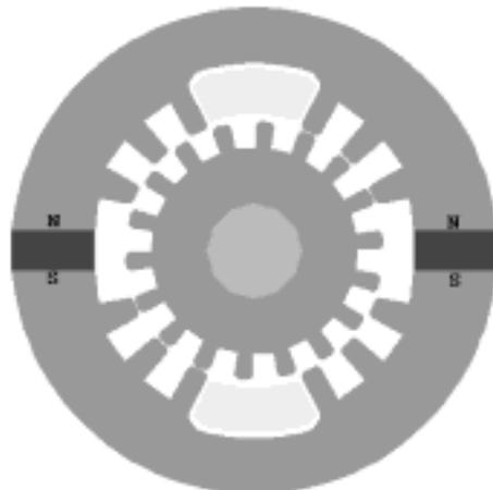
Fig. 3: A 2-D TM machine using rare earth magnets
