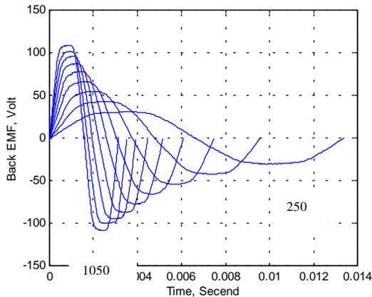
Fig. 13. Back EMF for speeds 250~1,050 RPM, 100 RPM increments
