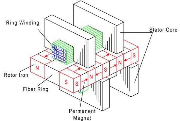
Fig. 1 Transverse Flux Machine proposed by H. Weh
