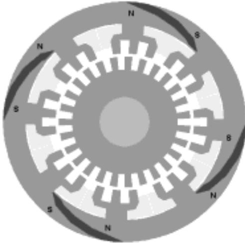
Fig. 10 Two phase spiral magnet machine
