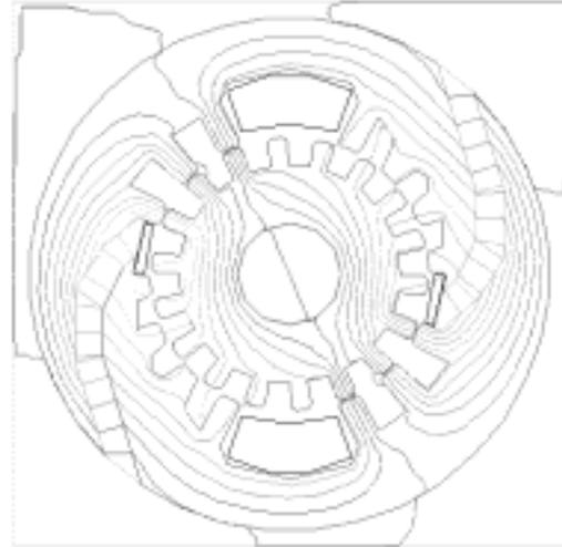
Fig. 5: Flux distribution with zero armature current
