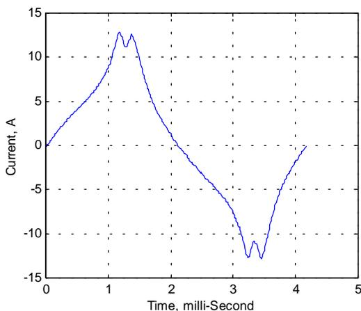
Fig. 15 One Cycle of Machine Current Waveform at 1000 RPM
