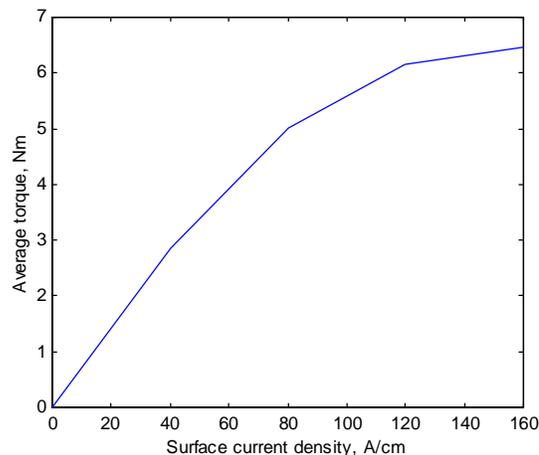
Fig. 8: Torque-current relation due to armature reaction
