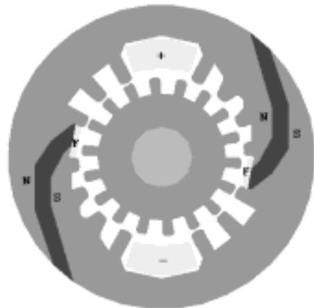
Fig. 2: The SMTM machine using ceramic magnets
