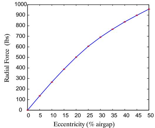
Fig. 8 Radial force –vs– eccentricity, 18/12 SRM, 90 amps and 100% alignment.
