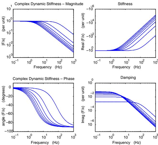
Fig. 12 Radial force frequency response to eccentricity variations.
