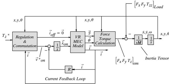
Fig. 9 Dynamic simulation model of the SR system.
