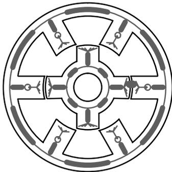
Fig. 1 Simplified MEC representation for a 6/4 SRM
