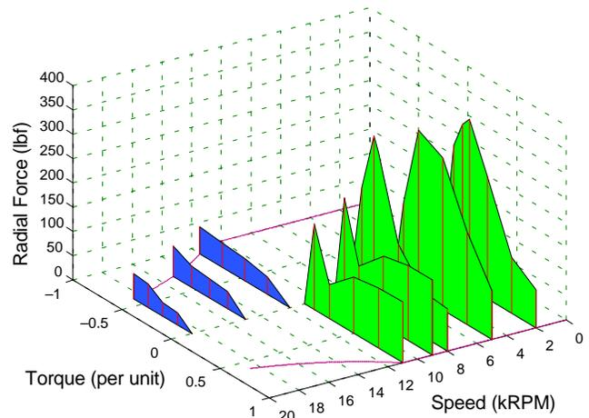
Fig. 13 Radial force -vs- Torque-speed operating point, 18/12 SRM, 33% eccentricity.
