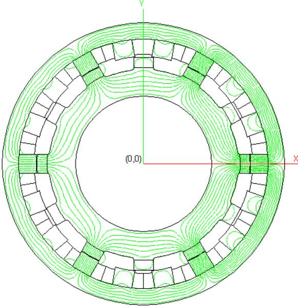
Fig. 2 FEA Flux plot for an 18/12 SRM with a 33% gap eccentricity.
