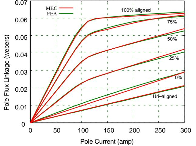
Fig. 3 Flux Linkage Characteristics, 18/12 SRM – Comparison of MEC & FEA
