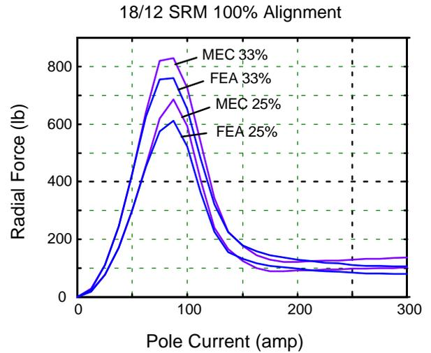
Fig. 5 Radial force –vs– pole current, 18/12 SRM, 25% & 33% gap offset in rotor position.
