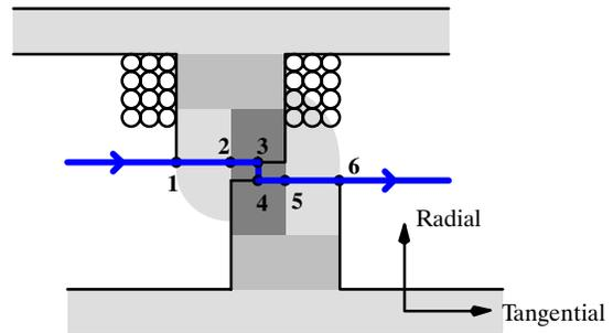
Fig. 4 Application of the Maxwell Stress Tensor in the calculation of radial and tangential forces.
