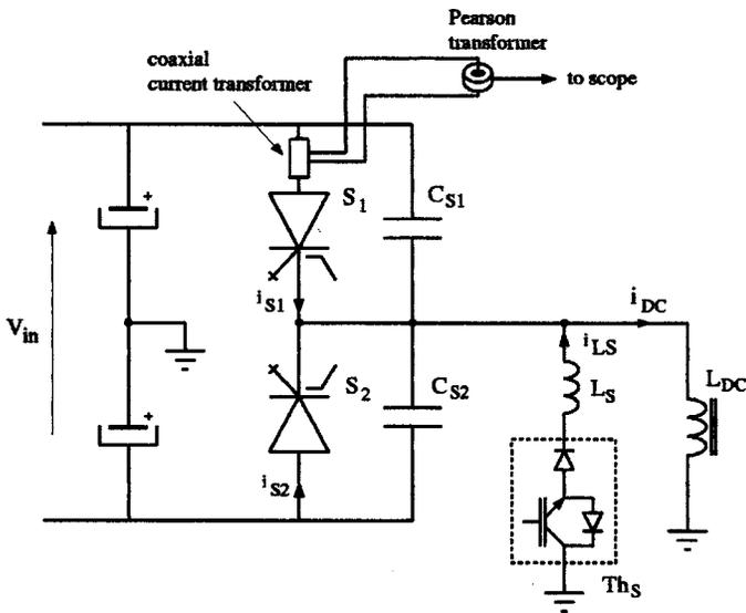
Fig. 4. High-power (pulsed) test setup employing MTOs.
