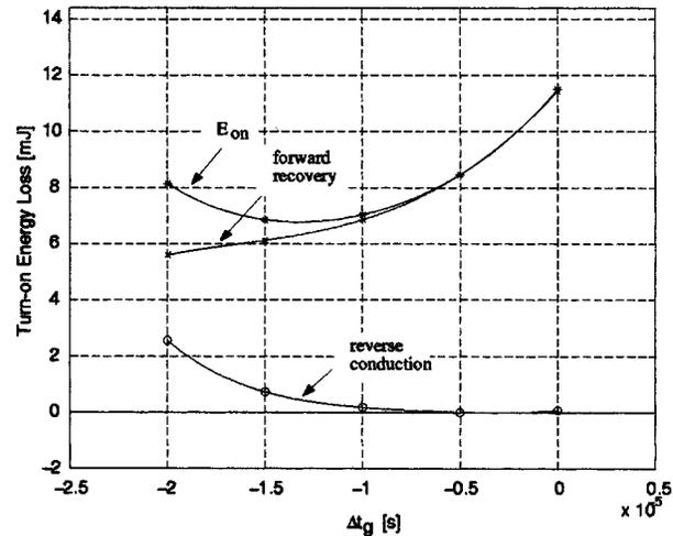
Fig. 8. Passive commutation: turn-on energy loss.
