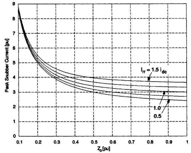
Fig. 12. Active commutation: current stress due to large  $I_{rr}$ .
