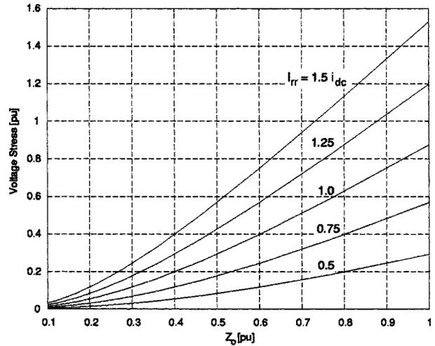
Fig. 11. Active commutation: voltage stress due to large  $I_{rr}$ .
