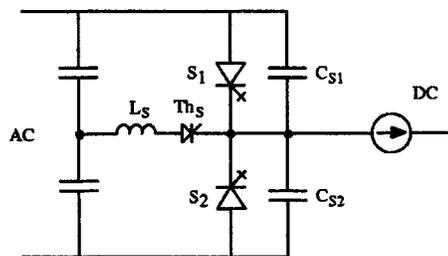
Fig. 2. Basic realizations of the resonant snubbers in CSC.
