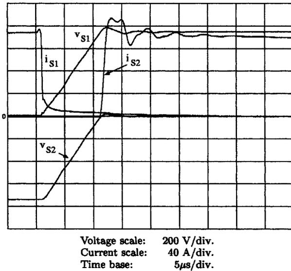
Fig. 7. Passive commutation sequence.
