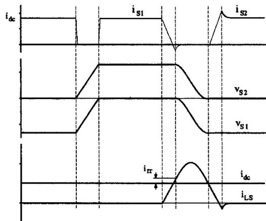
Fig. 3. Basic waveforms of the CSC with resonant snubbers.
