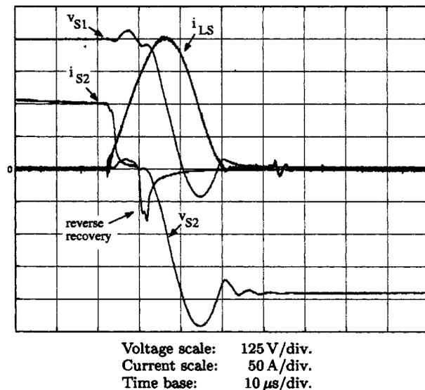
Fig. 10. Active commutation waveforms: snubber voltage boost.
