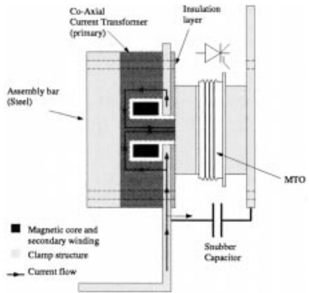
Fig. 5. Detail of the assembly of the coaxial current transformer.
