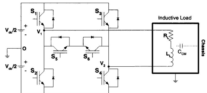
Fig. 1. Schematic diagram of modified single phase topology.
