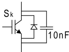
Fig. 2. Snubber configuration of laboratory prototype inverter.
