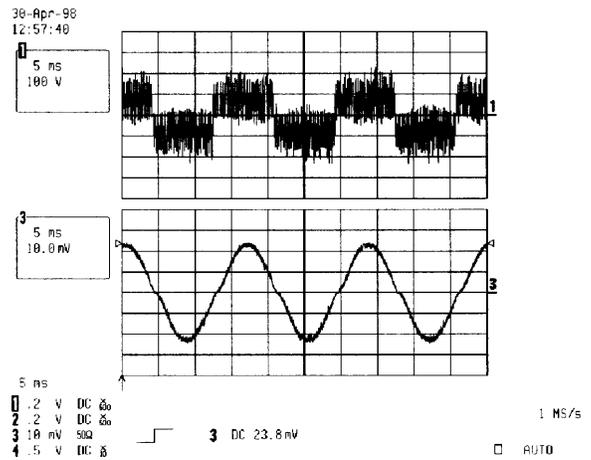
Fig. 4. Load voltage and current waveforms for proposed topology. (a) Upper trace: Voltage (100V/Div) (b) Lower trace: Current (10A/Div).
