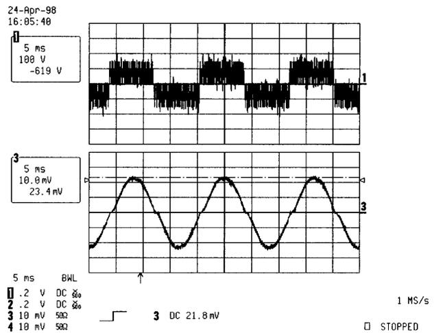
Fig. 3. Load voltage and current waveforms for conventional topology. (a) Upper trace: Voltage (100V/Div) (b) Lower trace: Current (10A/Div).
