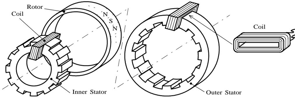
Fig. 2 Structure of the Dual-Excitation Permanent Magnet Vernier Machine
