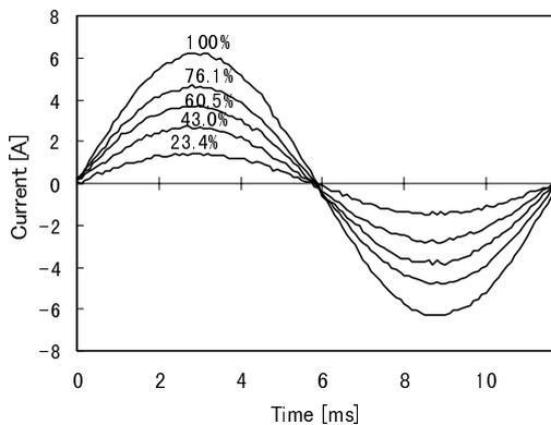
(a) Current waveforms of various values of load
