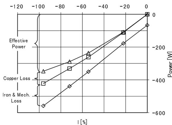
Fig. 10 Power flow of the prototype at 300r/min.
