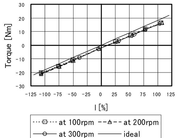
Fig. 9 Torque vs. Current characteristics
