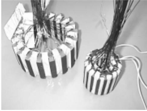
(a) Outer (left) and inner (right) stators with coils
