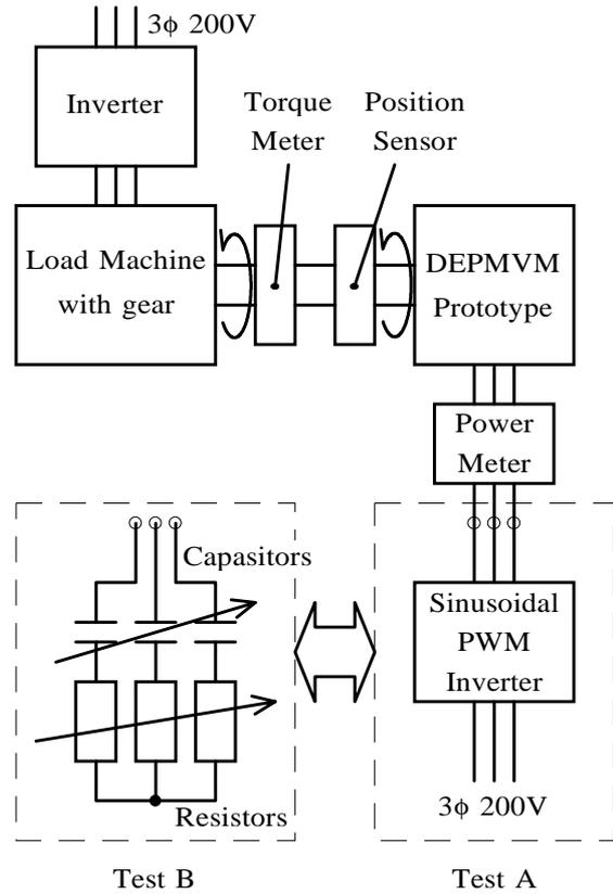
Fig. 6 Schematic of the experimental setups
