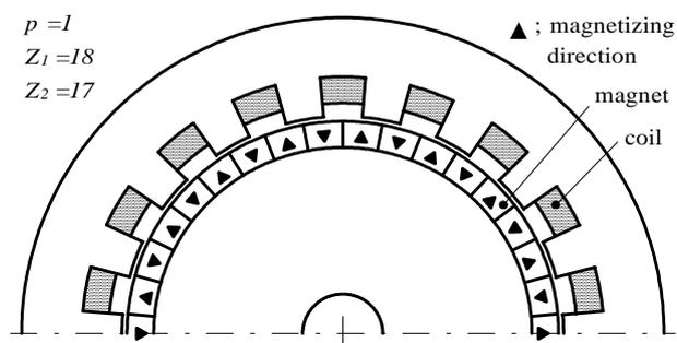
Fig. 1 Permanent Magnet Vernier Machine
