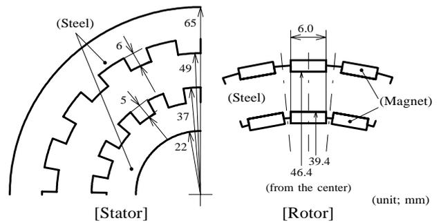
Fig. 3 Major dimensions of the prototype DEPMVM
