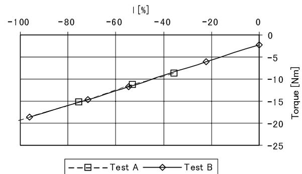
Fig. 11 Torque vs. current characteristics in Test A and Test B (300/min)
