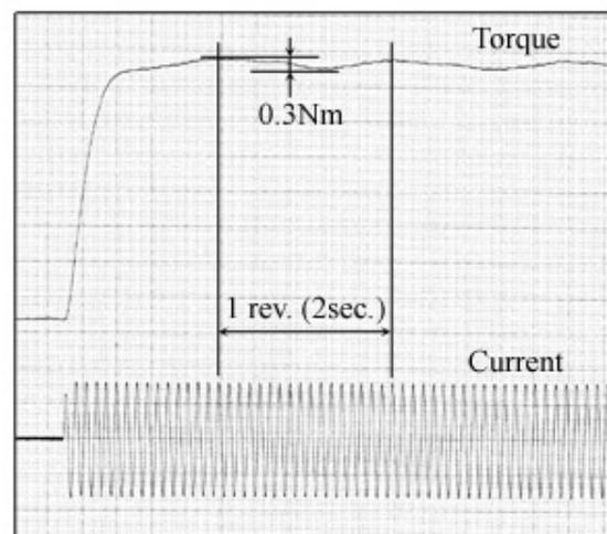
Fig. 12 Shaft torque of the prototype with short-circuited coils (10r/min.)
