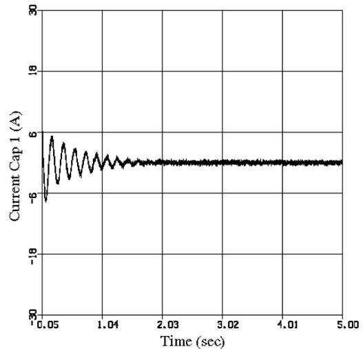
Fig. 7. Straight-line regime: DC-link capacitor current with the same load (4 N.m) and same speed (36 rad/sec) in both motors.
