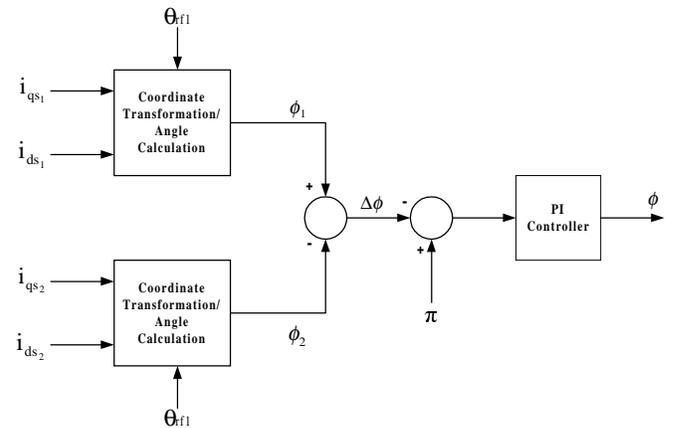
Fig. 2. Active calculation of the rotation angle  $\phi$ .
