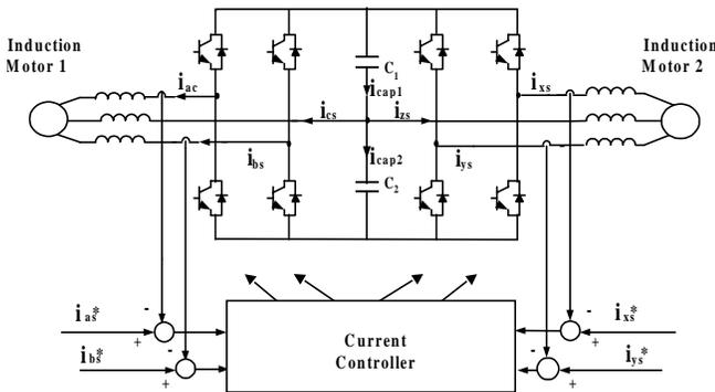
Fig. 1. Reduced switch count three-phase dual drive.
