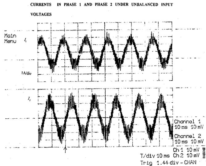
Fig. 12. Currents in phase 1 and 2 under unbalanced input voltages (experimental results).
