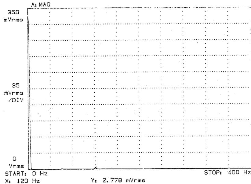
Fig. 14. Frequency spectrum of the output dc voltage (experimental results).
