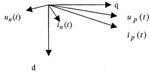
Fig. 3. The positive and negative sequence input voltages and currents in  $d$ - $q$  stationary frame.
