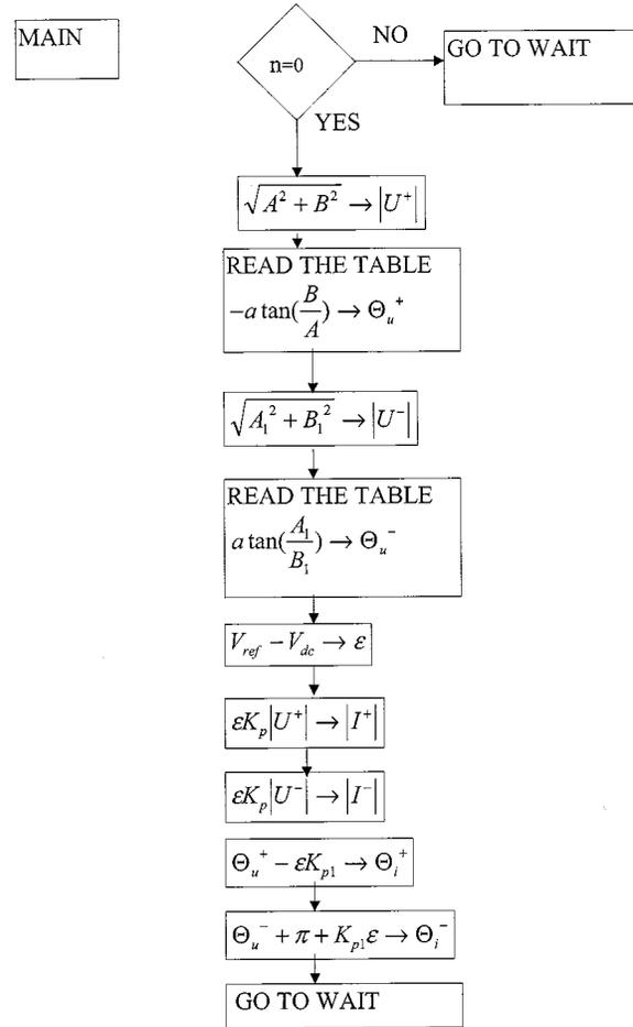
Fig. 11. Flowchart of the main loop (MAIN).
