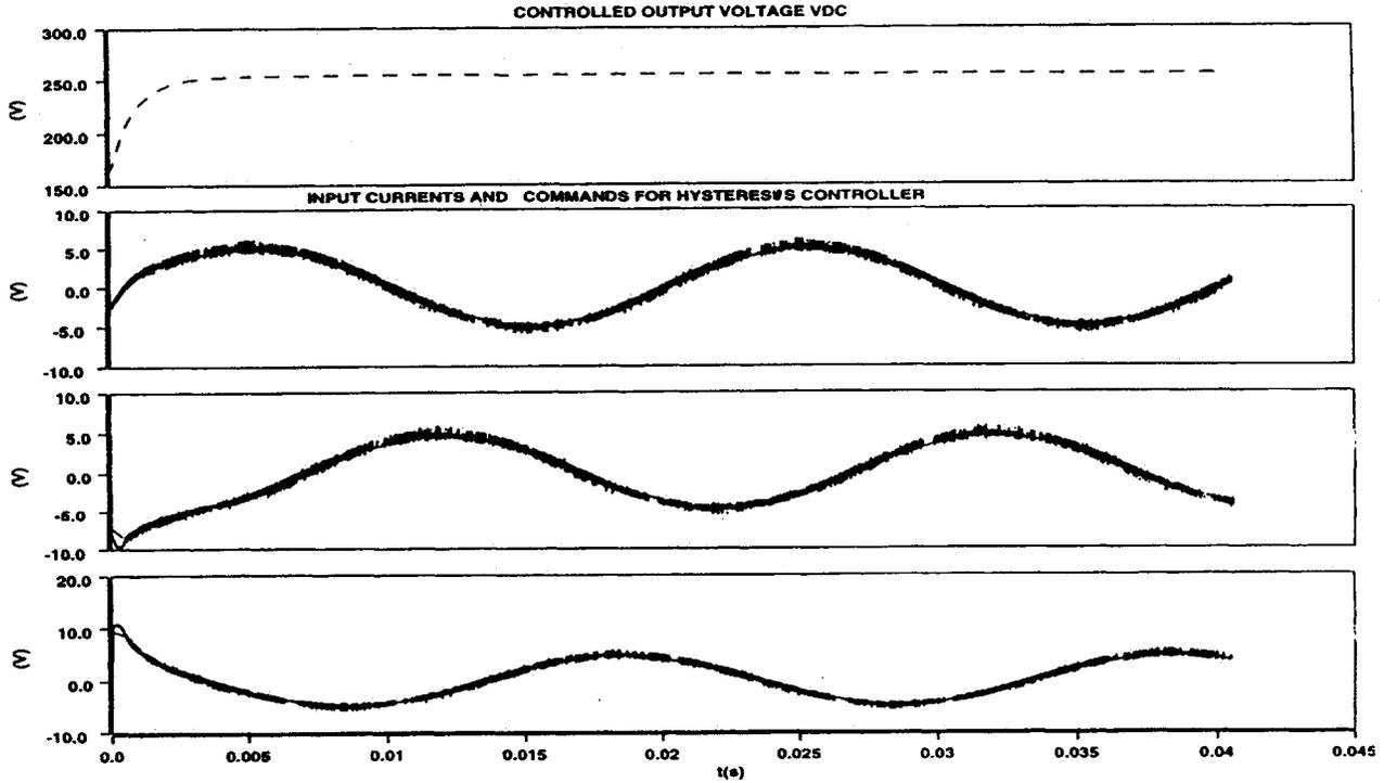
Fig. 6. Controlled output voltage, input currents, and commands for the hysteresis controllers (simulation results).
