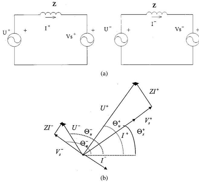
Fig. 2. (a) Per-phase positive and negative sequence equivalent circuit. (b) Graph representation of the proposed solution for harmonic elimination.
