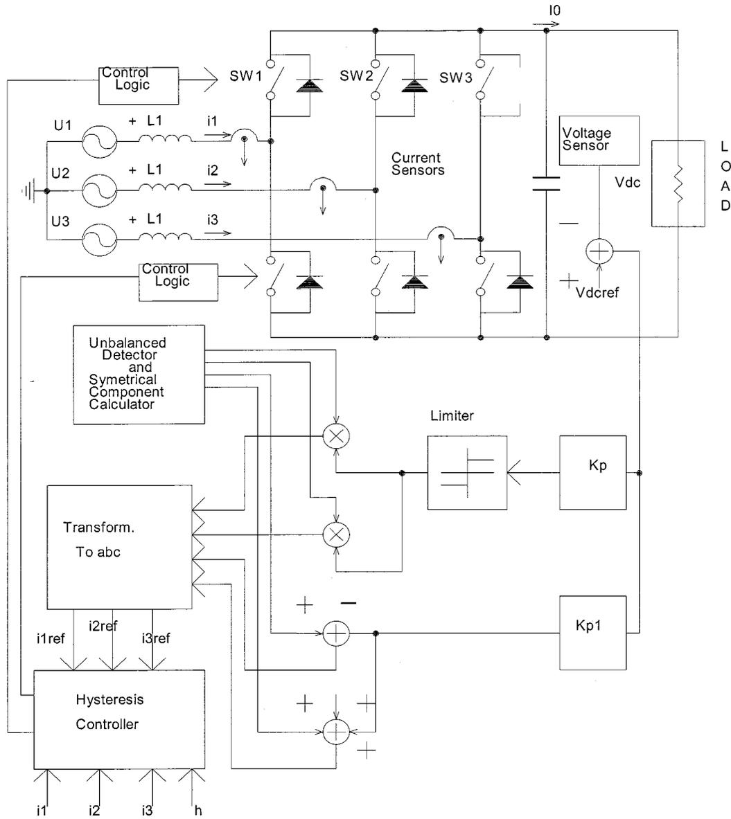
Fig. 5. Proposed control loop solution under unbalanced input voltages.
