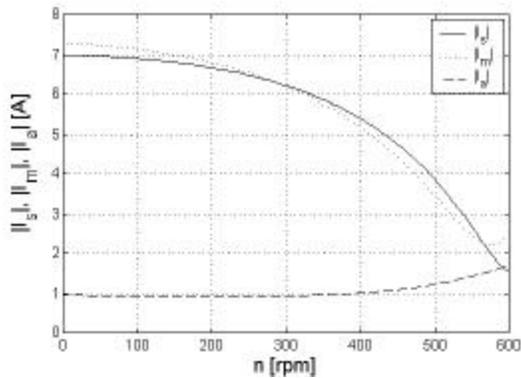
Fig. 7. Stator currents-speed characteristics,  $f = 30$  Hz.
