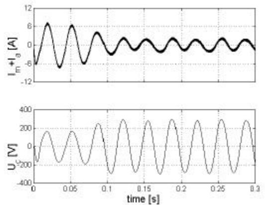
Fig. 11. Stator current and voltage across AC capacitor at start,  $f = 30$  Hz.
