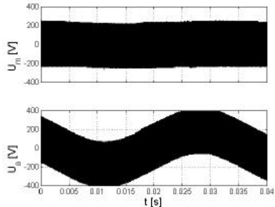
Fig. 16. Stator voltages,  $f = 30 \text{ Hz}$ ,  $C = 30 \mu\text{F}$ .
