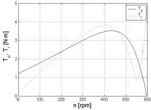
Fig. 6. Torque-speed characteristics,  $f = 30$  Hz.
