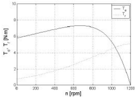
Fig. 2. Torque-speed characteristics,  $f = 60$  Hz.
