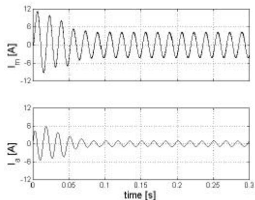
Fig. 5. Stator currents at start,  $f = 60$  Hz.
