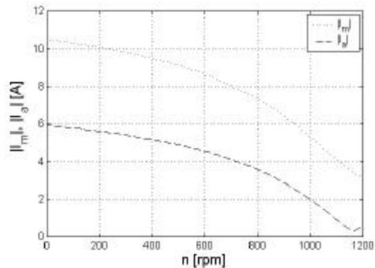
Fig. 3. Stator currents-speed characteristics,  $f = 60$  Hz.
