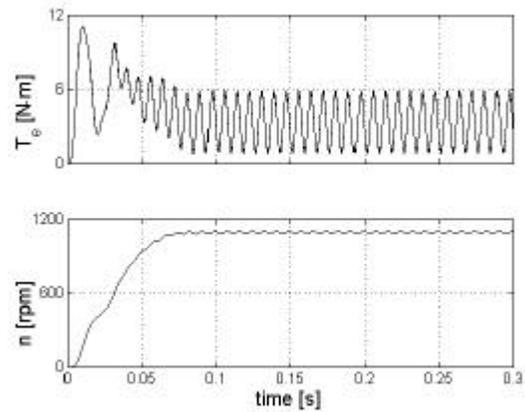
Fig. 4. Torque and speed at start,  $f = 60$  Hz.
