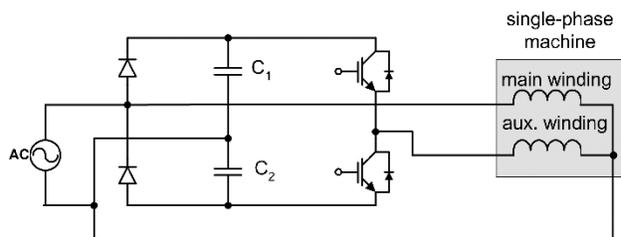
Fig. 6. Scheme of system under investigation, full-speed mode.
