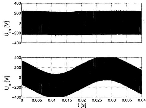
Fig. 20. Stator voltages,  $f = 30$  Hz,  $C_R = 30 \mu\text{F}$ .
