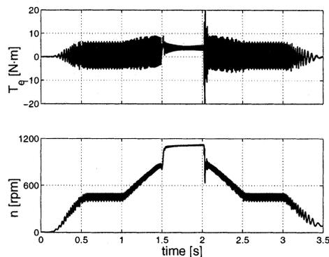
Fig. 16. Torque and speed during control of drive.
