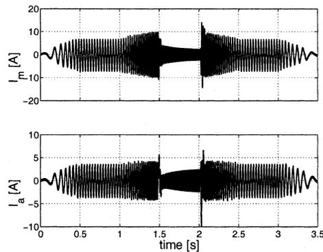
Fig. 17. Stator currents during control of drive.
