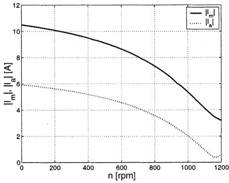
Fig. 8. Stator currents–speed characteristics, full-speed mode.
