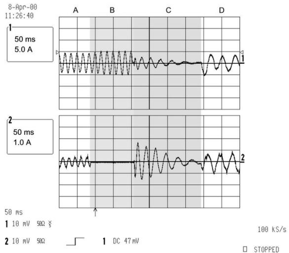
Fig. 21. Measured stator currents during transition from full- to reduced-speed operation.
