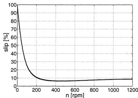
Fig. 15. Slip of machine,  $C_R = 20 \mu F$ .
