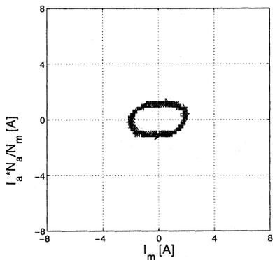
Fig. 19. Measured stator current layer,  $f = 30$  Hz,  $C_R = 30 \mu\text{F}$ .
