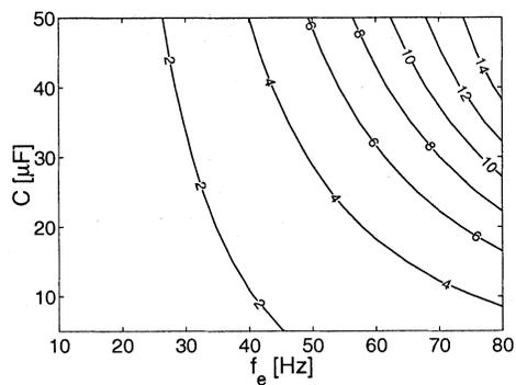
Fig. 3. Breakdown torque dependence for slip = 7.5%.
