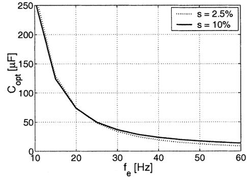
Fig. 2. Optimal run-capacitor capacitance.
