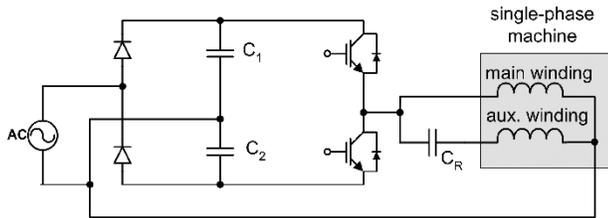
Fig. 9. Scheme of system under investigation, reduced-speed mode.
