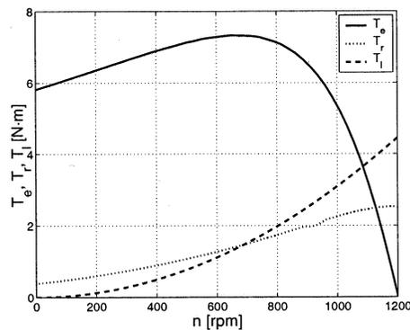
Fig. 7. Torque–speed characteristics, full-speed mode.
