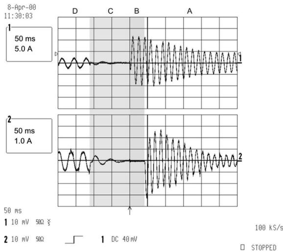
Fig. 22. Measured stator currents during transition from reduced- to full-speed operation.
