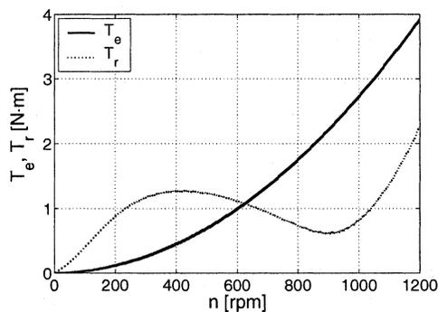
Fig. 13. Electromagnetic torque and torque-ripple amplitude,  $C_R = 20 \mu F$ .
