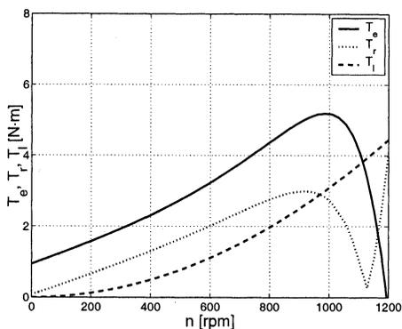
Fig. 4. Torque–speed characteristics, standard operation.
