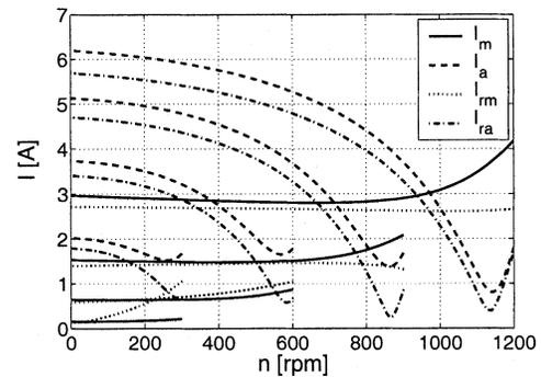
Fig. 12. Stator and rotor currents,  $C_R = 20 \mu\text{F}$ .
