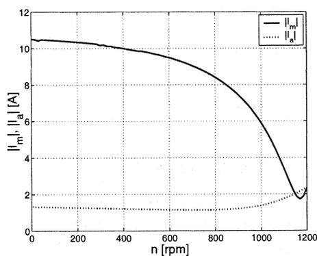
Fig. 5. Stator currents–speed characteristics, standard operation.
