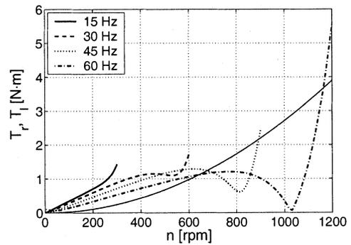
Fig. 11. Torque-ripple amplitudes,  $C_R = 20 \mu\text{F}$ .
