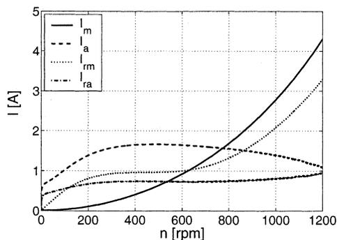
Fig. 14. Stator and rotor currents,  $C_R = 20 \mu F$ .
