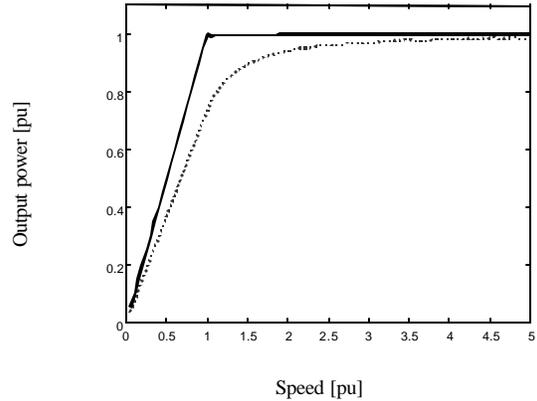
Figure 4. Power Capability curve, ideal MTA case (dotted line) and unity power factor control (solid line)
