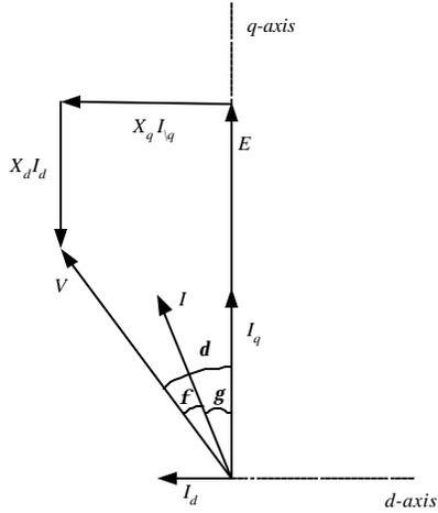
Figure 3. Phasor diagram for salient pole machine
