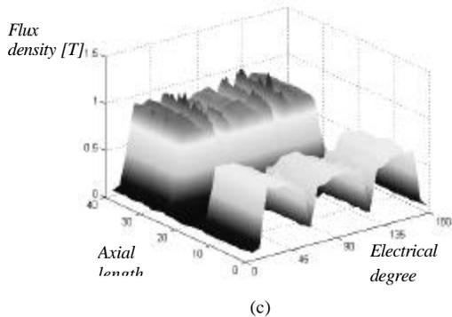
Fig. 8. Airgap flux distribution for one pole and different field AT. a) No field current, b) -500 AT, c) 500 AT
