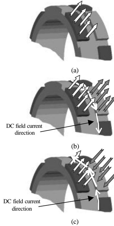
Figure 2. Airgap flux composition with field current excitation.
