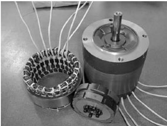
Figure 9. CPPM machine prototype
