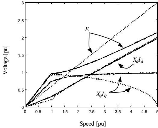
Figure.6. Open circuit voltage and reactive voltage drop for (a) MTA control ( $E_o=0.6$ pu), and (b) Unity power factor control. Machine parameters:  $X_{ds}=0.4$  pu,  $X_{qs}=1.1$  pu.
