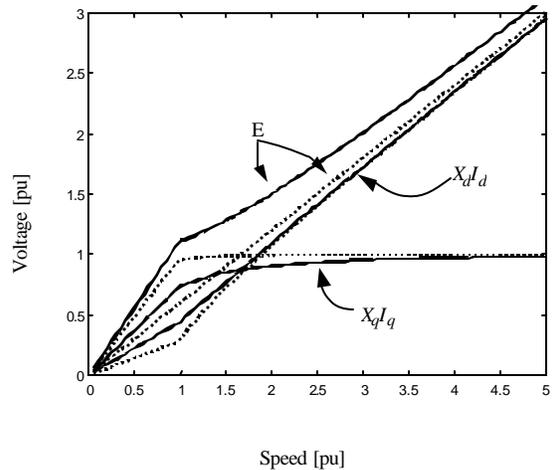
Figure 5. Control performance comparison. Solid line: unity power factor. Dotted line: MTA control ( $E_o = 0.6$  pu). Machine parameters:  $X_{ds} = 0.6$  pu,  $X_{ds} = 1.1$  pu.
