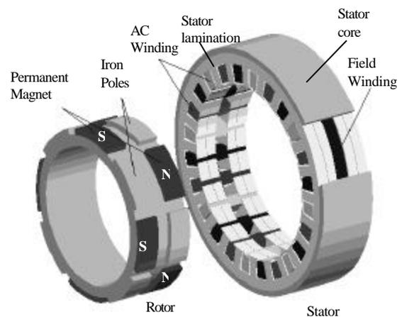
Fig. 1. 8-poles CPPM machine structure.
