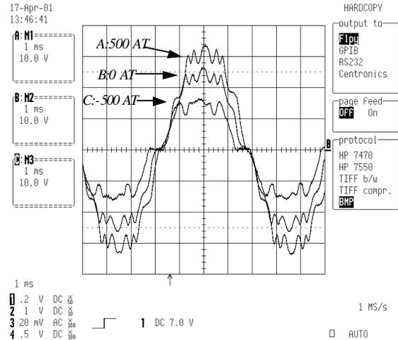
Figure 10. Oscillograph of the CPPM machine's output voltage.
