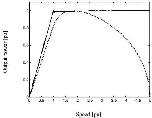
Figure. 7. Power Capability curve, non-ideal MTA case (dotted line) and unity power facto control (solid line)
