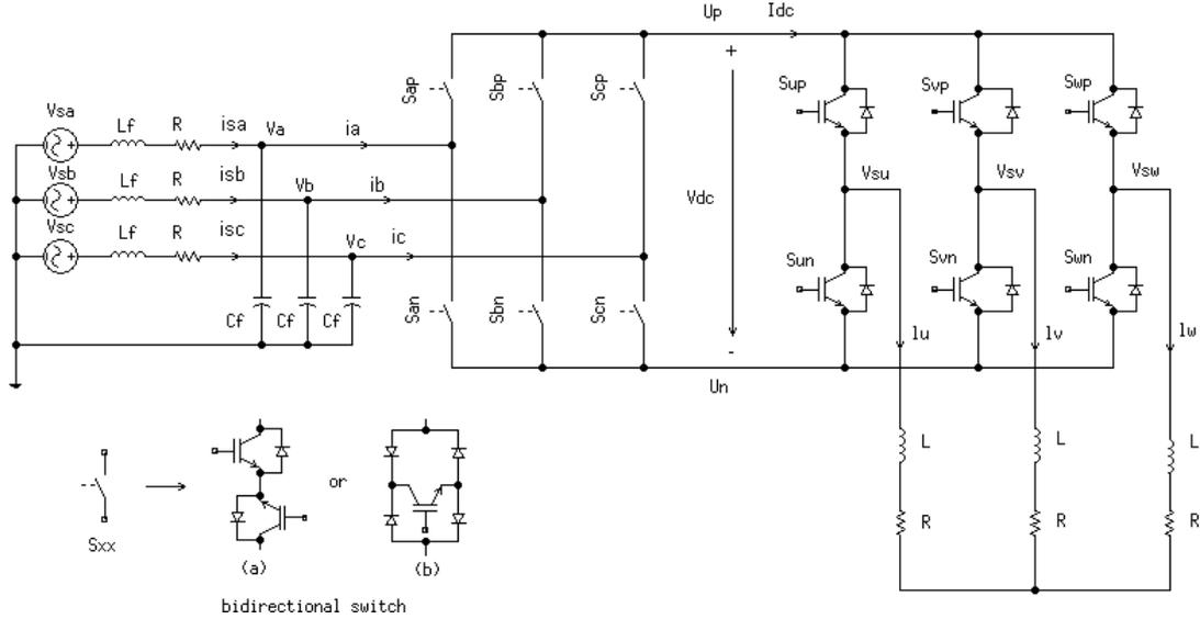
Fig. 2 Basic topology of the proposed matrix converter
