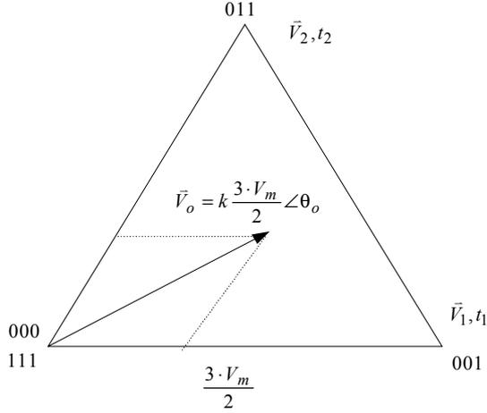
Fig. 4. Space vector PWM for inverter over the instant while  $0 < \theta_o < \pi/3$
