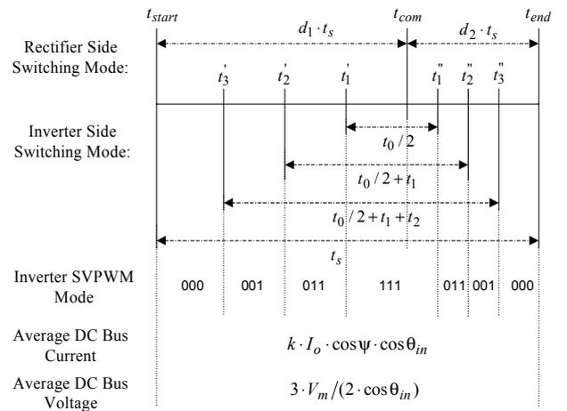
Fig. 3. PWM sequence for the proposed converter
