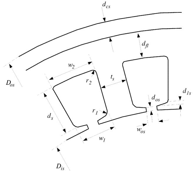
Fig. 6. Stator slot dimensions.
