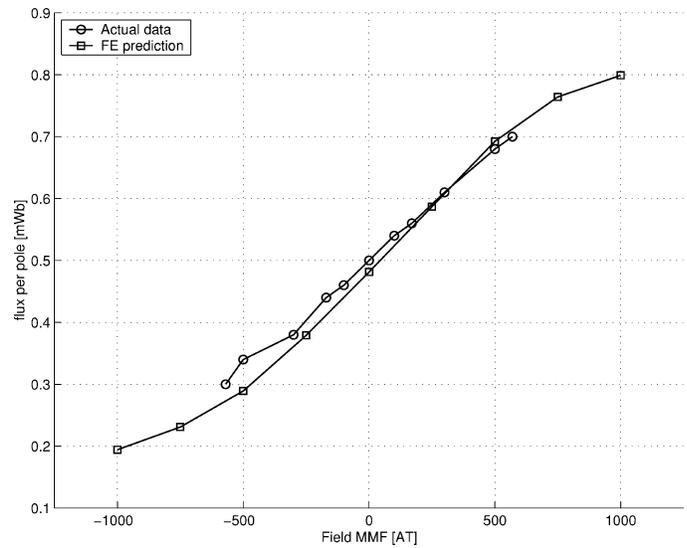
Fig. 9. FE analysis and experimental result.
