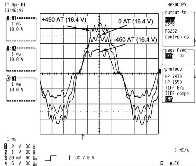
Fig. 10. Back EMF for different field ampere-turns.
