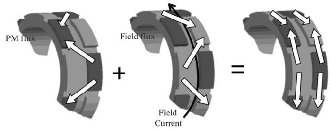
Fig. 3. Magnetizing effect of the field flux.
