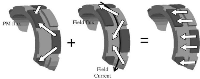
Fig. 2. Demagnetizing effect of the field flux.
