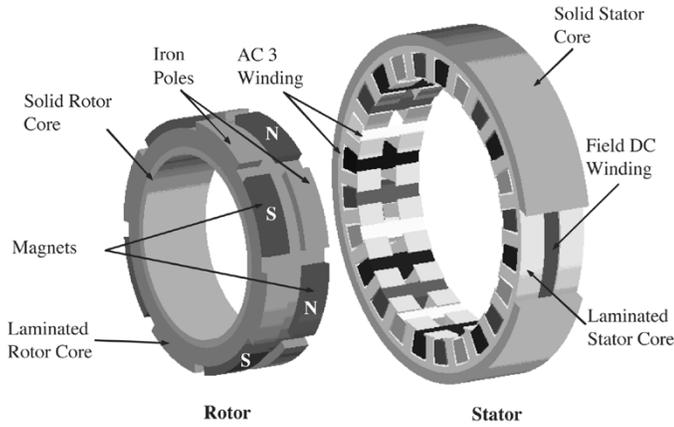
Fig. 1. Magnetic structure of the CPPM machine.
