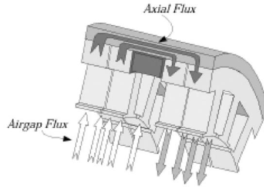
Fig. 5. Flux path in the stator yoke for the demagnetizing condition.
