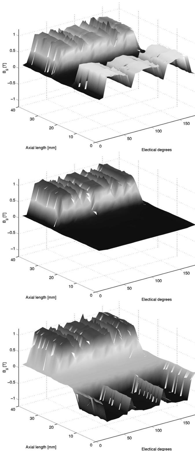
Fig. 8. Air-gap flux distribution for different field ATs. (a) 500 ATs with magnetizing effect. (b) No field current. (c) 500 ATs with demagnetizing effect.
