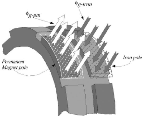
Fig. 4. Air-gap flux components.
