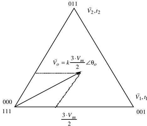
Fig. 9. Space vector PWM for inverter while  $0 < \theta_o < \pi/3$
