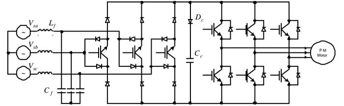
Fig. 6 The 9-switch topology with clamp circuit
