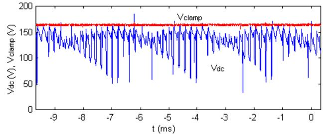
(b) DC side voltage and clamp capacitor voltage
