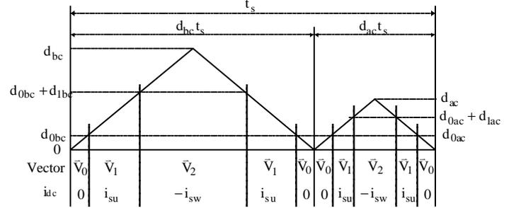
Fig. 10. PWM sequence of the converter in interval 2
