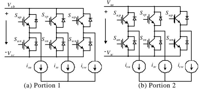
Fig. 8. Equivalent circuit in interval 2
