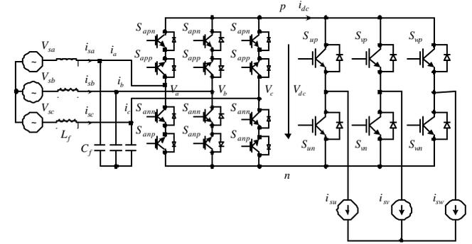
Fig. 3 Topology with 18 uni-directional voltage blocking switches
