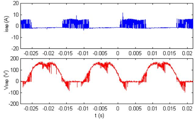
(c) Line side switch voltage / current ( $S_{ap}$ )
