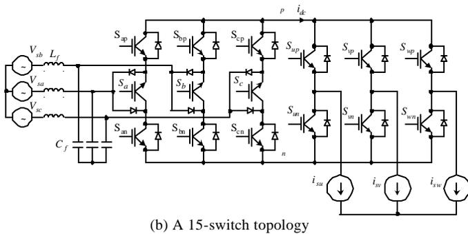
Fig. 4 Reduction of switch number from 18 to 15
