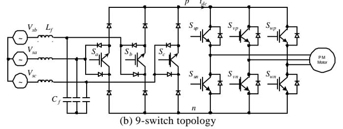
Fig. 5 Reduction of switch number to 9 or 12
