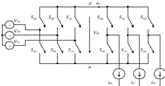
Fig. 2 Alternative matrix converter topology
