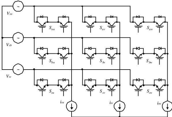
Fig. 1 Main circuit of conventional matrix converter
