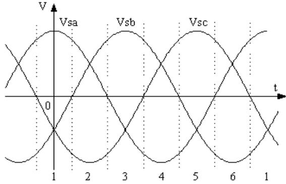
Fig. 7. Six intervals of a switching cycle
