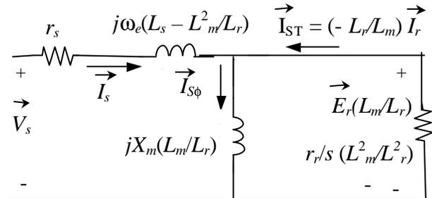
Fig. 3. Per Phase Equivalent Circuit of a Field Oriented Controlled (FOC) Induction Machine.
