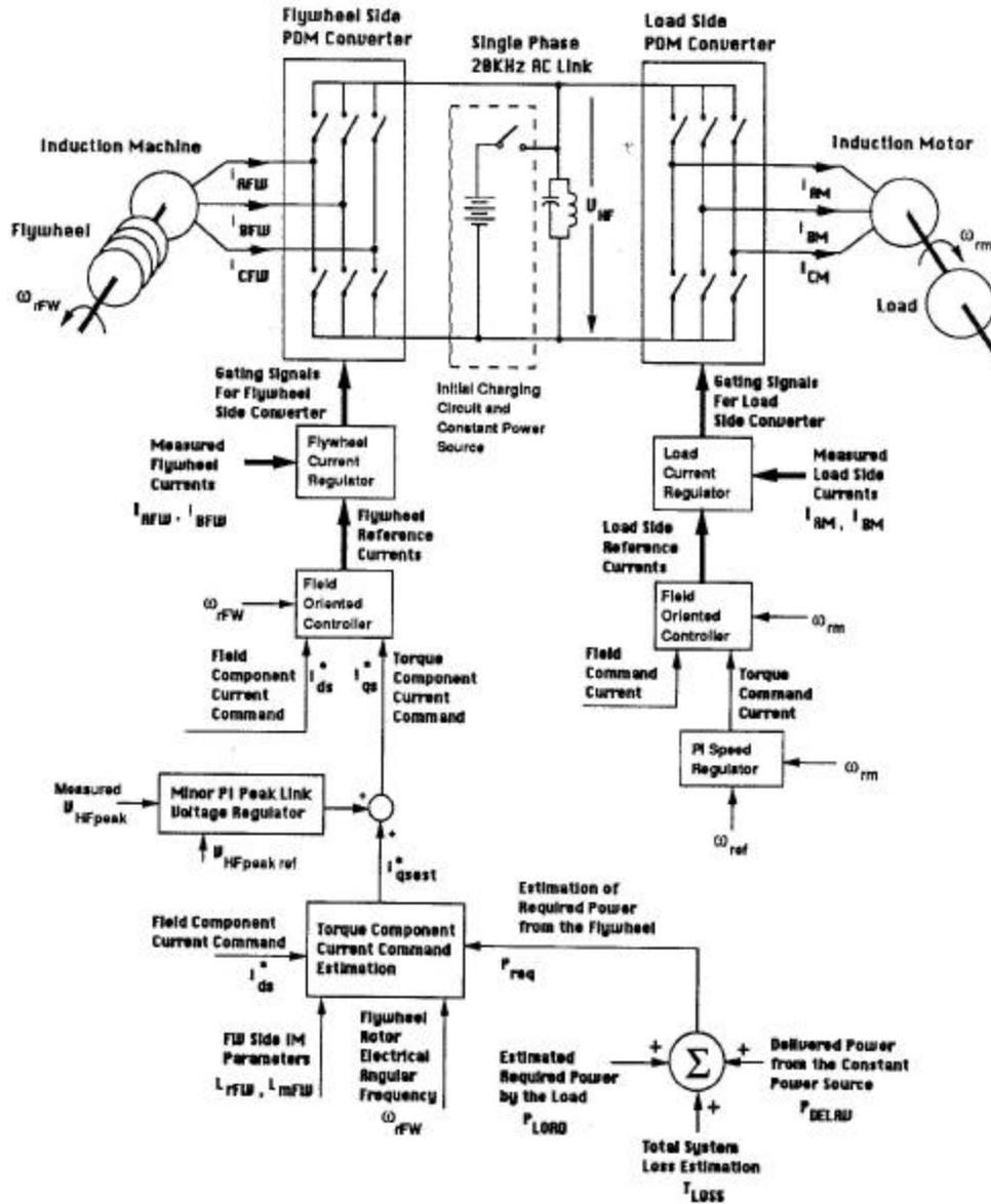
Fig. 1. Power and Control Block Diagram of the Software Simulated Flywheel Energy Storage and Load Leveling System
