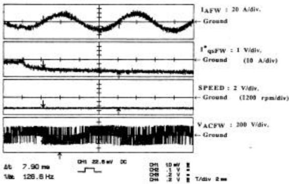
Fig. 9. Performance of Operation of the Flywheel Machine Concerning Its Electrical Quantities.  $I_{AFW}$ : Phase-A Flywheel Induction Machine Current, 20A/div.  $I_{qsfw}^*$ : Torque Component Current Command of the Flywheel Induction Machine, 10A/div. **Speed**: Speed of the Flywheel, 1200 rpm/div.  $V_{ACFW}$ : Phase-AC Line to Line Voltage of the Flywheel, 200V/div. Time/div: 1 ms.
