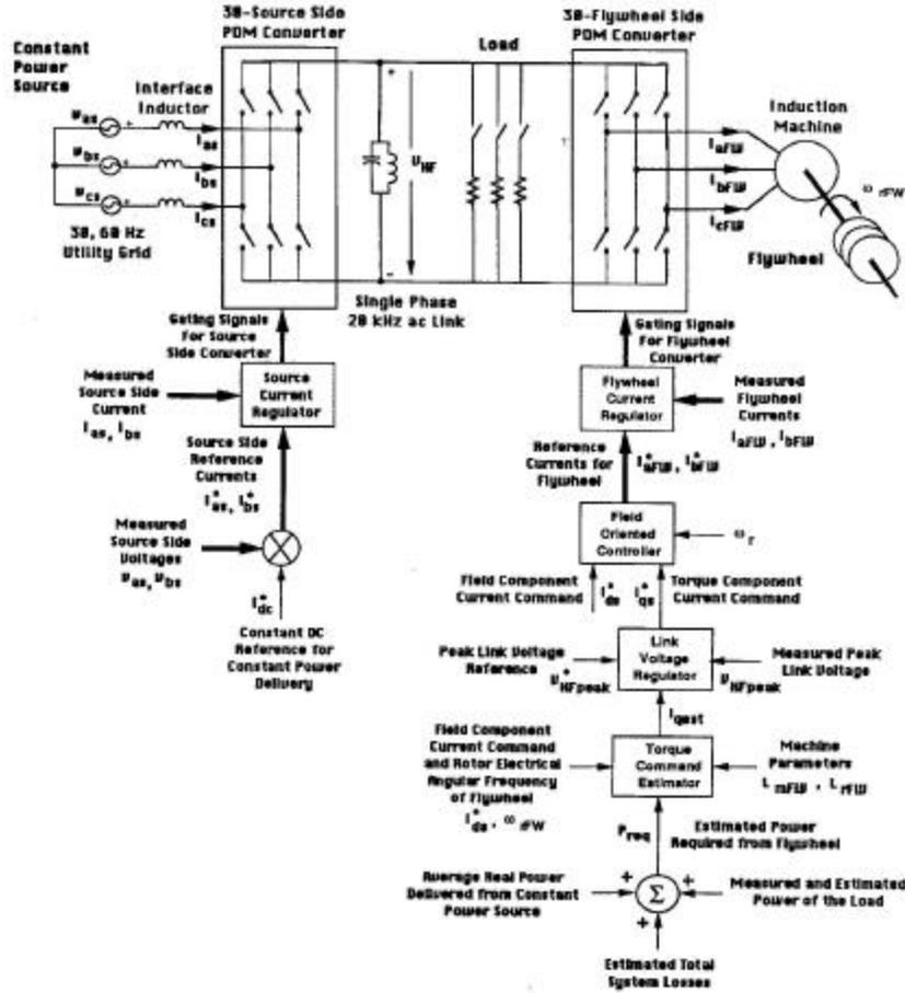
Fig. 7. Power and Control Block Diagram of the Hardware Prototype Flywheel Energy Storage and Load Leveling System
