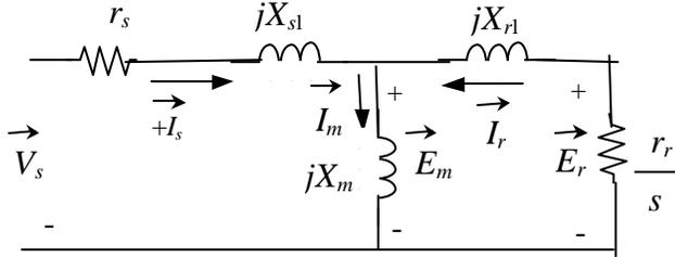
Fig. 2. Classical Per Phase Equivalent Circuit of an Induction Machine.
