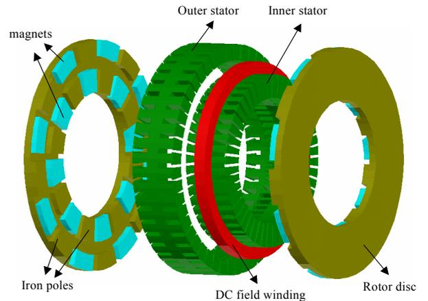
Fig. 3. 3D view of the new axial flux surface mounted field controlled TORUS (FCT) machine
