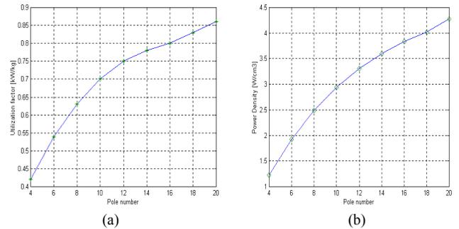
Fig. 10. Machine utilization and power density for different pole numbers
