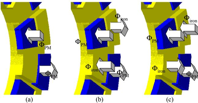
Fig. 6. Airgap flux directions of the FCT machine (a) with no (b) with positive and (c) with negative field currents
