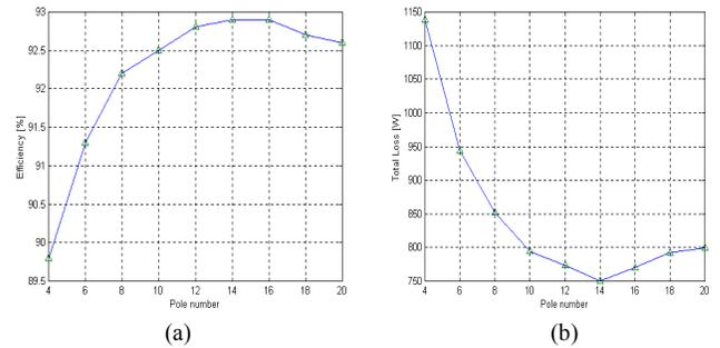
Fig. 9. Machine efficiency and total loss for different pole numbers
