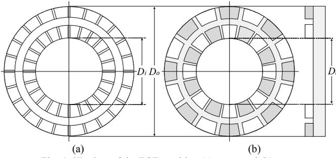
Fig. 4. 2D view of the FCT machine (a) stator and (b) rotor
