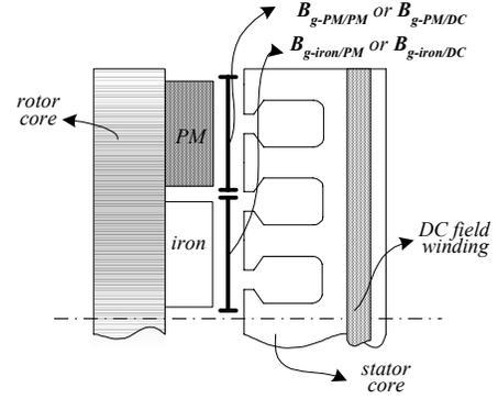
Fig. 8. 2D Illustration of the airgap flux density components of the FCT machine
