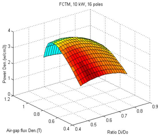
Fig. 11. Power density plot as a function of airgap flux density and diameter ratio (without field winding)
