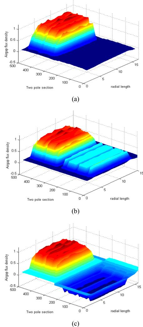
Fig. 17. Airgap flux density distribution of the FCT machine for different values of the DC field current over one pole at (a) 0 Atorns, (b) +1200 Atorns, (c) -1200 Atorns current cases
