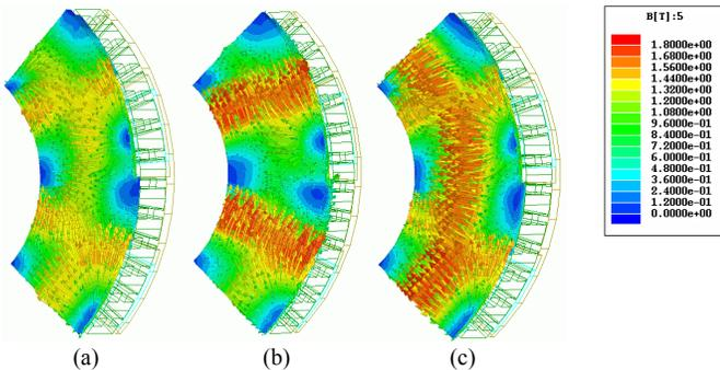
Fig. 16. Rotor flux density distribution and directions for different values of the DC field current: (a) 0 Atorns, (b) -1200 Atorns, (c) +1200 Atorns current cases
