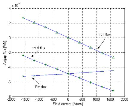
Fig. 18. Airgap flux (PM flux, iron flux and total flux) of the FCT machine over one pole
