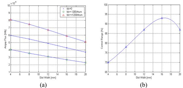
Fig. 13. Total airgap flux of the FCT machine for different field currents (a) and control range (b) for varying slot width at no load
