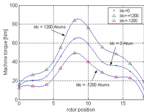
Fig. 19. Static torque characteristic of the FCT machine for different field current values
