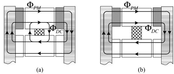
Fig. 12. PM and DC field flux paths of the FCT machine with (a) small slot width and (b) large slot width
