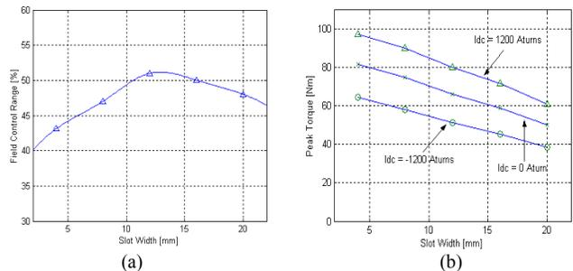
Fig. 14. Field control range at full load (a) and machine peak torque (b) for different slot width of the DC field winding
