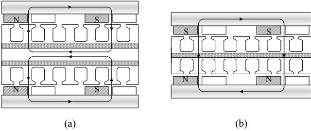
Fig. 2. Structures and 2D main flux directions of the NN type FCT (a) and NS type FCT (b) machines at the average diameter over two poles
