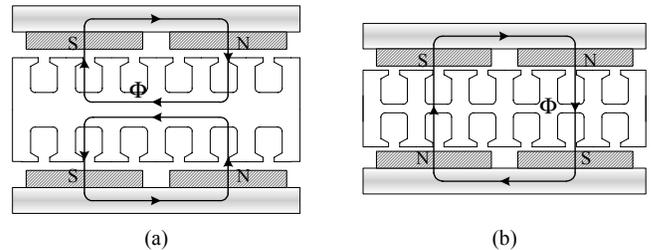
Fig. 1. Structures and 2D flux directions of the NN type TORUS (a) and NS type TORUS (b) machines at the average diameter over two poles
