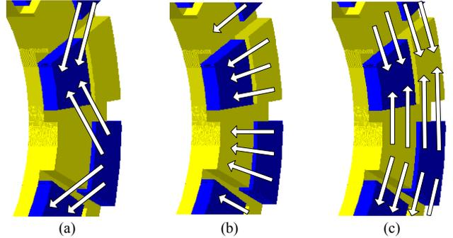
Fig. 7. Flux distribution of the FCT machine (a) with no (b) with positive and (c) with negative field currents
