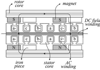
Fig. 5. Main flux directions of the 2 pole portion of FCT machine at the average diameter
