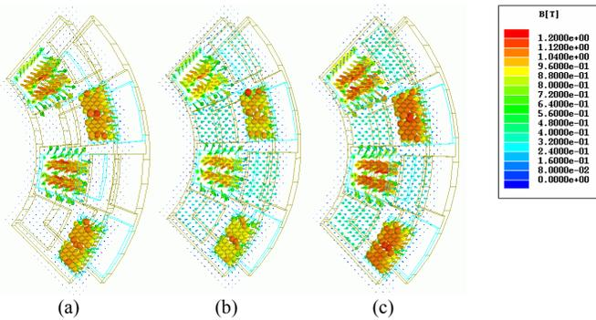
Fig. 15. Stator and rotor flux density distribution and directions for different values of the DC field current
