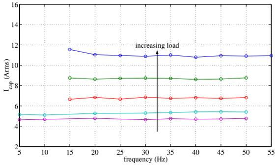
Figure 11. Calculated RMS capacitor current with varying  $V_{dc}$  and constant modulation index  $M_i = 1.07$ .
