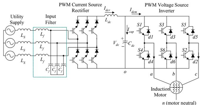
Figure 1. PAM/PWM converter with Current Source Rectifier and Voltage Source Inverter.
