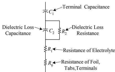
Figure 2. Electrolytic Capacitor Model.
