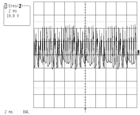
Figure 8. Experimental capacitor ripple current waveform:  $V_{dc} = 228V$ , 40Hz fundamental, 75% rated motor torque load, 3bit enhanced res.
