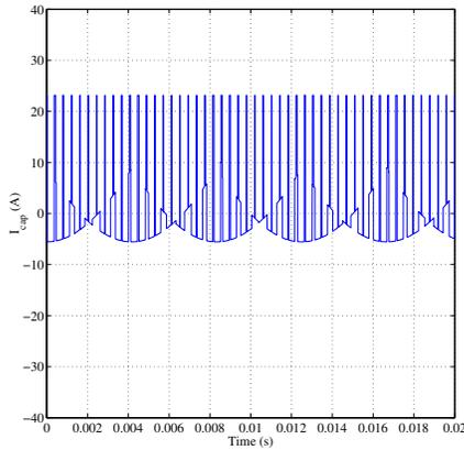
Figure 7. Calculated capacitor ripple current waveform:  $V_{dc} = 228V$ , 40Hz fundamental, 75% rated motor torque load.
