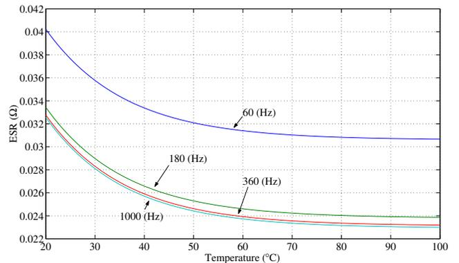
Figure 4. ESR vs. Temperature of electrolytic capacitor bank for several frequencies of interest.
