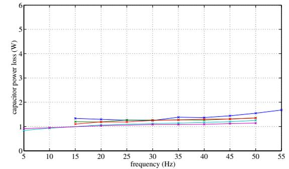
Figure 16. Experimental capacitor power loss with varying  $V_{dc}$  and constant modulation index  $M_i = 1.07$ .
