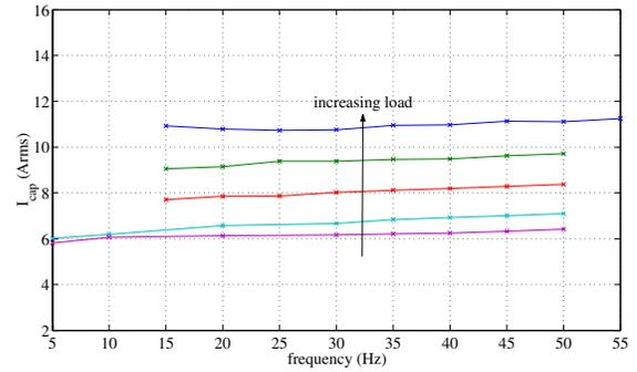
Figure 12. Experimental RMS capacitor ripple current with varying  $V_{dc}$  and constant modulation index  $M_i = 1.07$ .
