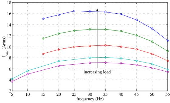
Figure 9. Calculated RMS electrolytic capacitor current with constant  $V_{dc} = 323V$  and varying modulation index.
