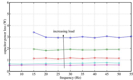
Figure 15. Calculated capacitor power loss with varying  $V_{dc}$  and constant modulation index  $M_i = 1.07$ .
