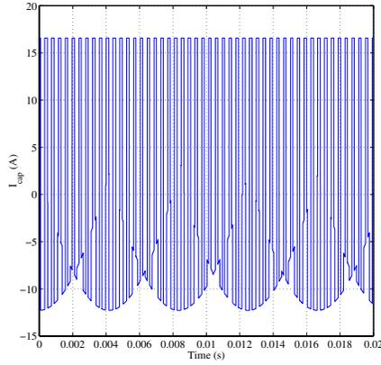
Figure 5. Calculated capacitor ripple current waveform: full  $V_{dc}$ , 40Hz fundamental, 75% rated motor torque load.
