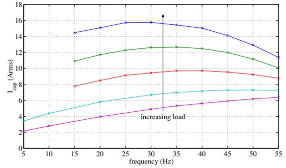
Figure 10. Experimental RMS capacitor ripple current with constant  $V_{dc} = 323V$  and varying modulation index.
