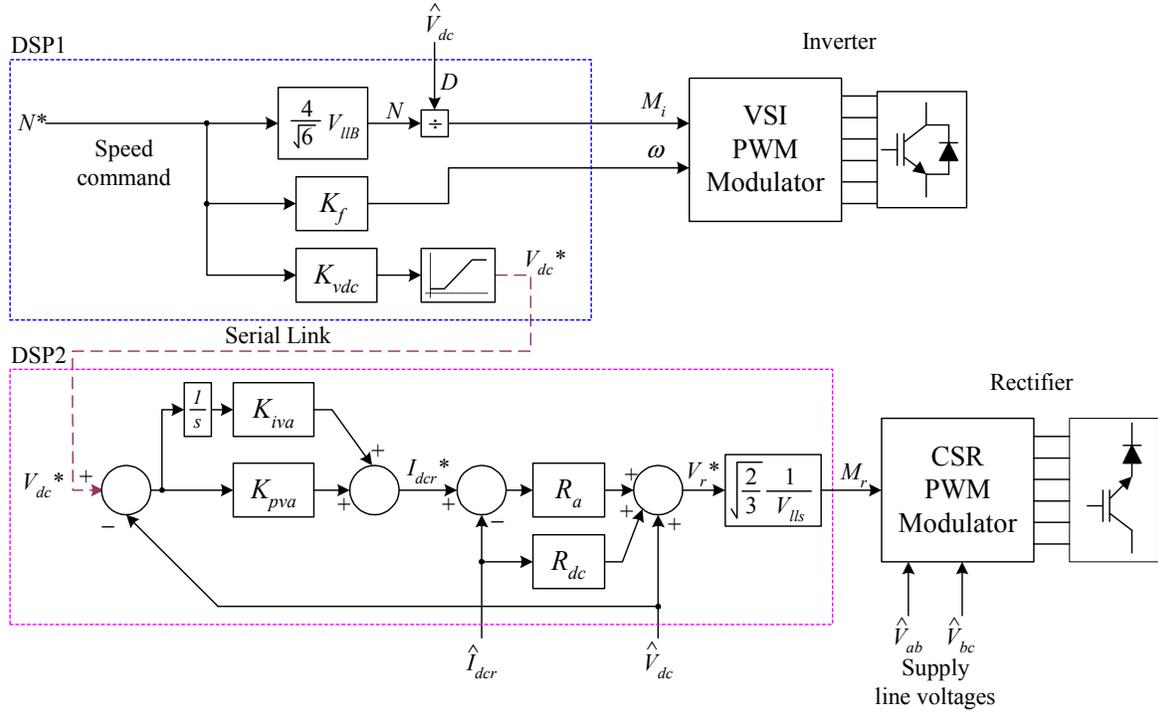
Figure 17. Proposed two DSP controller for PAM/PWM motor drive: VSI with  $V_{dc}$  compensation of modulation index for open loop V/f control and  $V_{dc}^*$  generation, CSR with closed loop PI voltage regulator.
