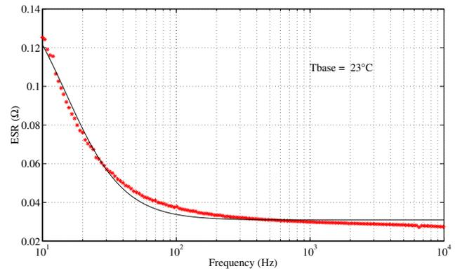
Figure 3. ESR vs. frequency of electrolytic capacitor bank: experimental data points (\*), model with curve fit parameters (—).
