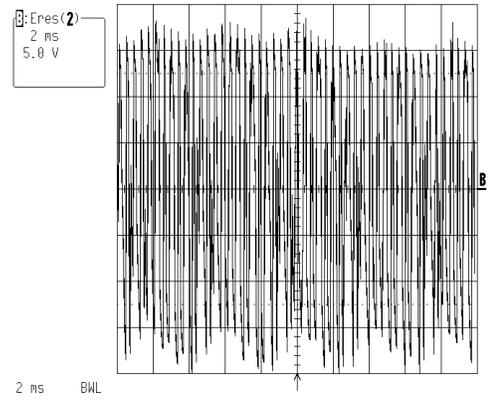
Figure 6. Experimental capacitor ripple current waveform: full  $V_{dc}$ , 40Hz fundamental, 75% rated motor torque load, 3bit enhanced res.
