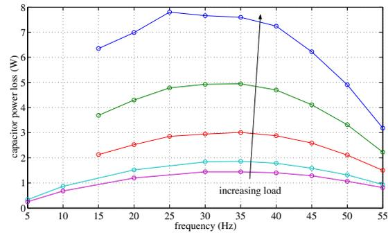
Figure 13. Calculated capacitor power loss with constant  $V_{dc} = 323V$  and varying modulation index.
