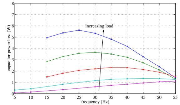
Figure 14. Experimental capacitor power loss with constant  $V_{dc} = 323V$  and varying modulation index.
