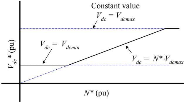
Figure 18. Per unit DC bus voltage command ( $V_{dc}^*$ ) vs. Speed ( $N^*$ ) generated in VSI controller and sent serially to CSR controller.
