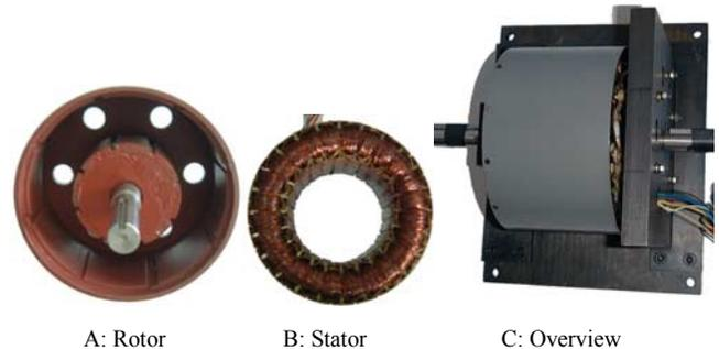
Figure 12. Prototype machine
