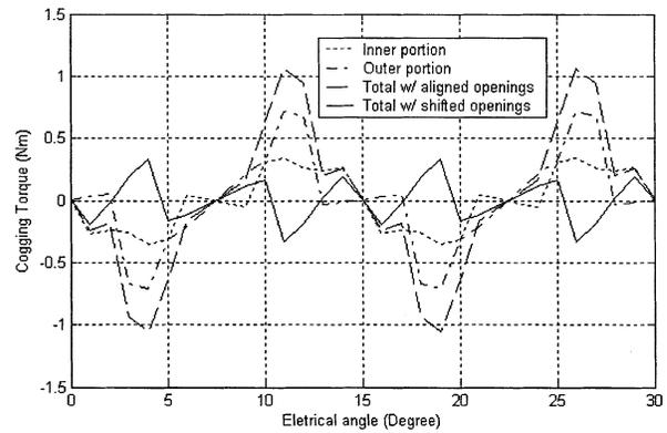
Fig. 6. Cogging torques achieved by different-type slot openings.
