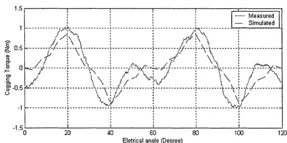
Fig. 14. Cogging torque of the prototype.
