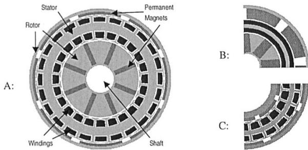
Fig. 2. Other dual-rotor RFTPM machine topologies. A: hybrid-PM with slots; B: hybrid-PM without slots; C: surface-PM with slots.
