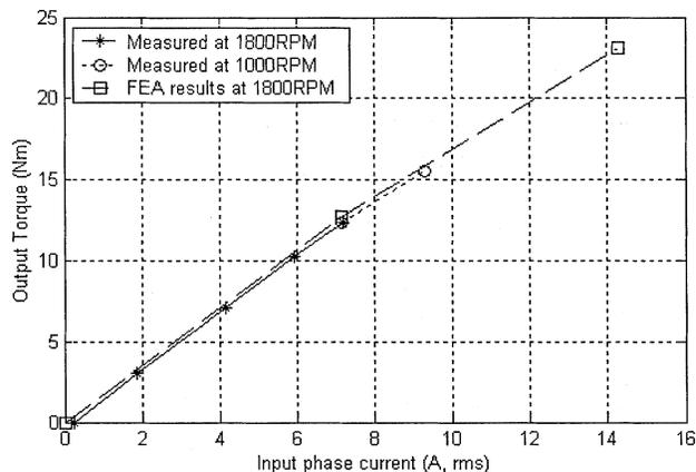
Fig. 15. Output torque versus input phase current.
