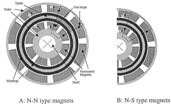
Fig. 1. Structure and flux distributions of dual-rotor, radial-flux, nonslotted, PM machine with surface-mounted magnets.
