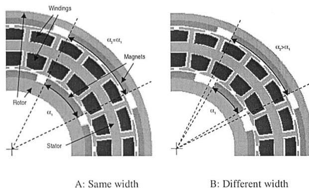
Fig. 9. Varying PM angular width for the inner and outer magnets.
