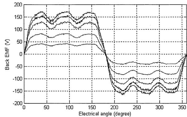
Fig. 13. Open-circuit back-EMF waveforms of Phase A at 500, 1000, 1500, 1800, and 2000 r/min.
