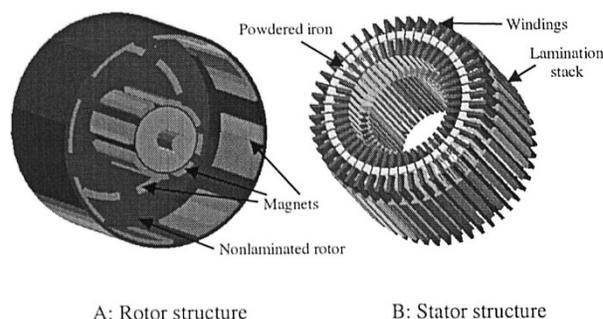
Fig. 4. Structure of an enhanced dual-rotor, slotted, RFTPM machine.
