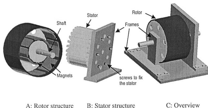
Fig. 3. Mechanical structure.
