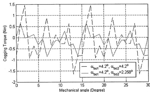
Fig. 8. Comparison of the cogging torques for the different slot-opening angular widths ( $\alpha_1 = \alpha_2 = 40^\circ$ ).
