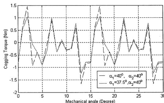
Fig. 10. Comparison of the cogging torques for the different PM angular widths ( $\alpha_{bo1} = \alpha_{bo2} = 4.2^\circ$ ).
