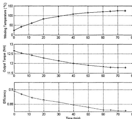
Fig. 16. Temperature effect on torque and efficiency.
