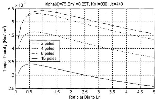
Fig. 11. Effect of the ratio of stator inner diameter  $D_{is}$  to machine effective length  $L_r$  on torque density.
