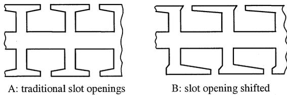
Fig. 5. Linear translational stator laminations with the different slot opening designs.
