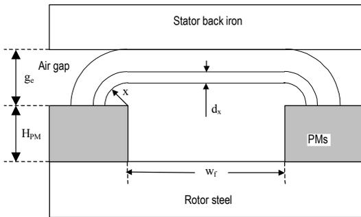
Figure 6. A circular-arc, straight-line permeance model of magnet-to-magnet leakage flux
