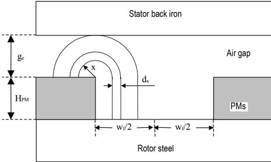
Figure 5. A circular-arc, straight-line permeance model of magnet-to-rotor leakage flux
