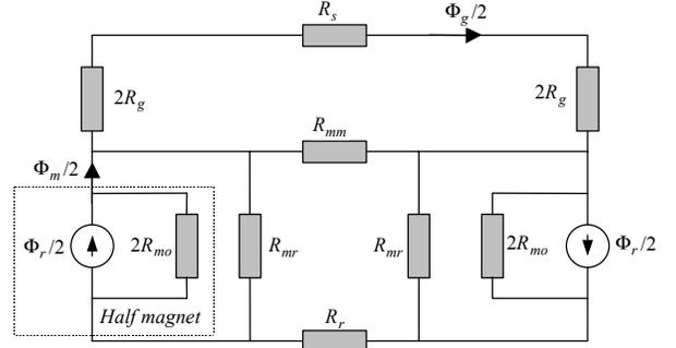
Figure 2. Equivalent magnetic lumped circuit for Fig. 1
