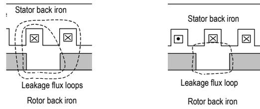
(b) leakage flux linking a part of one phase winding
