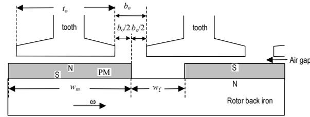
(a) no zigzag leakage at  $x=0$
