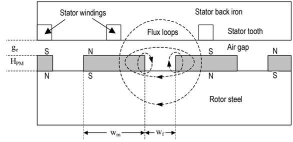
Figure 1. Simple linear translational motor topology
