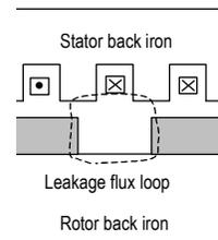
(c) leakage flux going through tooth to tooth
