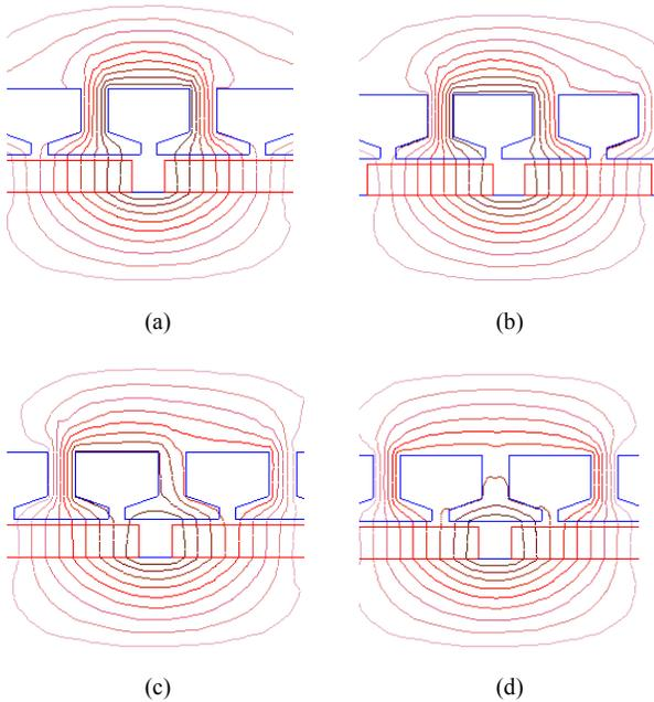
Figure10. Zigzag leakage fluxes short-circuited by a tooth
