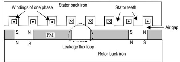
(a) leakage flux short-circuited by one tooth
