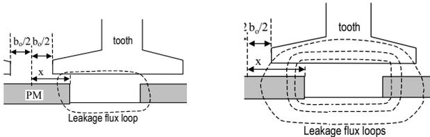
(b) Increasing leakage flux as  $x$  increases to  $(t_o + b_o - w_f)/2$  from 0
