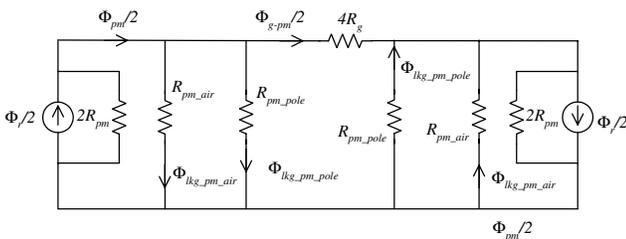
Fig. 5. Reluctance based equivalent circuit for the PM flux
