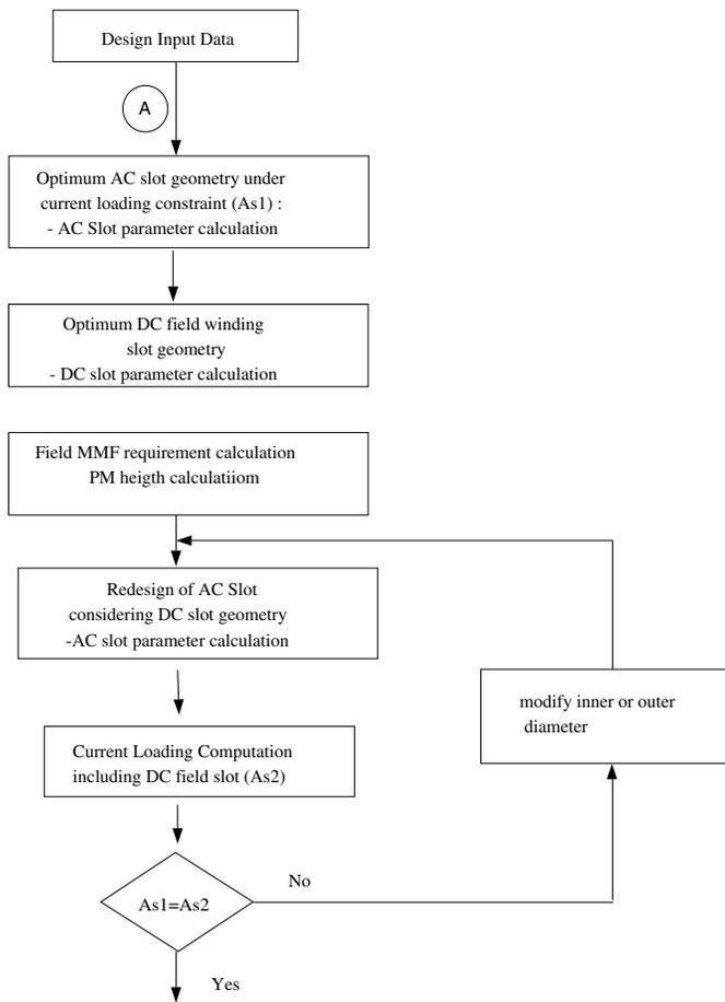
Fig. 11. Design flow diagram for the CPPM machine
