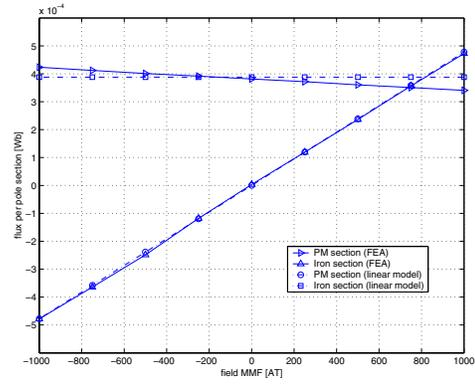
Fig. 6. Comparison with the linear model: eqs. 5 and 6 with 3D-FEA
