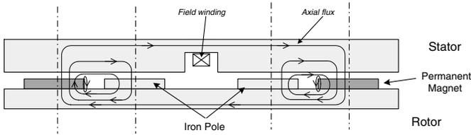
Fig. 2. 2-pole extended magnetic circuit of the CPPM machine
