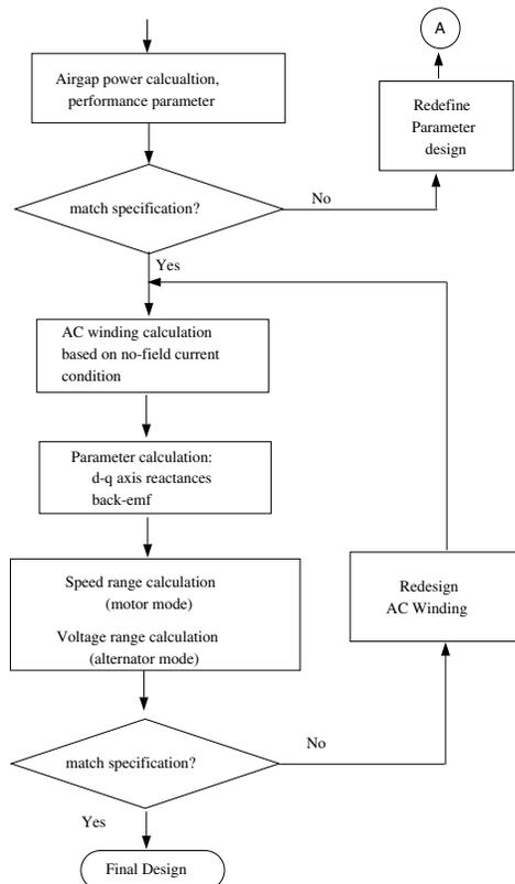
Fig. 12. Design flow diagram for the CPPM machine (continuation)
