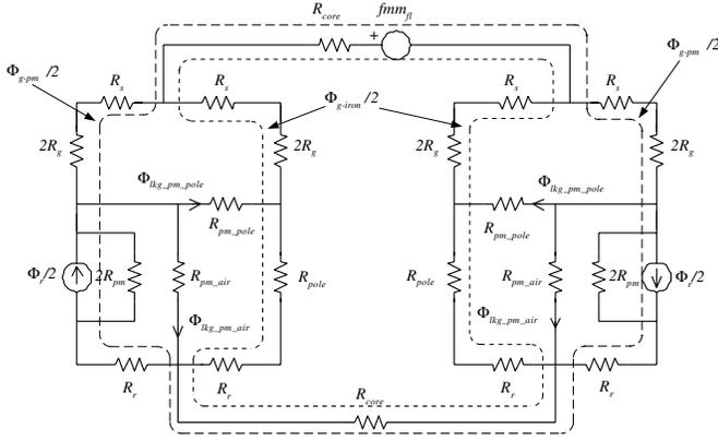
Fig. 3. Reluctance based equivalent circuit of figure 2.
