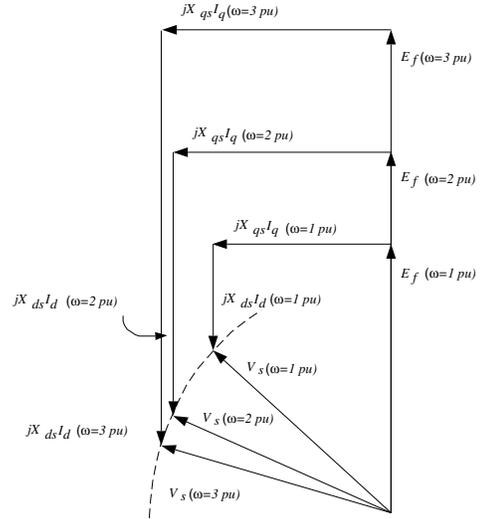
Fig. 8. Phasor diagram for constant power mode
