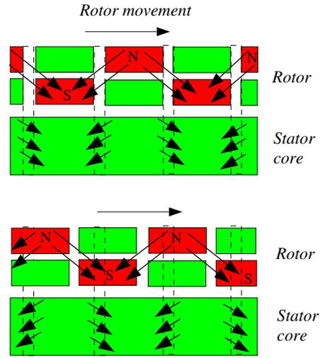
Fig. 7. Spatial flux variation in the stator core due to the rotor movement
