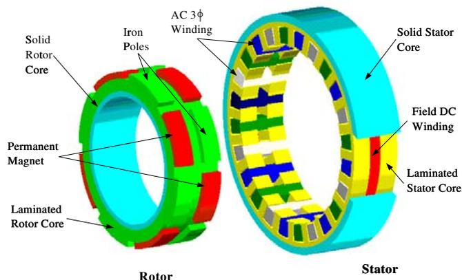
Fig. 1. Structure of the CPPM machine
