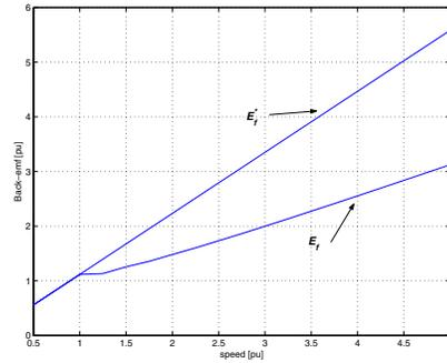
Fig. 9. Back-emf requirement to maintain unity terminals voltage as speed increases
