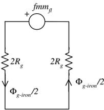
Fig. 4. Equivalent circuit for the field flux
