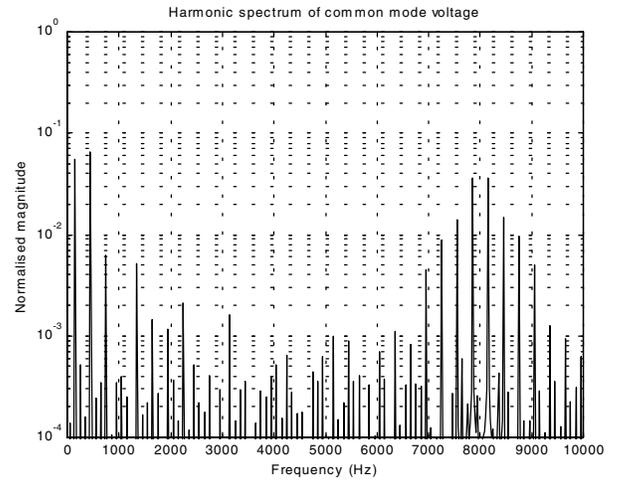
Figure 13: Simulated spectrum of common mode voltage using phase-shifted PCME-APOD – normalised to line fundamental voltage magnitude.
