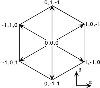
Figure 4: Reduced space vector diagram of a three-level inverter.
