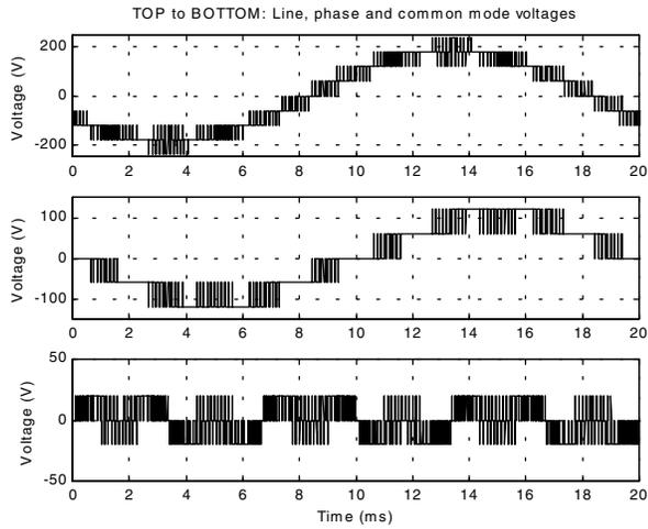
Figure 12: Simulated waveforms using phase-shifted PCME-APOD – (1) line voltage, (2) phase-leg voltage, (3) common mode voltage.
