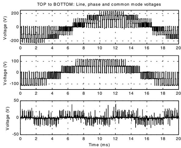
Figure 14: Experimental waveforms using phase-shifted CCME-APOD – (1) line voltage, (2) phase leg voltage, (3) common mode voltage.
