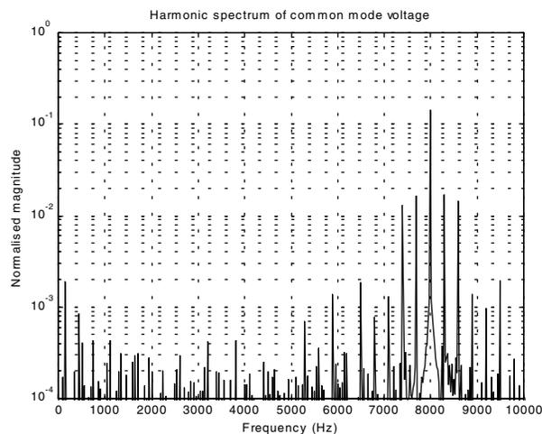
Figure 11: Simulated spectrum of common mode voltage using conventional discontinuous PD – normalised to line fundamental voltage magnitude.
