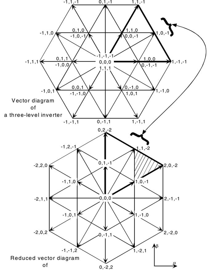
Figure 5: Linkage between vector diagrams of three-level and reduced common mode five-level inverters.
