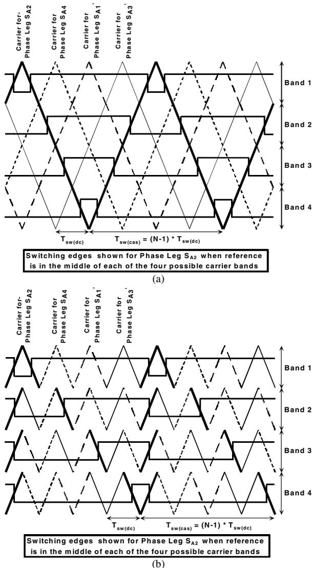
Figure 7: Derivation of cascaded inverter PWM from NPC carrier disposition PWM (a) APOD strategy (b) PD strategy.
