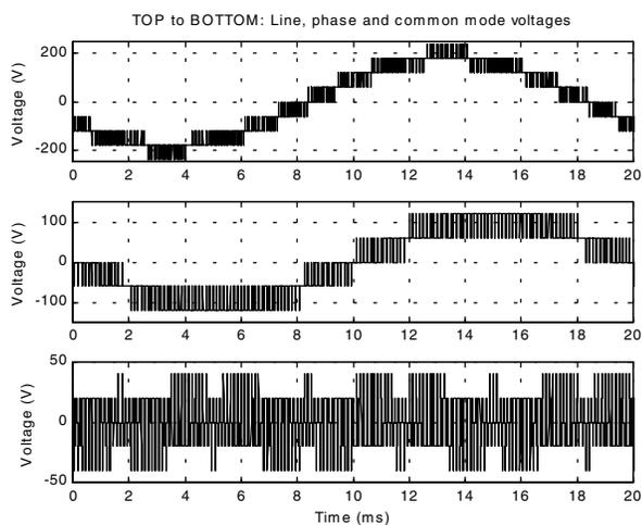
Figure 10: Simulated waveforms using conventional discontinuous PD – (1) line voltage, (2) phase-leg voltage, (3) common mode voltage.
