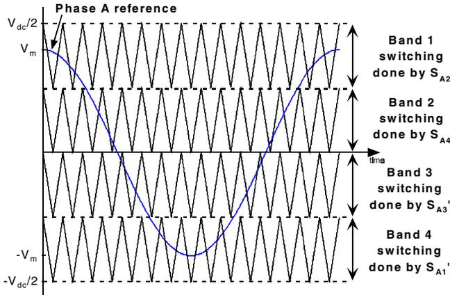
Figure 8: Derivation of discontinuous PD strategy: switching band allocation for each H-bridge phase-leg.
