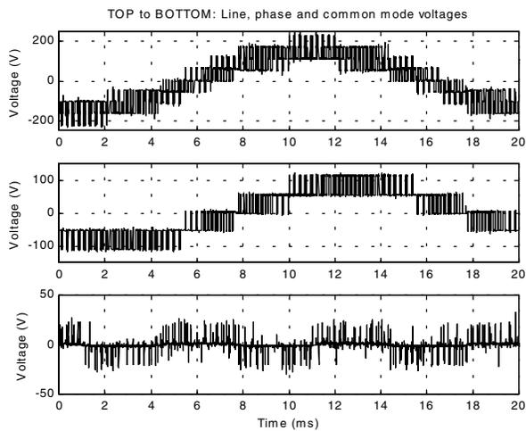
Figure 16: Experimental waveforms using discontinuous CCME-PD – (1) line voltage, (2) phase leg voltage, (3) common mode voltage.
