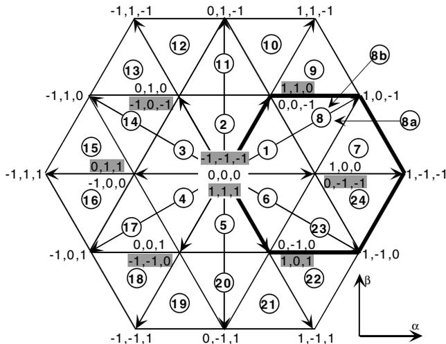
Figure 2: Space vector diagram of a three-level inverter (state indexes normalised with  $V_{dc}$ ).
