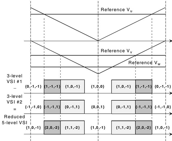
Figure 6: Generation of reduced common mode five-level switching states.
