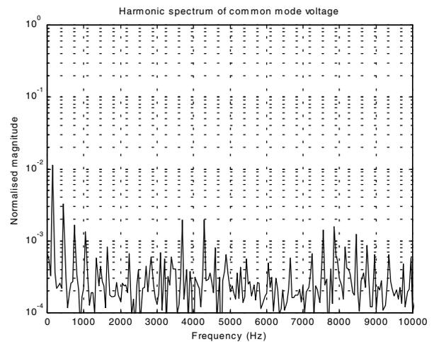
Figure 17: Experimental spectrum of common mode voltage using discontinuous CCME-PD – normalised to line fundamental voltage magnitude.
