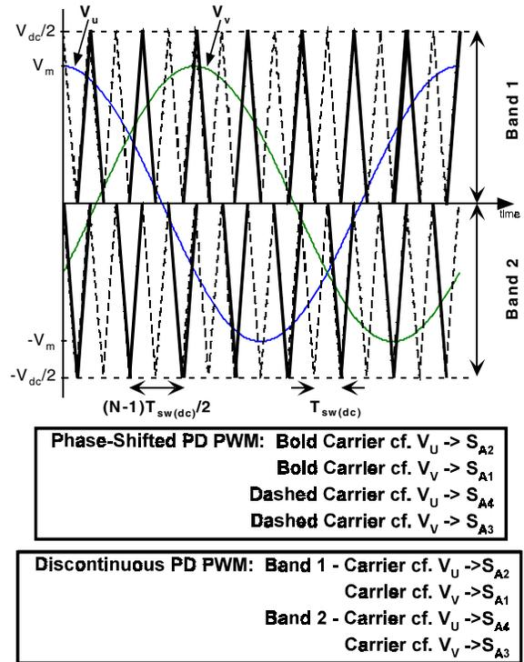
Figure 9: Derivation of carrier placements for phase-shifted and discontinuous CCME-PD for cascaded five-level inverter.
