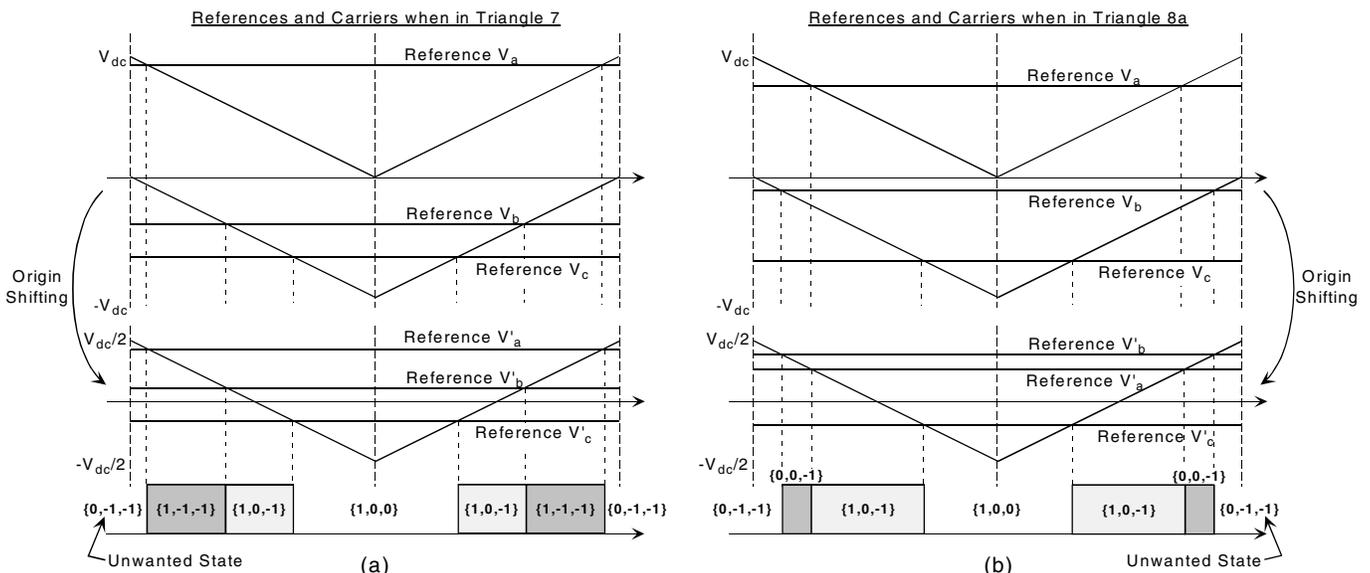
Figure 3: Typical vector sequences when reference phasor is in (a) triangle 7 and (b) triangle 8a.
