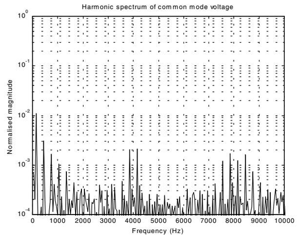
Figure 15: Experimental spectrum of common mode voltage using phase-shifted CCME-APOD – normalised to line fundamental voltage magnitude.
