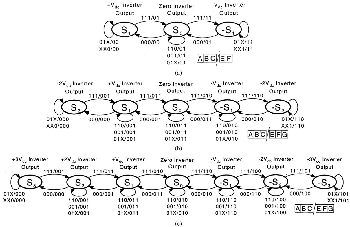
Fig. 5. State machine transitions for (a) a three-level system, (b) a five-level system, and (c) a seven-level system. A, B, and C represent the comparator outputs while E, F, and G represent the logic state bits.
