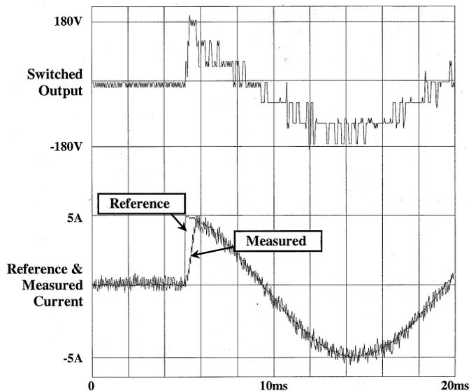
Fig. 21. Experimental transient performance with outer hysteresis band (hybrid inverter).
