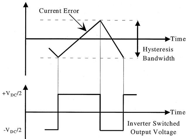
Fig. 1. Conventional two-level hysteresis current regulation.
