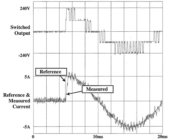
Fig. 19. Experimental transient performance with outer hysteresis band (five-level inverter).
