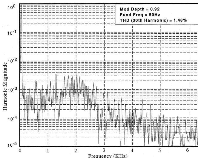
Fig. 15. Experimental load current harmonic spectrum (hybrid inverter).
