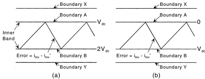
Fig. 7. Current error trajectory within the inner hysteresis band. (a) Switching between  $V_{DC}$  and  $2V_{DC}$ . (b) Switching between 0 and  $V_{DC}$ .
