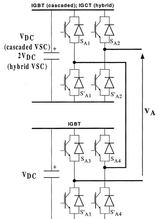
Fig. 6. Single-phase hybrid inverter.
