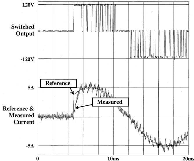
Fig. 17. Experimental transient performance with outer hysteresis band (three-level inverter).
