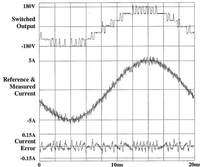
Fig. 14. Experimental steady-state performance (hybrid inverter).
