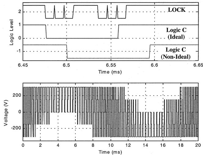
Fig. 8. System performance using a lockout time of  $10 \mu s$  (five-level inverter). Top: lockout logic LOCK, Logic C without delays (ideal), Logic C with delays (nonideal); bottom: output voltage.
