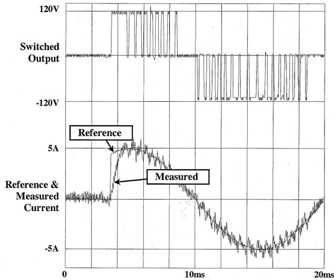
Fig. 16. Experimental transient performance without outer hysteresis band (three-level inverter).
