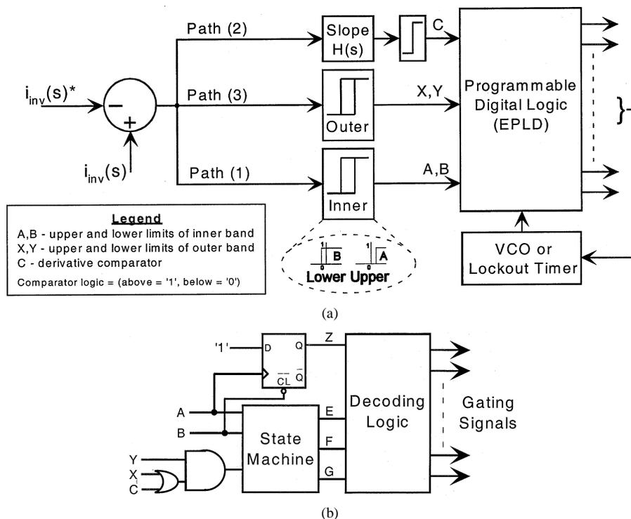
Fig. 4. Time-based hysteresis current regulator. (a) General layout. (b) Digital logic.
