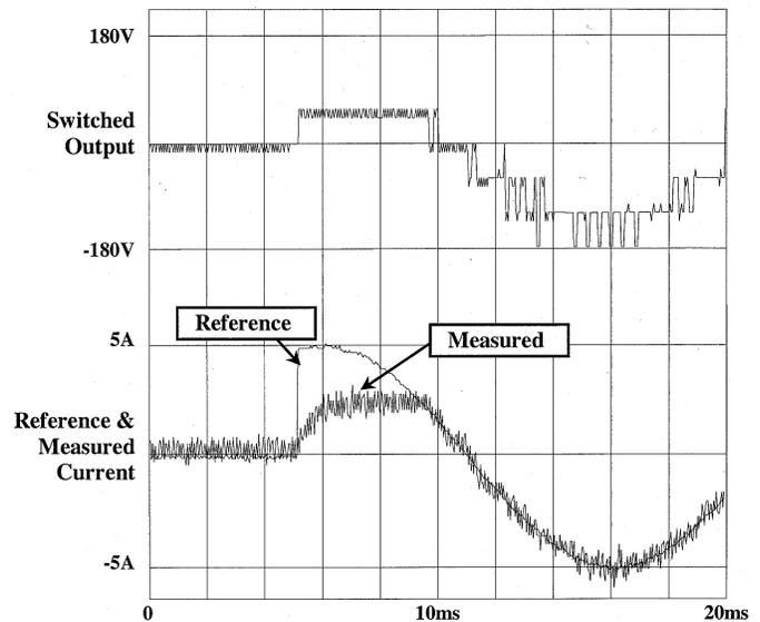
Fig. 20. Experimental transient performance without outer hysteresis band (hybrid inverter).
