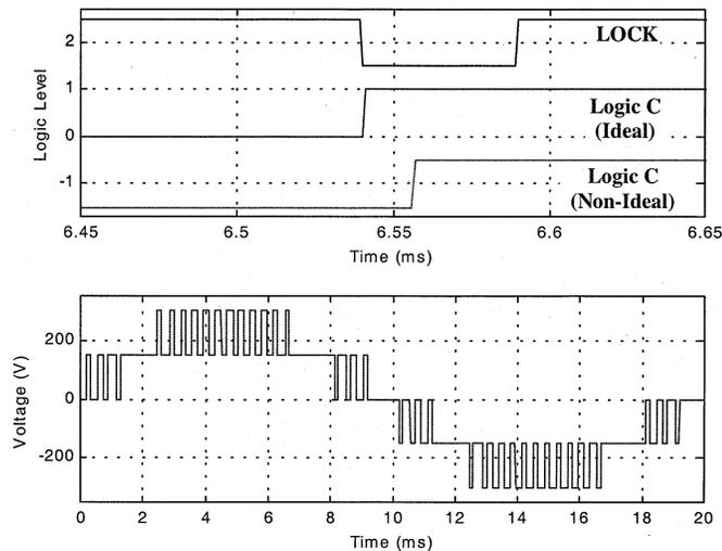
Fig. 9. System performance using a lockout time of  $50 \mu s$  (five-level inverter). Top: lockout logic LOCK, Logic C without delays (ideal), Logic C with delays (nonideal); bottom: output voltage.
