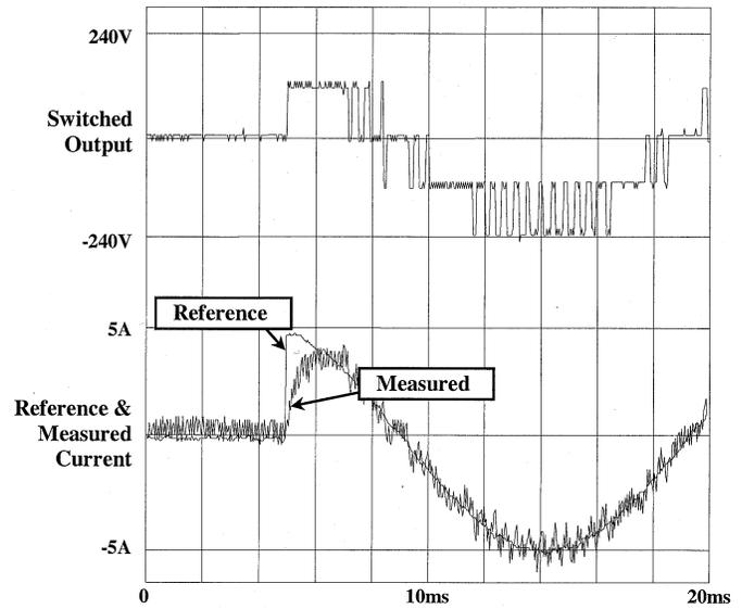
Fig. 18. Experimental transient performance without outer hysteresis band (five-level inverter).
