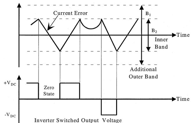
Fig. 3. Time-based multilevel hysteresis current regulation.
