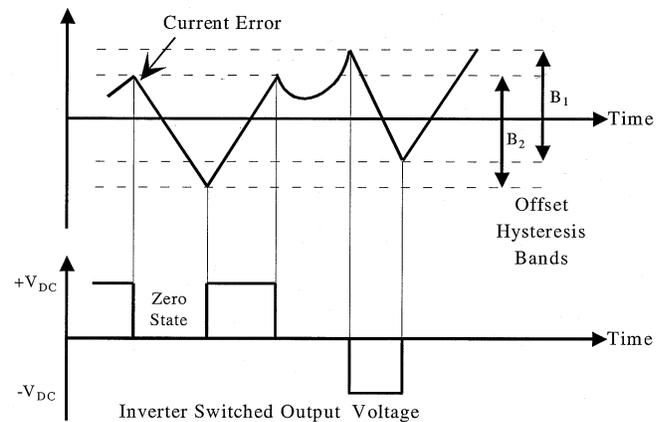
Fig. 2. Multiband multilevel hysteresis current regulation.
