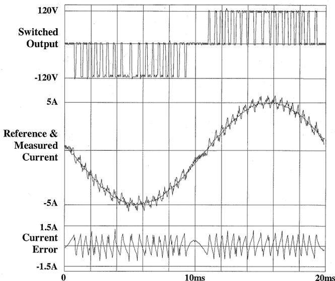
Fig. 12. Experimental steady-state performance (three-level inverter).
