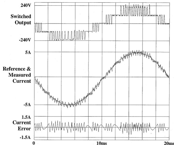
Fig. 13. Experimental steady-state performance (five-level inverter).
