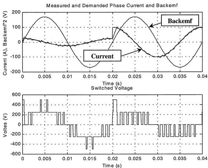
Fig. 11. Simulated transient performance for the case of demanded current in quadrature with the back-EMF (five-level inverter).
