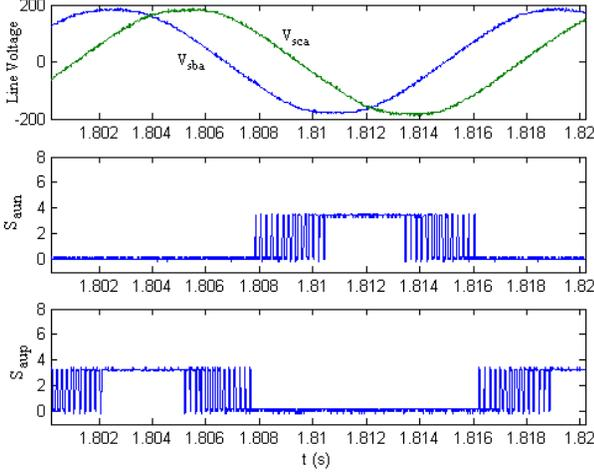
Fig. 6. Gating signal of switch  $S_{aup}$ ,  $S_{aun}$  and the line voltage of the conventional matrix converter during shut down
