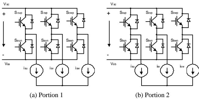
Fig. 4. Equivalent circuit in region 5
