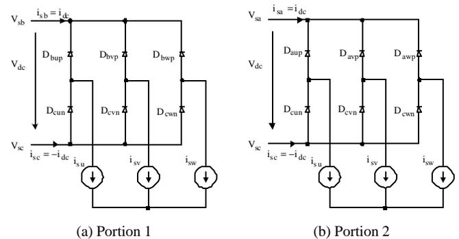
Fig. 5. Equivalent circuit in region 2 while the converter shut down
