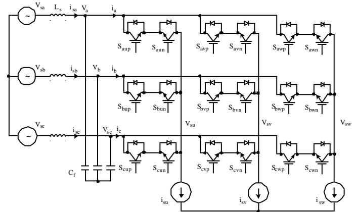
Fig. 1. Configuration of matrix converter system
