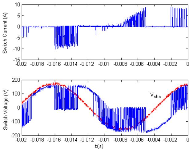
Fig. 11. Experimental result of switch voltage and switch current (  $i_{su}$  )
