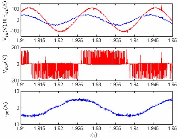
Fig. 10. Experimental result of the matrix converter
