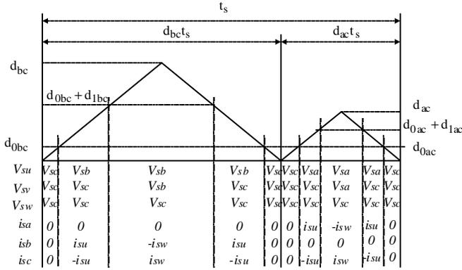
Fig. 8. PWM sequences in each switching cycle of interval 2
