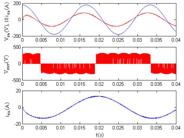
Fig. 9. Simulation result of the matrix converter
