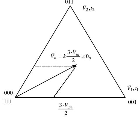
Fig. 7. Space vector PWM for inverter while  $0 < \theta_o < \pi/3$
