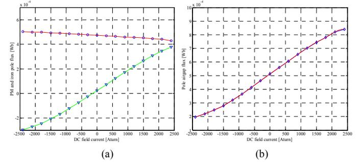
Fig. 6 Magnet and iron pole flux (a) and resultant airgap flux over one pole as a function of DC field current (No load)
