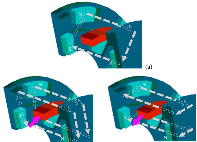
Fig. 3 Operating principle of the FCT machine showing the magnet created and field winding created flux components: (a) No DC field current, (b) negative DC field current and (c) positive DC field current
