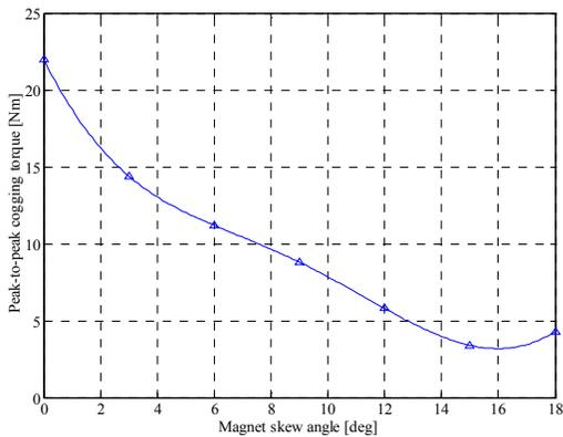
Fig. 12. Peak to peak cogging torque for the FCT machine for different skew angles
