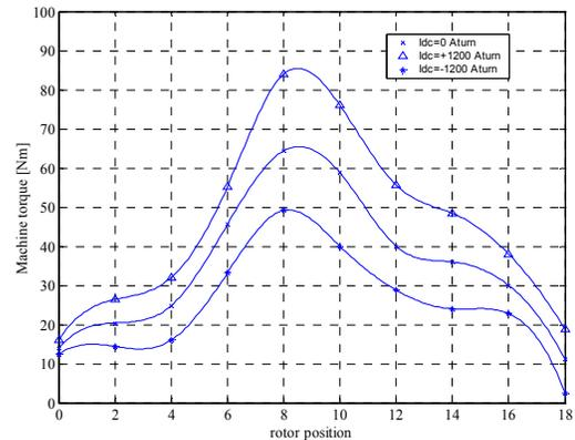
Fig. 10. Static torque characteristics of the FCT machine for different field current values at rated conditions
