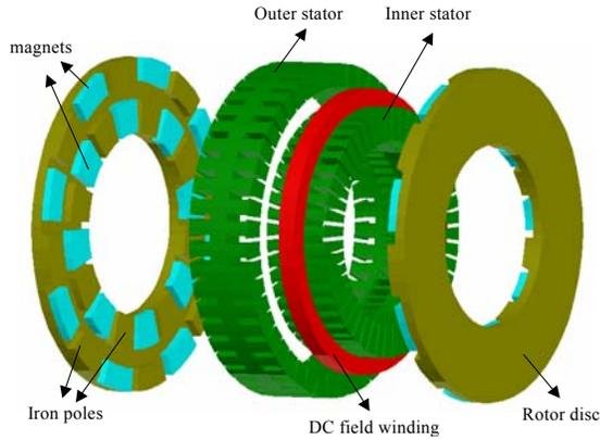
Fig. 1. 3D view of the new axial flux surface mounted field controlled PM machine without 3 phase AC winding
