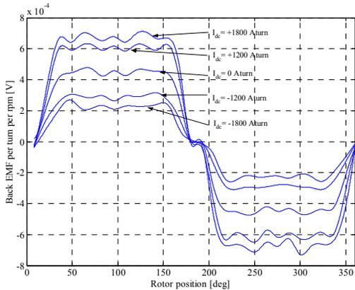
Fig. 8. Back EMF (per turn per rpm) variation of the FCT machine for different DC field currents
