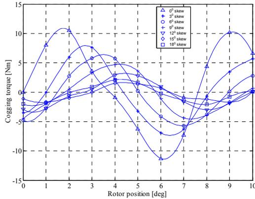
Fig. 11. Peak cogging torque variation for different magnet skew angles
