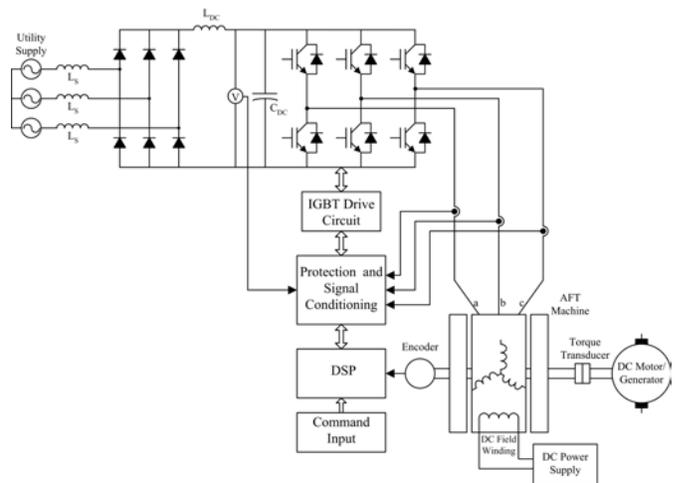
Fig. 13. Experimental system set-up of the field controlled axial flux PM machine
