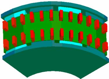
Fig. 5. 3D FEA model of the FCT machine
