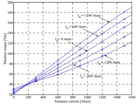
Fig. 9 Machine torque for various values of armature and field currents
