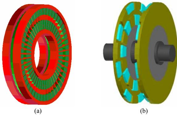
Fig. 2. 3D view of the stator (a) and rotor (b) structures of the FCT machine
