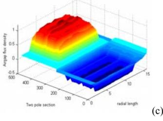
Fig. 4 Airgap flux density distribution for different values of the DC field current over two poles (a) 0 Atturns, (b) +1200 Atturns, (c) -1200 Atturns
