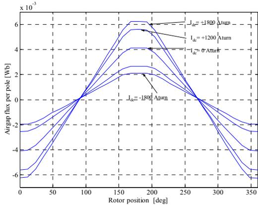
Fig. 7. Airgap flux (per turn per rpm) variation of the FCT machine for different DC field currents
