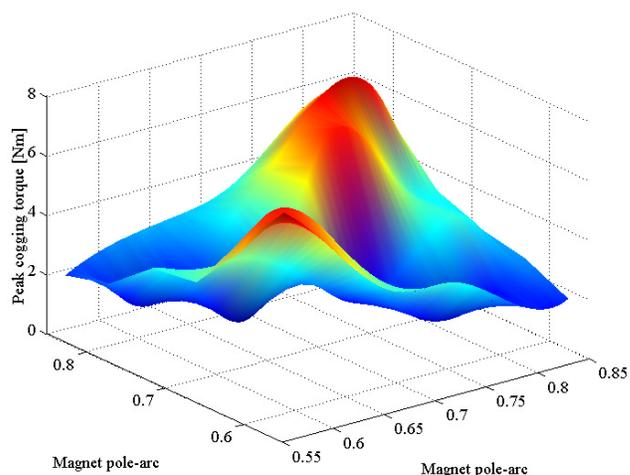
Figure 11. Peak cogging torque variation of the double-rotor-single-stator AFPM motor using finite element analysis as both adjacent magnet pole-arcs ( $\alpha_m$  and  $\alpha_c$ ) are varied
