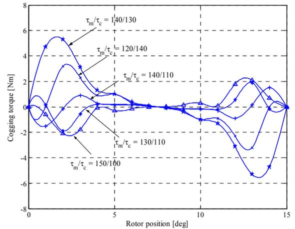
Figure 8. Cogging torque plots for different combinations of magnet pitch (in Nm)
