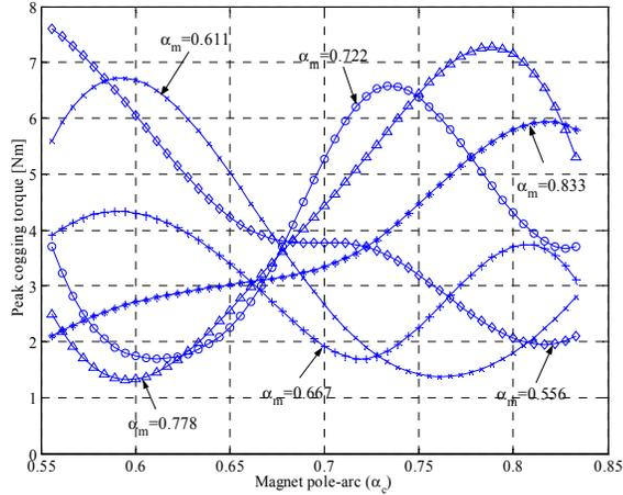
Figure 12. Peak cogging torque for various magnet pole-arcs around the focused critical magnet pole-arc region
