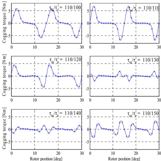
Figure 9. Cogging torque versus rotor position for different magnet pole arcs for a fixed  $\tau_m$  and varying  $\tau_c$  (in Nm s). First magnet pitch ( $\tau_m$ ) is fixed at 110 electrical degrees and the second magnet pitch ( $\tau_c$ ) is varied
