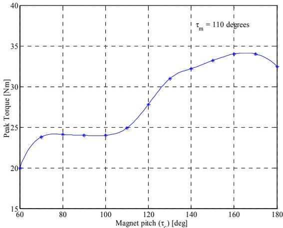
Figure 13. Peak torque versus magnet pole-arc for the AFPM machine for a fixed  $\tau_m (=110$  degrees) and varying  $\tau_m$
