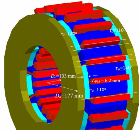
Figure 5. One of the 8-pole 24-slot double-rotor-single-stator AFPM motor models used in the cogging torque analyses (Case:  $\tau_m=110^\circ$  and  $\tau_c=140^\circ$ )
