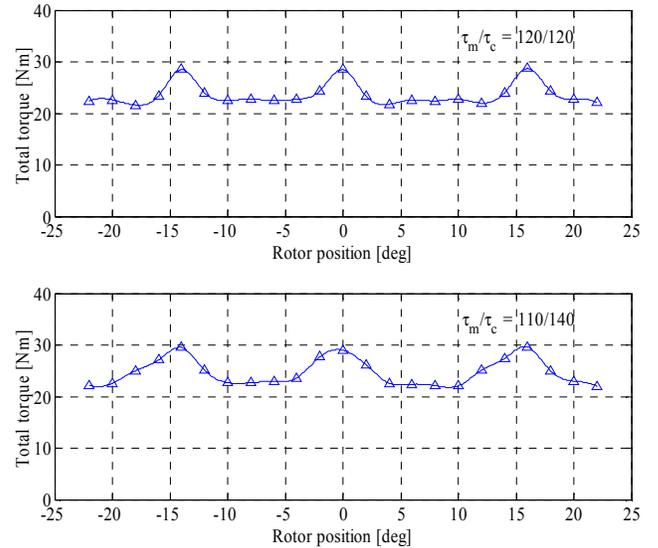
Figure 14. Total torque variation for two cases of magnet pole-arcs: (Case1:  $\tau_m/\tau_c = 120/120$  and Case2:  $\tau_m/\tau_c = 110/140$ )
