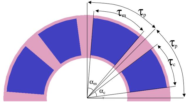
Figure 2. One of the AFPM machine rotors with alternating magnet pole-arcs. The other rotor disc is rotated by one mechanical pole.
