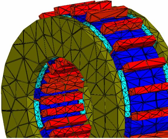
Figure 6. Typical 3D finite element mesh for one of the AFPM motor models analyzed (Case:  $\tau_m=110^\circ$  and  $\tau_c=140^\circ$ )
