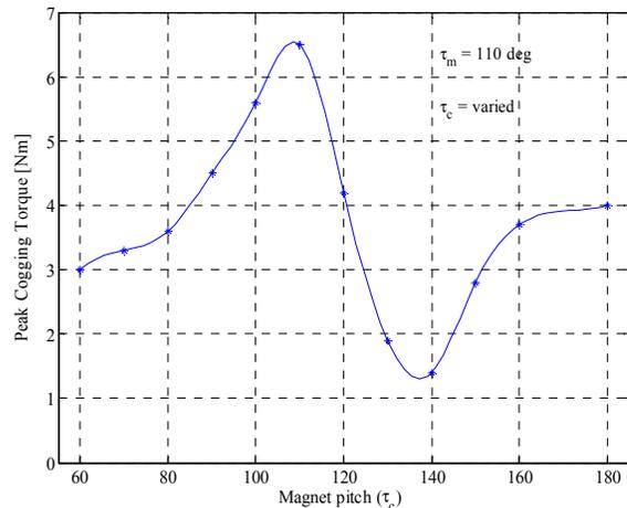
Figure 10. Peak cogging torque variation for various magnet pitch values with one of the magnet pitch is fixed at  $\tau_m = 110$  electrical degrees
