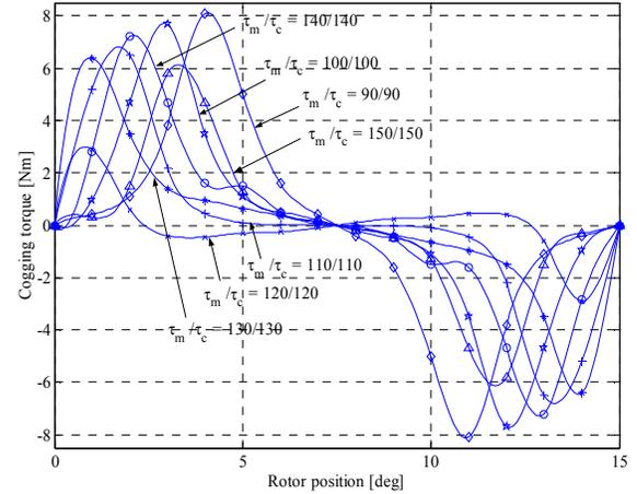
Figure 7. One cycle of cogging torque versus magnet rotor position for different values of magnet pole-arc (one cycle)
