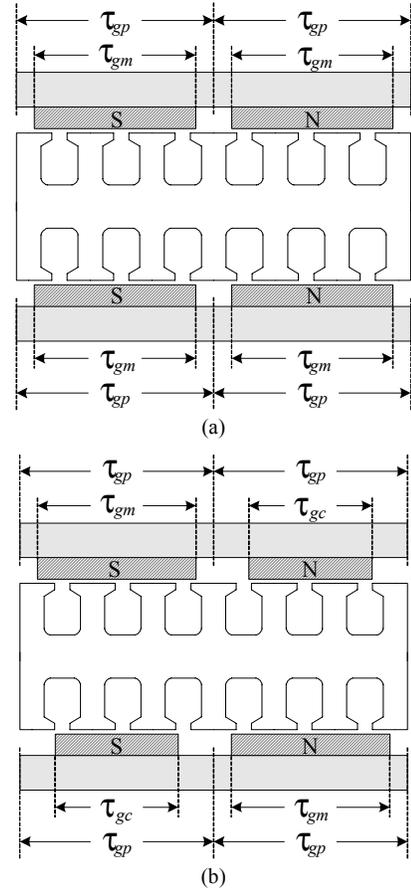
Figure 1. Two pole section of the (a) conventional double-rotor-single-stator AFPM machine with the same magnet pole-arc and (b) AFPM machine with alternating pole arcs for cogging torque minimization at the average diameter
