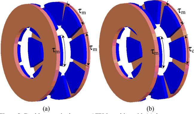
Figure 3. Double rotor single stator AFPM machine with (a) the same magnet pole-arcs and (b) alternating magnet pole-arcs for the purpose of cogging torque minimization
