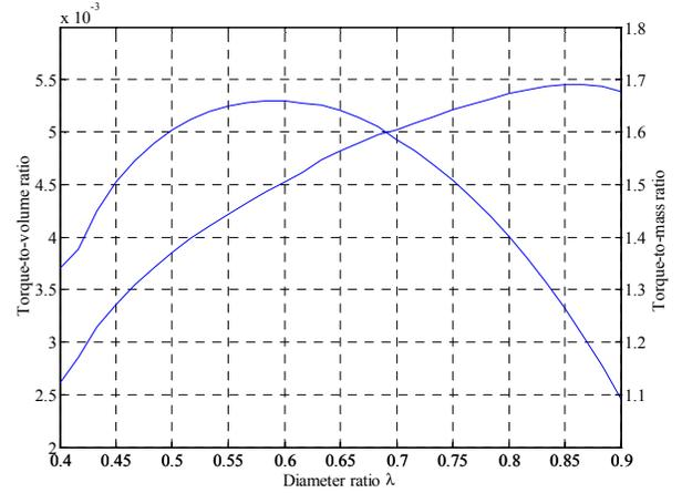
Figure 4. Torque density including torque-per-volume (Nm/cm<sup>3</sup>) and torque-per-kilogram (Nm/kg) plots as a function of diameter ratio for 3kW, 8 pole, double-rotor-single-stator North-North (NN) type AFPM machine
