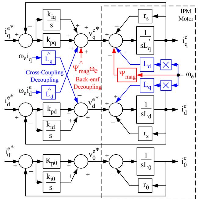
Fig. 7. Block diagram of the cross-coupling decoupling synchronous frame current regulator for IPM motor drives.
