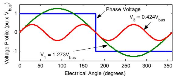
(b) Six-leg inverter voltage components in square wave operation.
