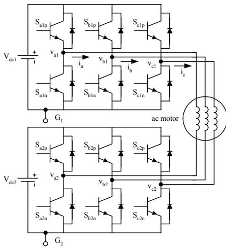
Fig. 2. Cascaded converter with separate dc links.
