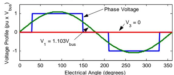
(c) Maximum six-leg inverter voltage components without a third harmonic.
