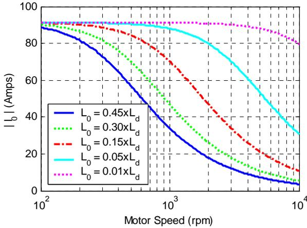
Fig. 8. Induced zero sequence current with magnet flux nulling control.
