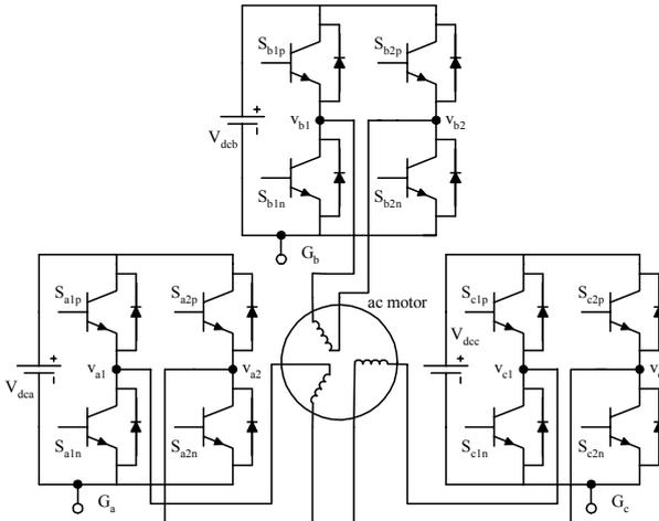
Fig. 1. Three single-phase inverters driving a three-phase ac motor.
