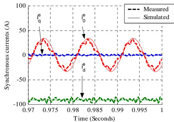
(b) Synchronous frame  $dq0$  currents.
