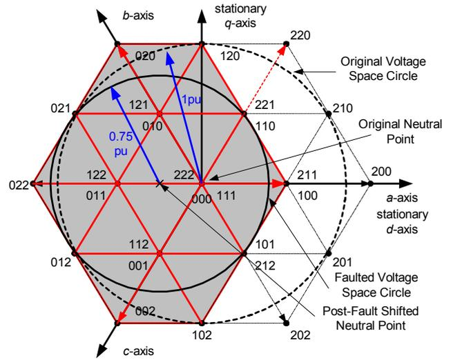
Fig. 6. Voltage space limits for pre- and post-fault single-switch short-circuit conditions for the six-leg inverter.
