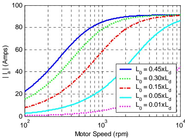
Fig. 9. Induced current in the shorted phase when employing magnet flux nulling control following a shorted stator winding.
