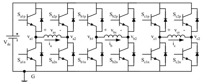
Fig. 4. Six-leg converter with a single dc bus.
