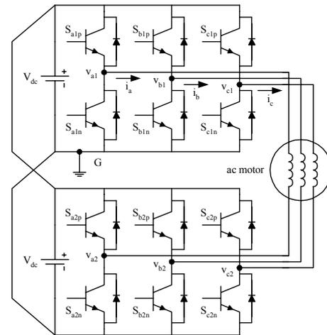
Fig. 3. Cascaded converter with connected dc links.
