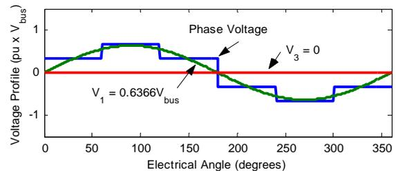
(a) Standard three-leg inverter voltage components in six-step operation.
