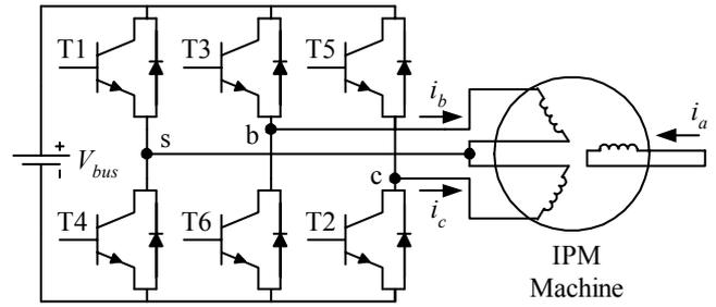
Fig. 10. Experimental drive configuration.
