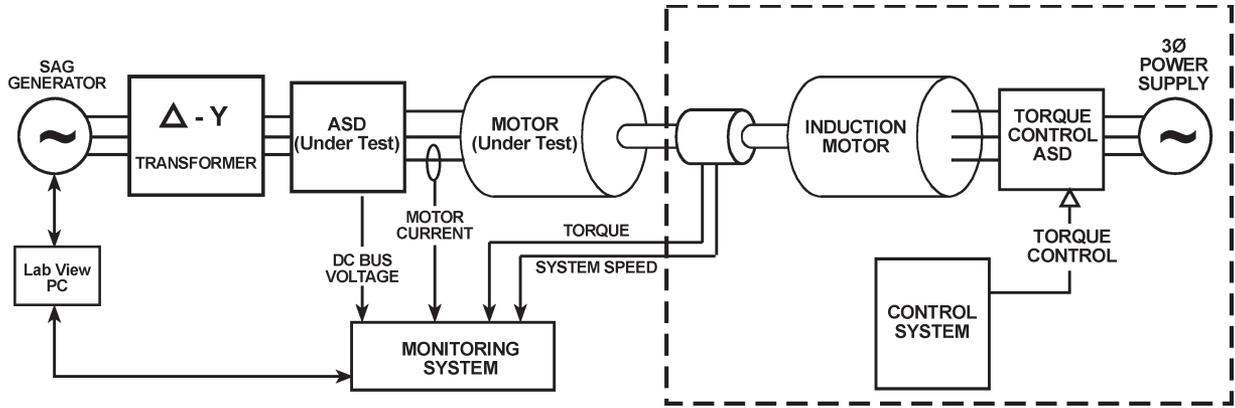
Fig. 10. Experimental test-equipment configuration.
