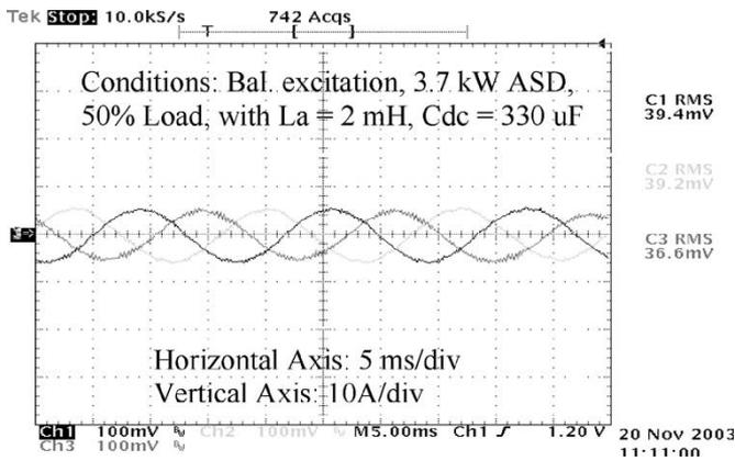
Fig. 11. Measured stator-current waveforms during balanced excitation at 460-V input voltage (50% load).
