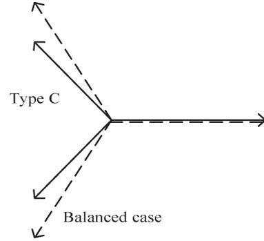
Fig. 2. Phasor diagram of type-C three-phase unbalanced input-voltage sag.
