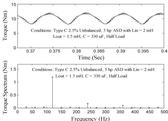
Fig. 9. Simulation results of machine-torque frequency spectrum during type-C sag with 2.5% voltage unbalance (50% load).
