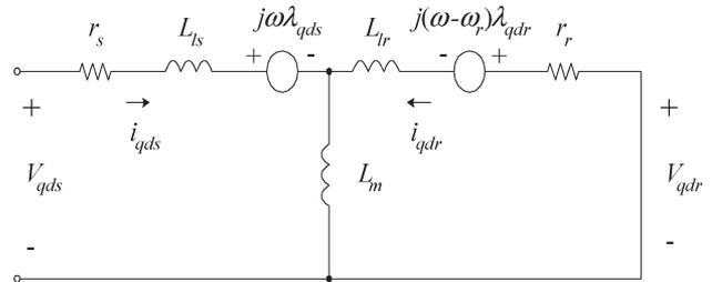
Fig. 13. Complex  $dq$  equivalent circuit of a three-phase induction machine in a rotating reference frame ( $\omega$ ).
