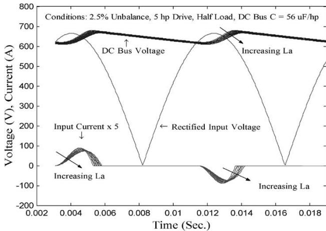
Fig. 4. Rectified input line voltage during single-phase operation caused by a type-C sag with 2.5% unbalance, showing dc-bus input current  $i_{dc}$  and dc-bus voltage  $v_d$  with varying line inductance (1%–2%).
