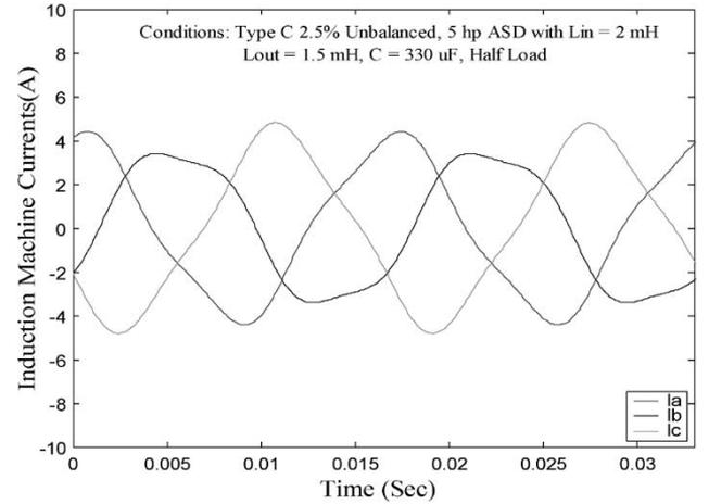
Fig. 6. Closed-form analysis results of machine phase currents during type-C sag with 2.5% voltage unbalance (50% load).
