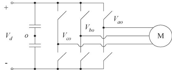
Fig. 5. Three-phase VSI diagram.
