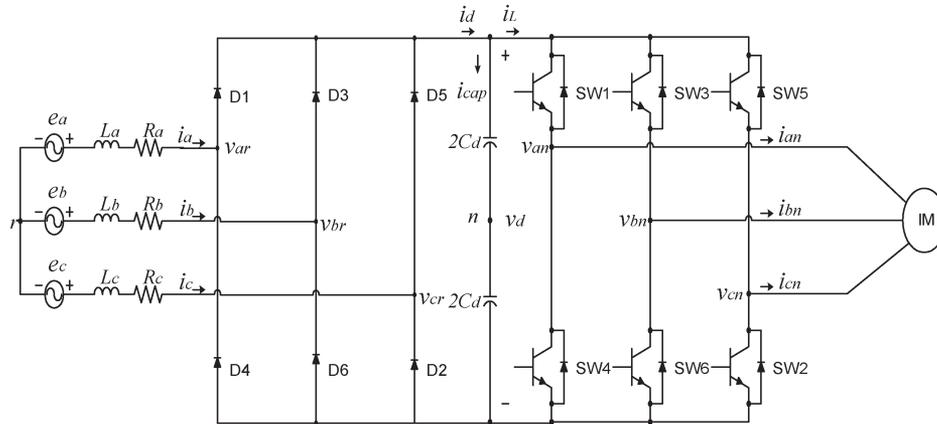
Fig. 3. Induction-machine ASD power circuit diagram including a three-phase input rectifier stage, a dc link, and a three-phase output inverter stage.
