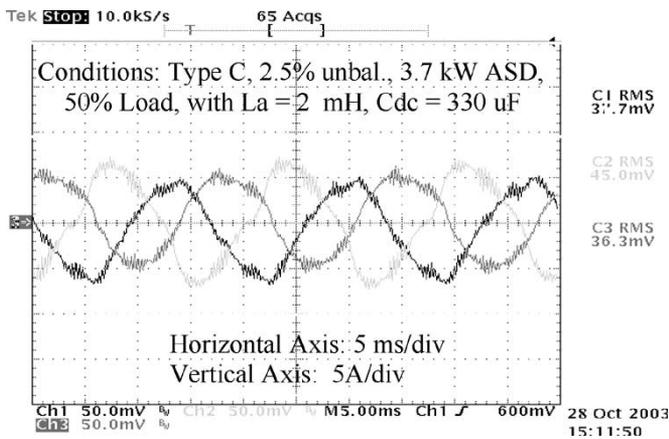
Fig. 12. Measured stator-current waveforms during type-C sag with 2.5% voltage unbalance (50% load).
