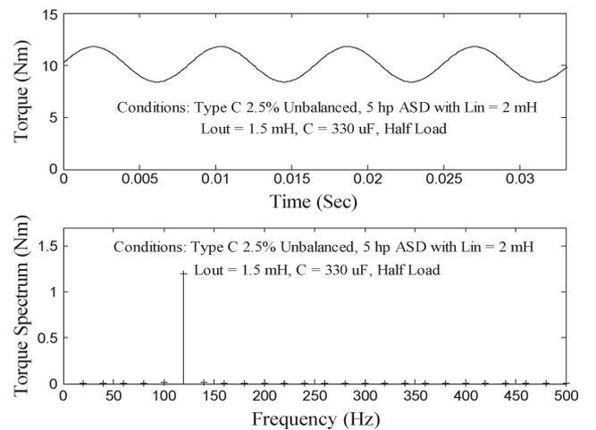
Fig. 7. Closed-form analysis results of machine-torque frequency spectrum during type-C sag with 2.5% voltage unbalance (50% load).
