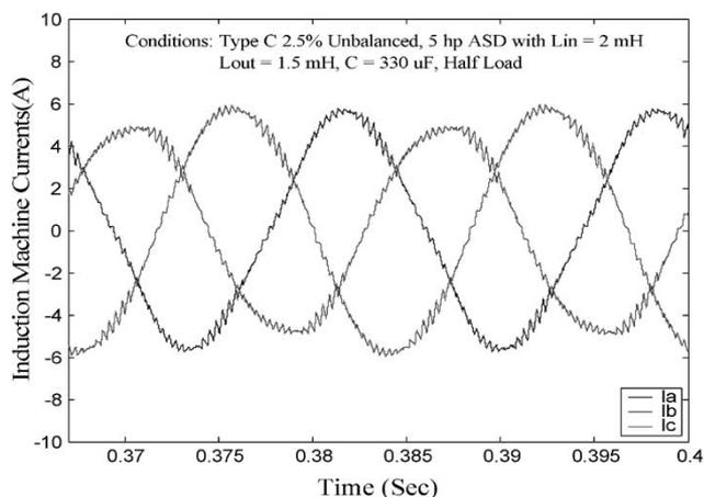
Fig. 8. Simulation results of machine phase currents during type-C sag with 2.5% voltage unbalance (50% load).
