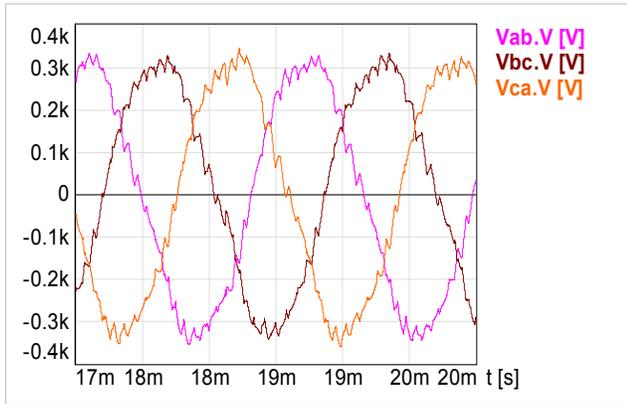
Fig. 10. Line to line voltage of the RL load
