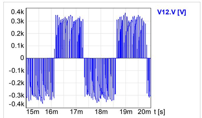
Fig. 4. Line voltage waveform of the generator
