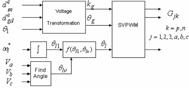
Fig. 3. Space vector PWM of DBMC under boost mode
