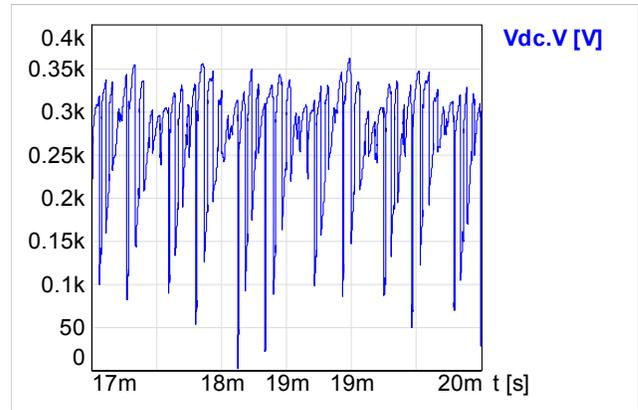
Fig. 7. DC bus voltage of the DBMC
