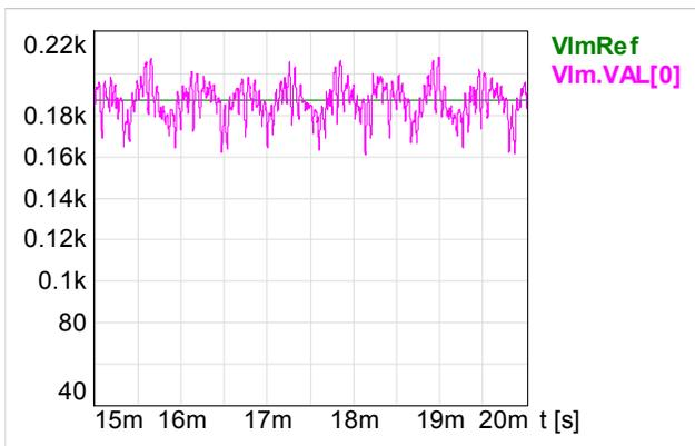
Fig. 6. RL load voltage command and the simulated voltage amplitude
