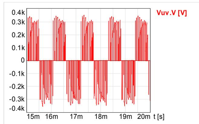
Fig. 8. Induction motor side line to line voltage
