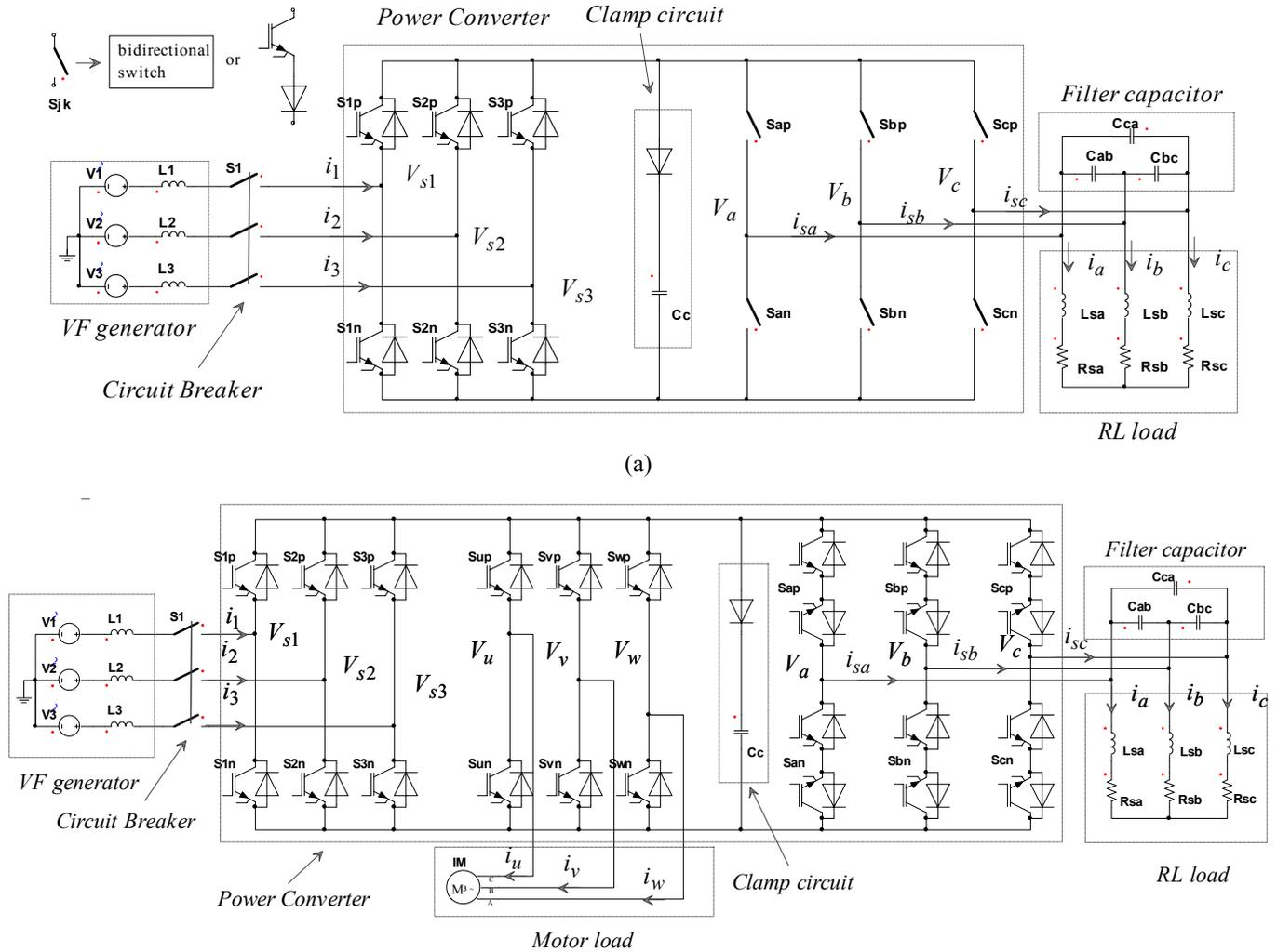
Fig. 1. Circuit configuration of DBMC operating under boost mode
