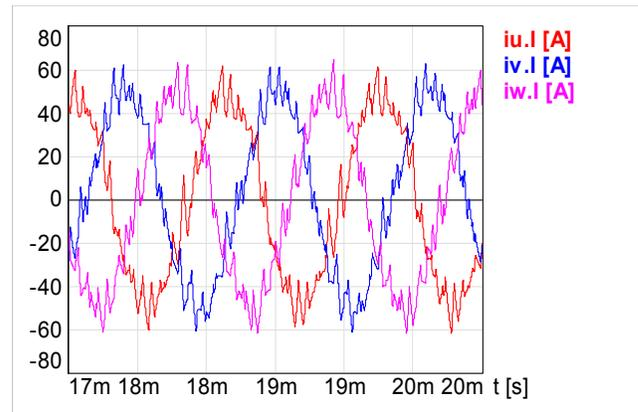
Fig. 9. Phase current of the induction motor
