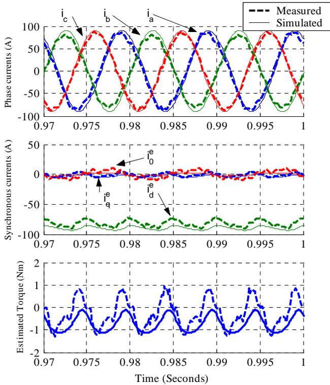
Fig. 7. Experimental and simulated results without a zero sequence at  $\omega_r = 1000$  rpm.
