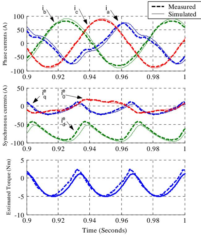
Fig. 6. Experimental and simulated results without a zero sequence at  $\omega_r = 150$  rpm.
