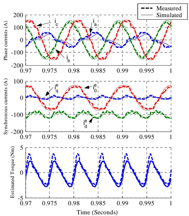
Fig. 9. Experimental and simulated results with a zero sequence at  $\omega_r = 1000$  rpm.
