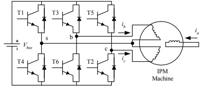
Fig. 5. Experimental drive configuration.
