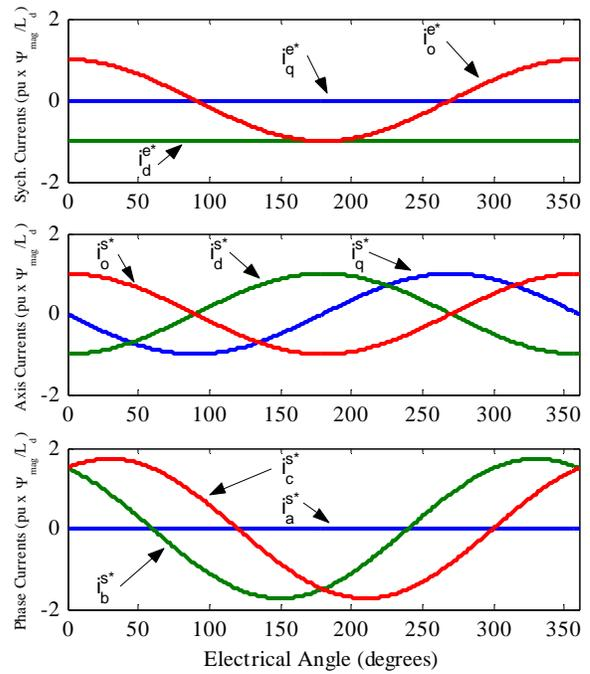
Fig. 3. Idealized flux nulling current commands with a zero sequence current command.
