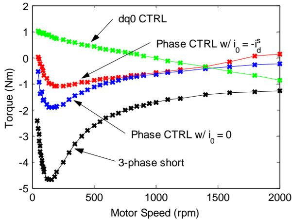
Fig. 11. Measured steady-state motor torque for different post-fault control methods.
