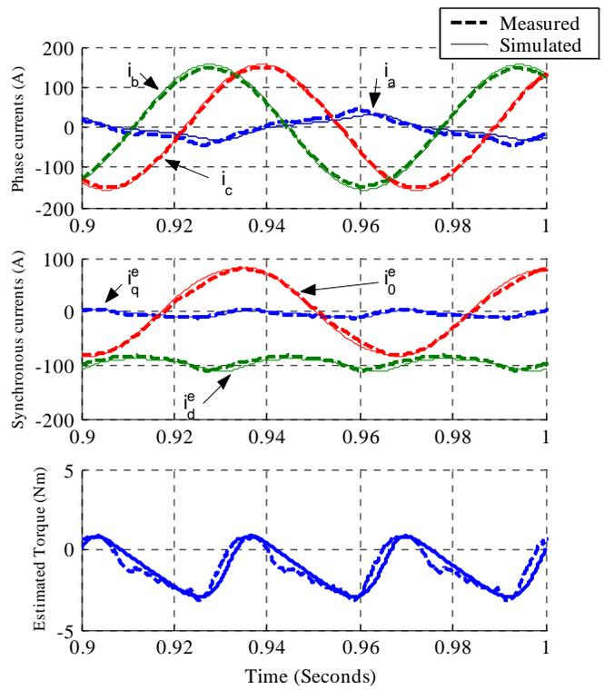
Fig. 8. Experimental and simulated results with a zero sequence at  $\omega_r = 150$  rpm.
