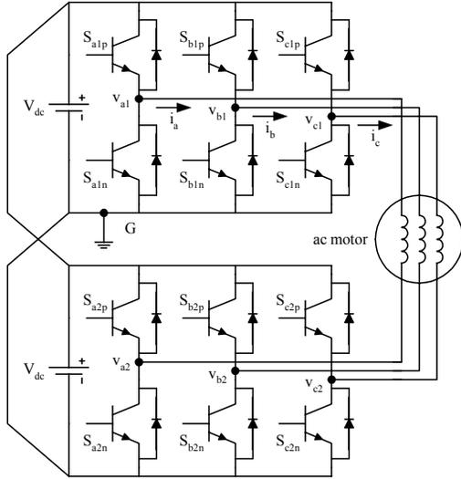
Fig. 1. Cascaded converter with connected dc links.
