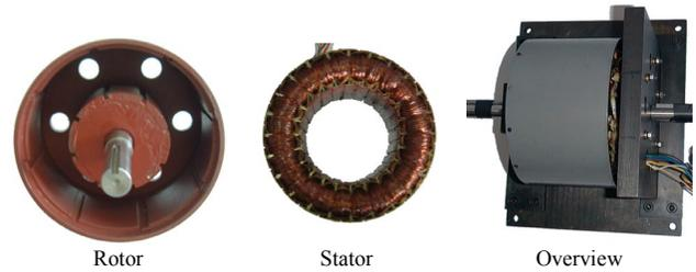
Figure 3. RFTPM prototype machine
