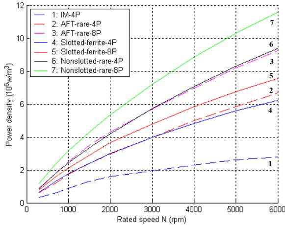
Figure 4. Power density comparison among RFTPM, AFTPM and induction machines
