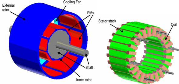
Figure 1. Dual-rotor, toroidally wound, slotted, RFTPM machine
