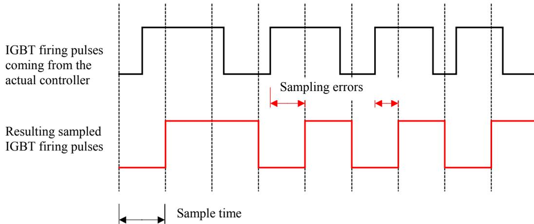
Fig. 2. Sampling errors made with standard I/O
