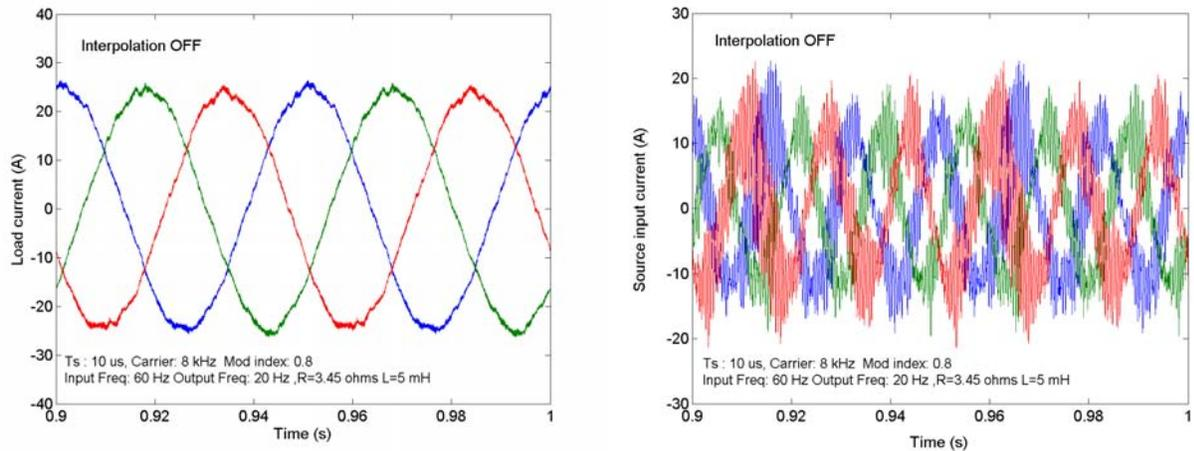
Fig. 11. Load and input filter current simulation at 10  $\mu$ s time step with interpolation disabled
