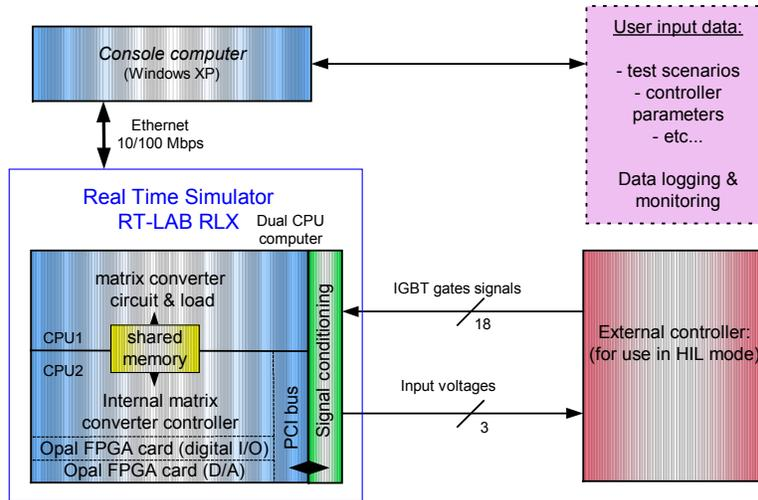
Fig. 3. Structure of the RT-LAB real-time simulator
