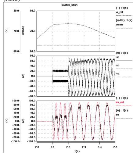
Fig. 10 Simulation results during starting of a 30kW doubly-fed wound rotor induction machine: (i) with contactor start method (LHS) and (ii) with extra switching start method (RHS)
