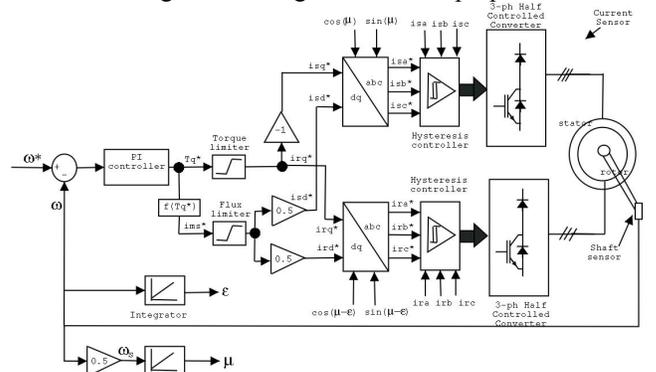
Fig. 6 Block diagram of the machine side control algorithm
