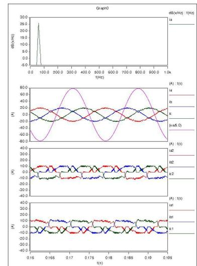
Fig. 11 Typical simulation results of a 30kW line side converter : (i) with full load and without active filter algorithm, (LEFT ), (ii) with full load and with active filter algorithm (CENTER) and (ii) with 30% load and with active filter algorithm (RIGHT)
