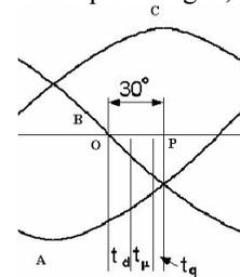
Fig. 5 Commutation methodology for the line commutated thyristors
