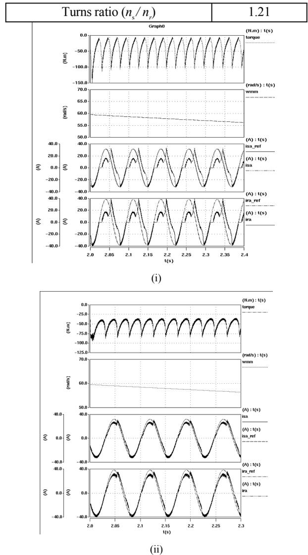
Fig. 8 Simulation results at (i) 25% load with full field excitation and (ii) at 25% load with field excitation as a function of load
