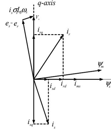
Fig. 3 Steady-state phasor diagram (stator reference frame) of a doubly-fed wound rotor induction machine for the super-synchronous generating mode
