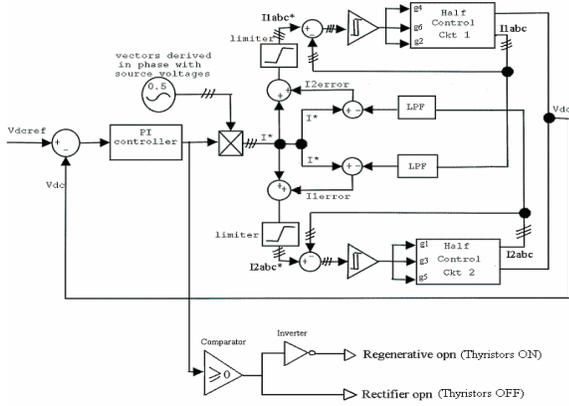
Fig. 7 Block diagram of the proposed line side control algorithm
