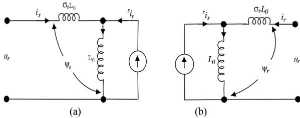
Fig. 2 Equivalent circuit diagrams of a doubly-fed wound rotor induction machine: (a) for rotor side control (LHS) and (b) for stator side control (RHS)
