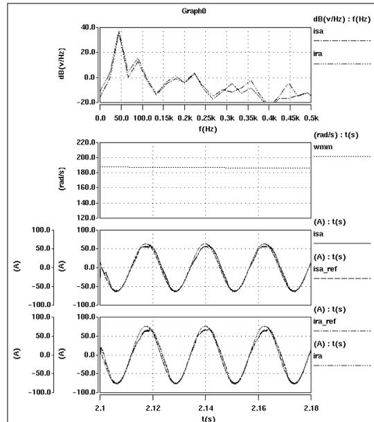
Fig. 9 Typical simulation results of a 30kW doubly-fed wound rotor induction machine: (i) with rotor shaft frequency at 30Hz (LHS) and (ii) with rotor shaft frequency at 90Hz (RHS)
