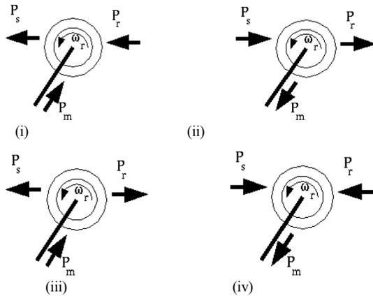
Fig. 1 Power flow diagram of a doubly-fed wound rotor induction machine for: (i) sub-synchronous generating mode, (ii) sub-synchronous motoring mode, (iii) super-synchronous generating mode and (iv) super-synchronous motoring mode
