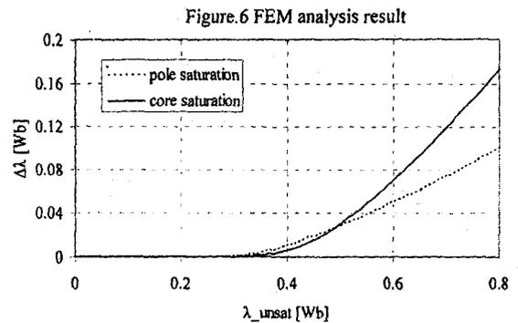
Figure 8 Core and Pole saturation curves.
