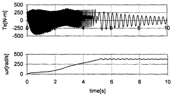
Figure 9 Torque and Speed during acceleration from rest.
