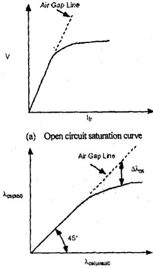
Figure 4 (a) Open circuit saturation curve and (b) derived curve.
