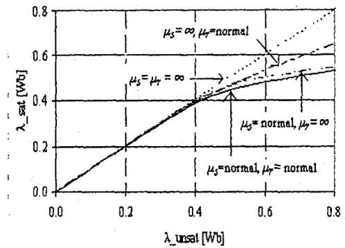
Figure 7 Saturation curves produced by finite elements.
