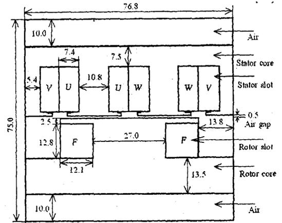
Figure 6 Dimensions of one pole of synchronous machine studied using finite elements.
