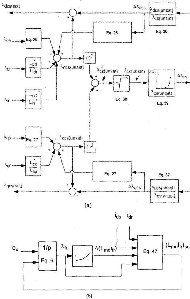
Figure 5 Flow diagram for simulation of (a) stator core saturation and (b) field pole saturation.
