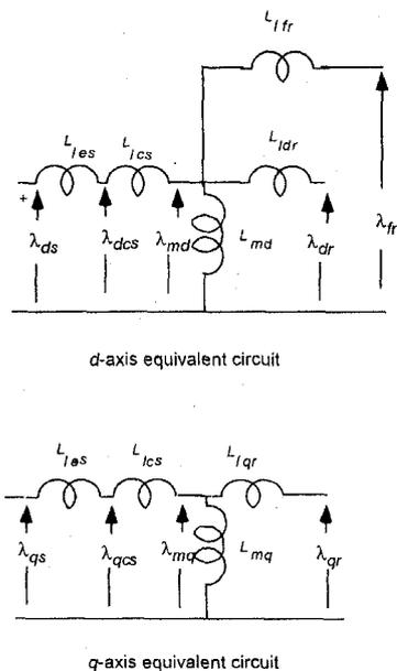
Figure 2 Flux linkages used as state variables.
