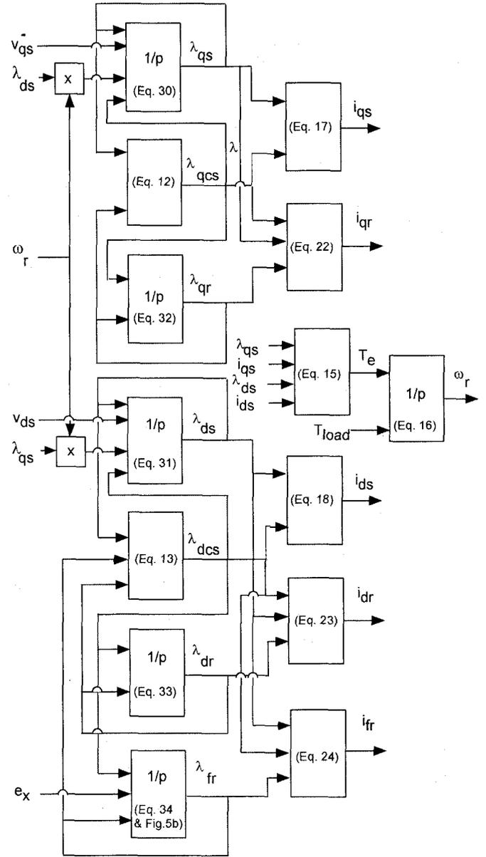
Figure 3 Signal flow diagram for a salient pole synchronous machine.
