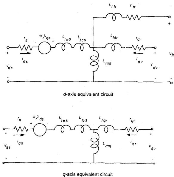
Figure 1  $d$ - $q$  axis equivalent circuit of a salient pole synchronous machine where the stator leakage inductance has been separated into saturable (core) and non-saturable (end winding) portions.
