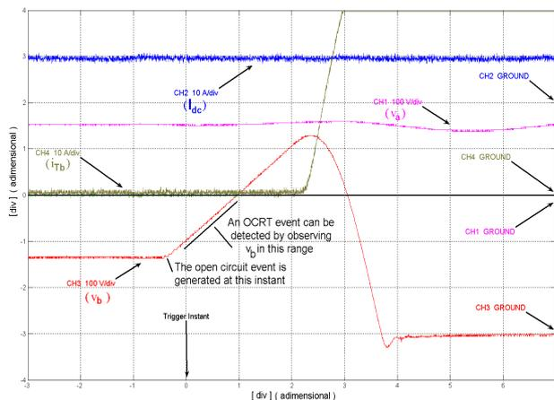
Fig. 10. Turn on of Thyristor  $T_b$  after a short circuit event at the left of port  $b1 - b2$
