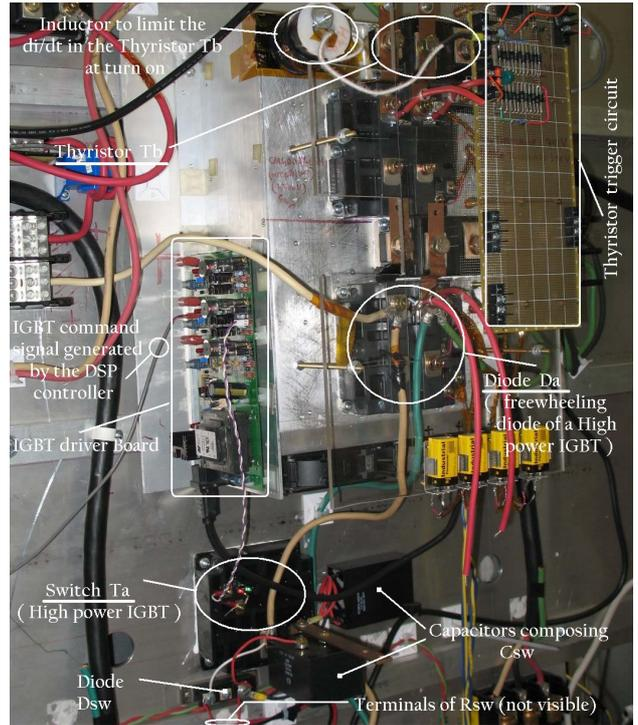
Fig. 9. Photo of the Switch  $T_a$  and fuses  $F_{a1}$  and  $F_{a2}$
