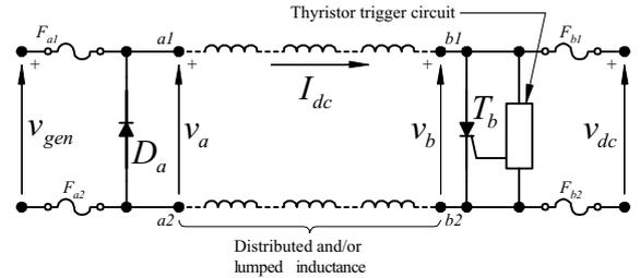
Fig. 4. Decentralized protection scheme.
