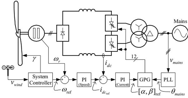
Fig. 3. Overview of the control system principle.
