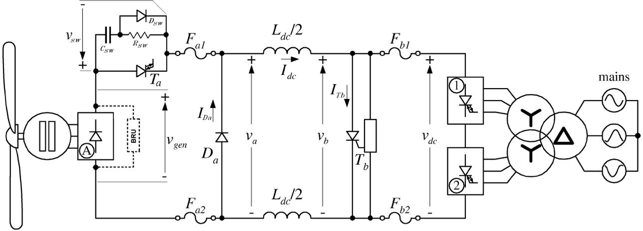
Fig. 5. Modified CSI topology to provide both fault protection and ride-through capability.
