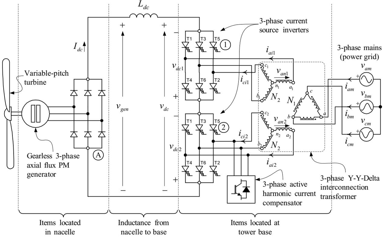
Fig. 2. Proposed Current source topology for gearless variable-speed wind turbines employing a permanent magnet synchronous generator.
