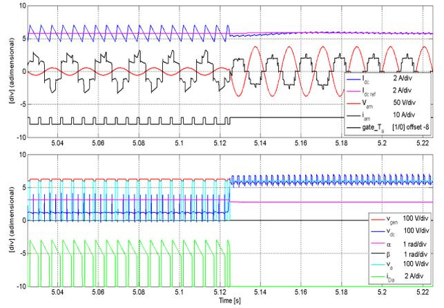
Fig. 7. Most significant quantities during the same LVRT event as Fig. 6 on an expanded time scale highlighting the recovery transient.
