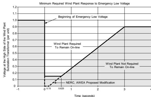
Fig. 1. Low Voltage Ride-Through (LVRT) requirement per Appendix G of FERC's Large Generator Interconnection Agreement (LGIA).
