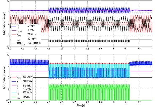
Fig. 6. Most significant quantities during a LVRT event lasting 0.625 seconds with percentage  $V_{LL}=0.15$  PU
