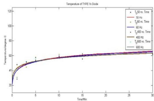
Fig 8. Temperature of TYPE I's diodes in degrees C.
