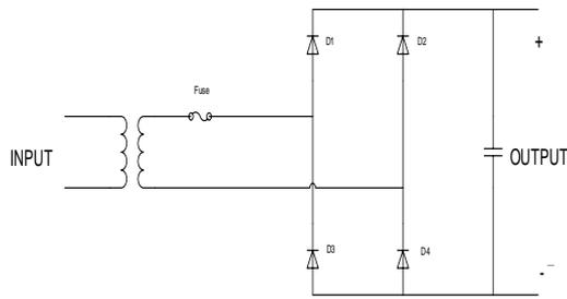
Fig 1. Topology of TYPE I DC power supply.
