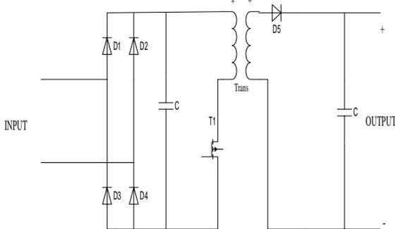
Fig 2. Simplified Topology of TYPE II DC power supply.
