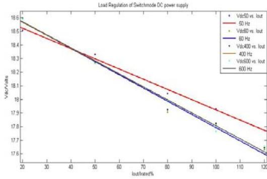
Fig 12. Load characteristics of TYPE II DC power supply.
