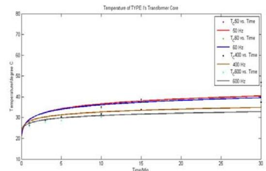
Fig 10. Temperature of TYPE I's Transformer Core.
