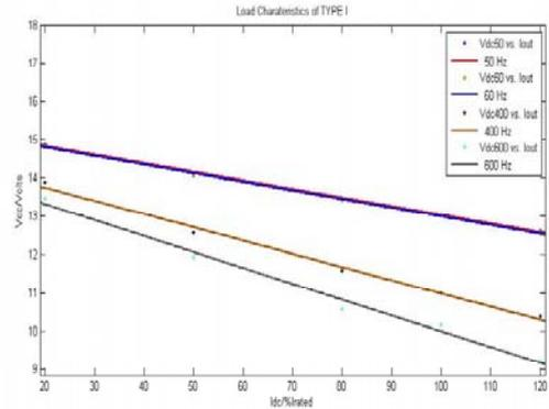
Fig 3. Load Characteristics of TYPE I DC power supply.
