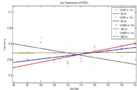
Fig 11. Line characteristics of TYPE II DC power supply.
